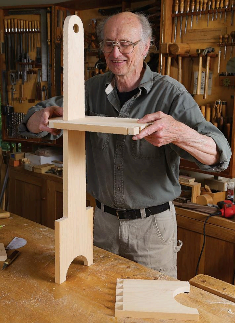
Mortise and dovetails first. Before applying glue, Becksvoort slides the back leg through the mortise in the step and just barely engages the dovetails at the front. He adds glue only to the dovetails and hammers them home.
