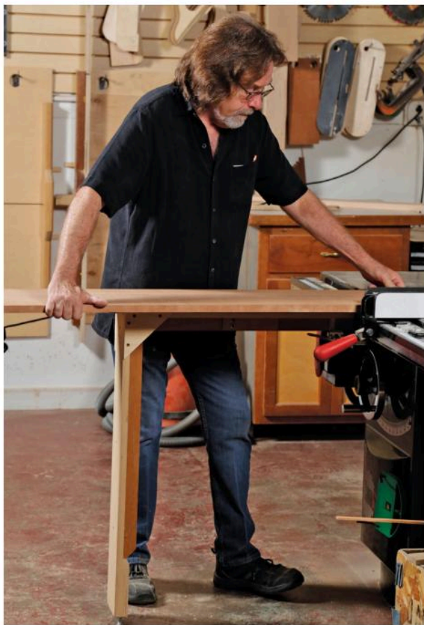
Stable setup. Feeding long stock into a tablesaw can be difficult without the proper support, so Van Dyke uses a specially made infeed support (left) that holds his stock at the right height, leaving him one less thing to worry about. If a board is so long you can't comfortably reach your right hand back to the end, grip the right edge of the board (center) and push until enough stock has gone through the blade that you can comfortably move your hand to the end of the board. Then the rip proceeds like any other (right).
