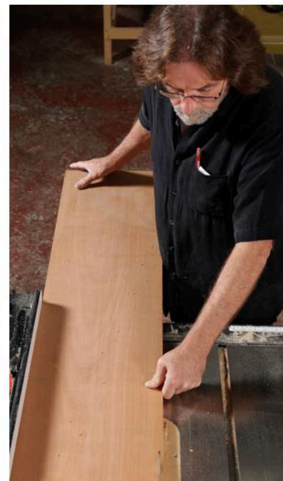
Stable setup. Feeding long stock into a tablesaw can be difficult without the proper support, so Van Dyke uses a specially made infeed support (left) that holds his stock at the right height, leaving him one less thing to worry about. If a board is so long you can't comfortably reach your right hand back to the end, grip the right edge of the board (center) and push until enough stock has gone through the blade that you can comfortably move your hand to the end of the board. Then the rip proceeds like any other (right).
