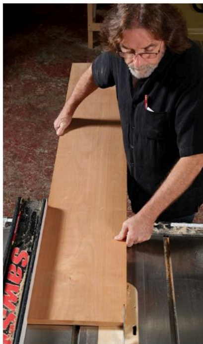
Stable setup. Feeding long stock into a tablesaw can be difficult without the proper support, so Van Dyke uses a specially made infeed support (left) that holds his stock at the right height, leaving him one less thing to worry about. If a board is so long you can't comfortably reach your right hand back to the end, grip the right edge of the board (center) and push until enough stock has gone through the blade that you can comfortably move your hand to the end of the board. Then the rip proceeds like any other (right).
