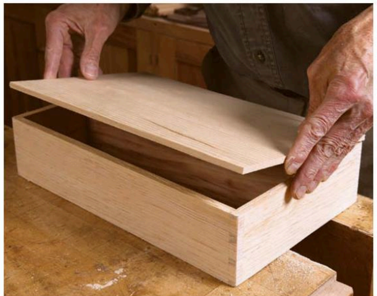
Insert the handle and add the bottom. After gluing up the dovetails, slide the handle in from the bottom, trapping it in place when you glue the bottom directly to the box (right).
