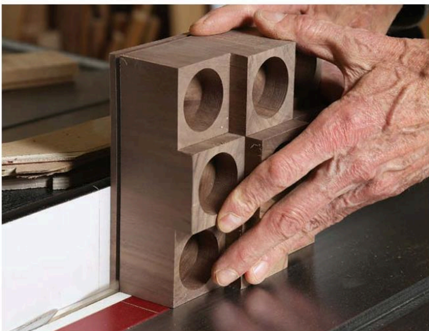
Adding a rabbet creates a base. Use the tablesaw to make two cuts on each side of the bottom. First, with the assembly bottom against the rip fence, make a cut on all four sides. Then with the bottom on the tablesaw top, cut along all four sides again.
