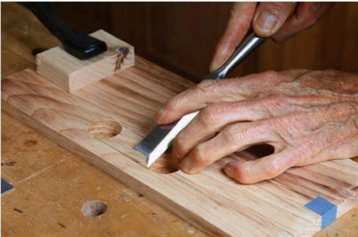
The handle is also the divider. After drilling both ends of the hand-hold with a Forstner bit, use a chisel to waste out the center. Becksvoort works halfway through one side, flips the piece over, and removes the rest. Then he uses a drawknife (right) to shape the scooped ends of the handle.
