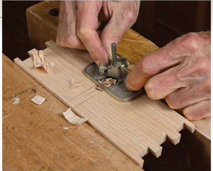
Cut a stopped dado. Because the stopped dados are small, Becksvoort cuts them by hand. He scribes the line with a knife, chisels out the sides and waste, and cleans it up with a router plane (right).
