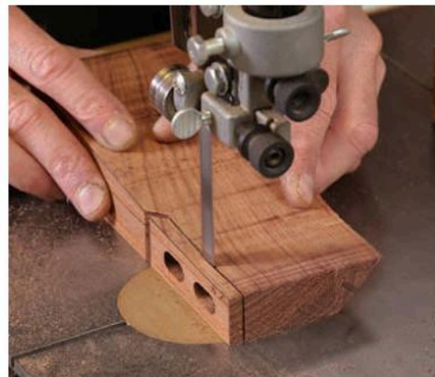
Finish the gunstock. Korsak roughs out the shoulder on the bandsaw. He'll follow up with multiple crosscuts on the tablesaw.
