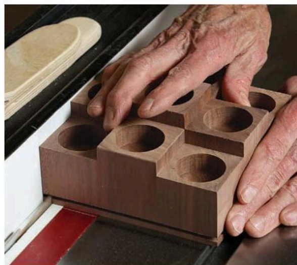
Adding a rabbet creates a base. Use the tablesaw to make two cuts on each side of the bottom. First, with the assembly bottom against the rip fence, make a cut on all four sides. Then with the bottom on the tablesaw top, cut along all four sides again.
