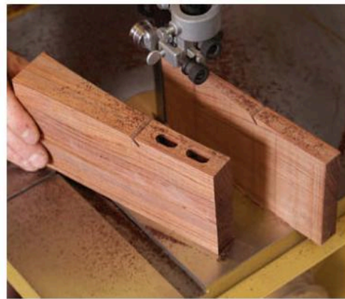
Bandsaw the sweep. The face of the foot is bandsawn to a curve.
