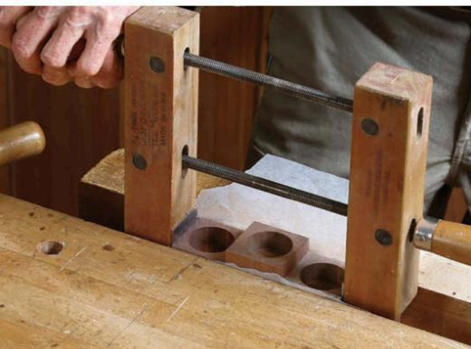
Cut and drill. After milling sticks square, use the tablesaw to cut all the parts to length. Then take the parts to the drill press. A hold-down jig keeps the block in place while you use a Forstner bit to drill the recess for the tea light candle.
