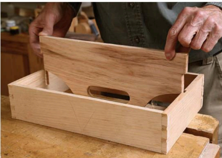
Insert the handle and add the bottom. After gluing up the dovetails, slide the handle in from the bottom, trapping it in place when you glue the bottom directly to the box (right).
