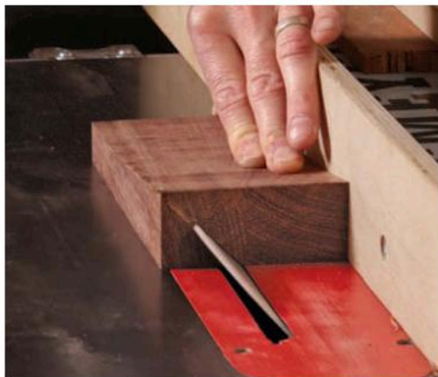
The feet meet in a miter. Korsak miter the feet at the tablesaw, cutting in several passes to reduce pressure on the short workpiece.
