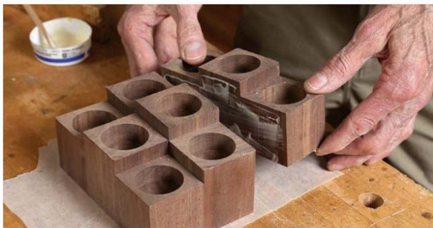
Glue up in two stages. First, glue together three rows of three. Once those are dry and cleaned up, glue the three rows into one block.
