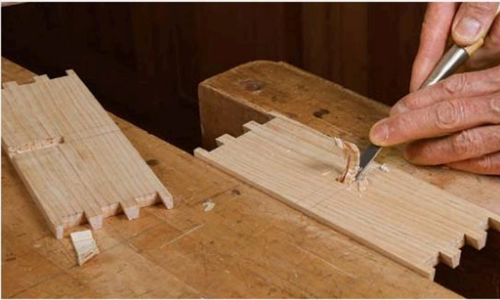
Cut a stopped dado. Because the stopped dados are small, Becksvoort cuts them by hand. He scribes the line with a knife, chisels out the sides and waste, and cleans it up with a router plane (right).
