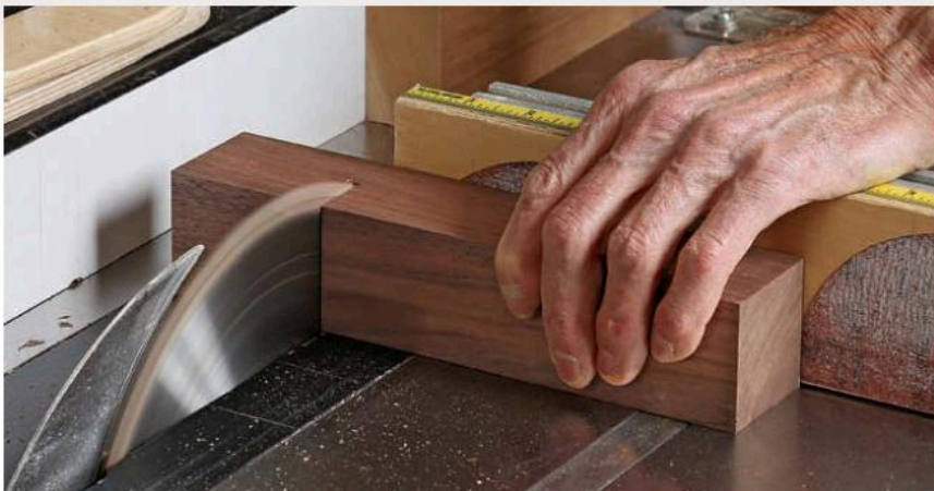
Cut and drill. After milling sticks square, use the tablesaw to cut all the parts to length. Then take the parts to the drill press. A hold-down jig keeps the block in place while you use a Forstner bit to drill the recess for the tea light candle.
