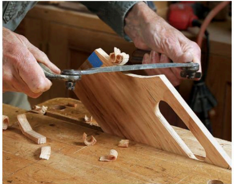
The handle is also the divider. After drilling both ends of the hand-hold with a Forstner bit, use a chisel to waste out the center. Becksvoort works halfway through one side, flips the piece over, and removes the rest. Then he uses a drawknife (right) to shape the scooped ends of the handle.
