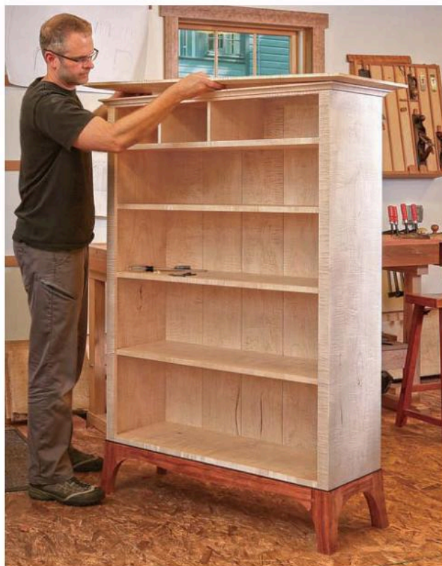
Tiny return. Because of the seasonal movement of the case sides, the side molding can't be joined to the back molding. For a clean seam, Korsak glues tiny mitered returns to the back end of the side molding.
