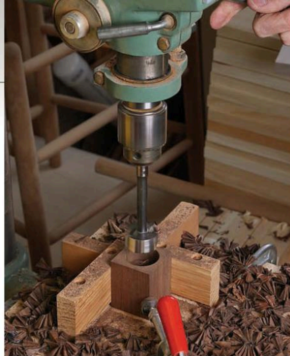
Cut and drill. After milling sticks square, use the tablesaw to cut all the parts to length. Then take the parts to the drill press. A hold-down jig keeps the block in place while you use a Forstner bit to drill the recess for the tea light candle.
