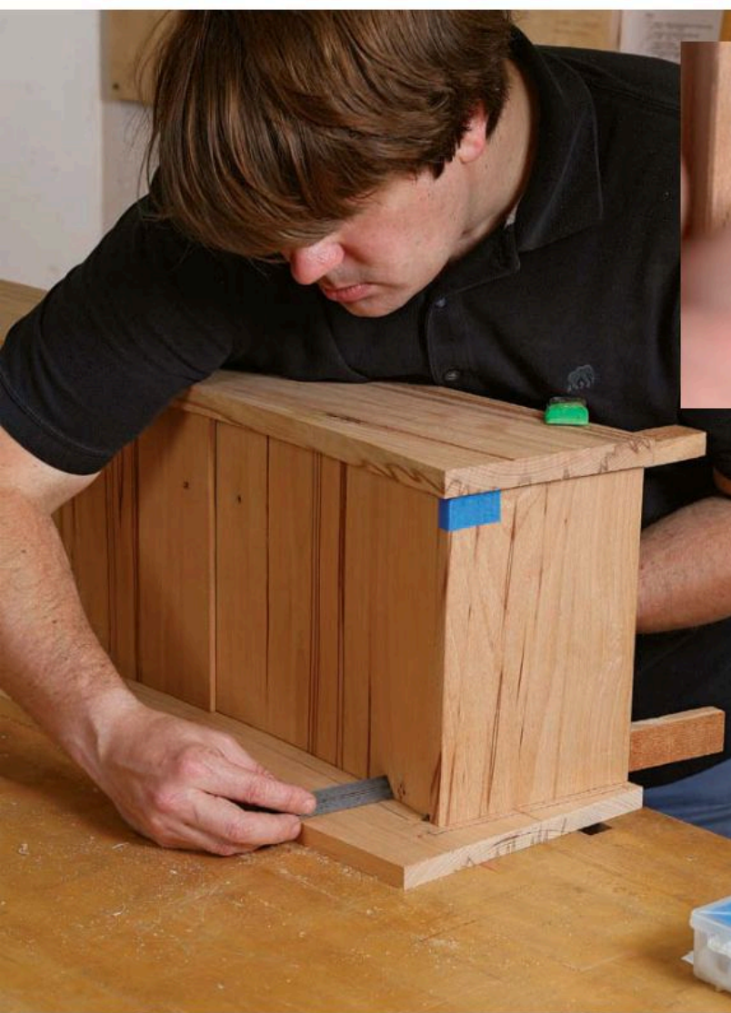
Locate the hinge. Blue tape on the cabinet creates a perfect gap, while a combination square ensures that all the hinges are in the same plane.
