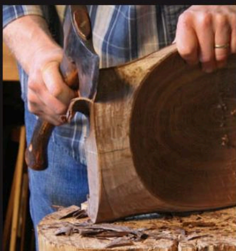
Shave the end grain. With the rest of the exterior nearly shaped, Fisher hews the handle, paring to the curved end line.
