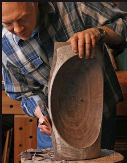
Ax work on the exterior. To rough-shape the outside of the bowl, Fisher alternates between hewing the sides and the back of the blank. Then he cuts right to the perimeter line.
