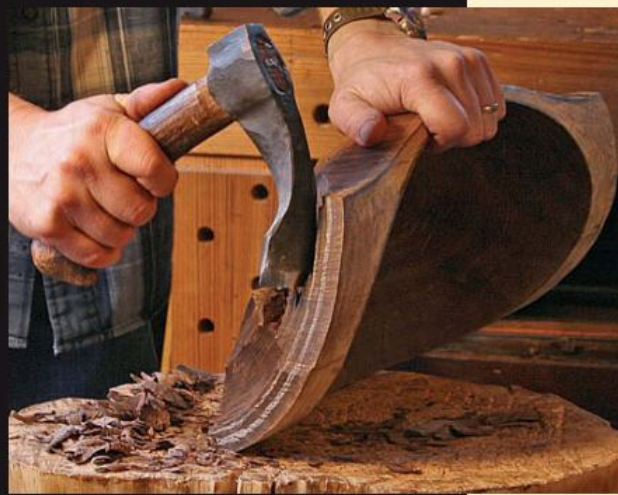
Hollow the handle. Switch to the adze and work cross-grain to create the concave underside of the handle.
