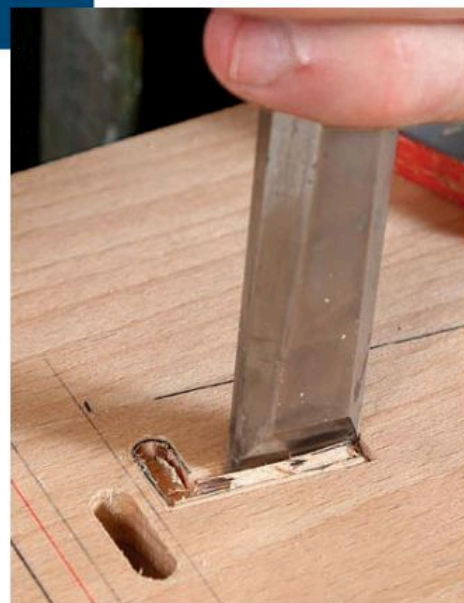
Pare to fit. After routing out the waste, use a chisel to clean up to the layout lines.
