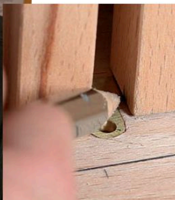
Mortise the door. Locate the door in the cabinet. Clamp scraps in the cabinet to keep it in place (left). Slide the door over and transfer the mortise (center). Hold the hinge in place and cut around it (right).
