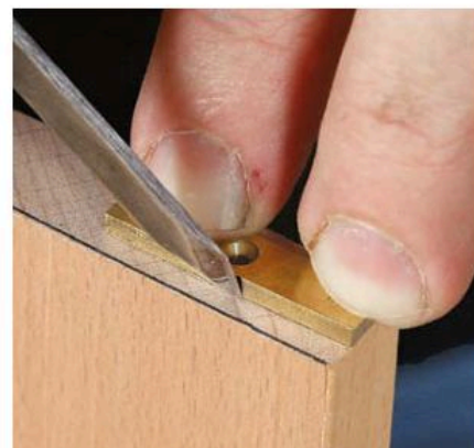
Mortise the door. Locate the door in the cabinet. Clamp scraps in the cabinet to keep it in place (left). Slide the door over and transfer the mortise (center). Hold the hinge in place and cut around it (right).
