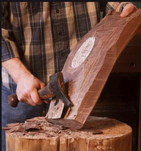
Ax work on the exterior. To rough-shape the outside of the bowl, Fisher alternates between hewing the sides and the back of the blank. Then he cuts right to the perimeter line.
