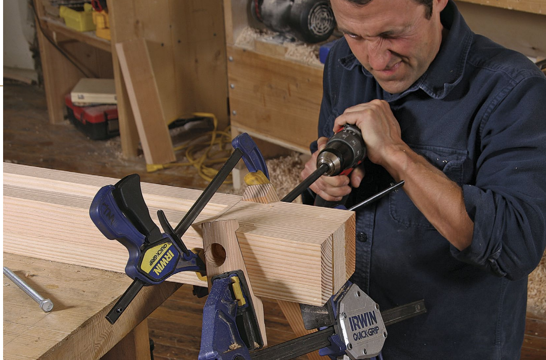
Boring for a bolt. After counterboring for the top bolt, Manney carefully drills the clearance hole.
