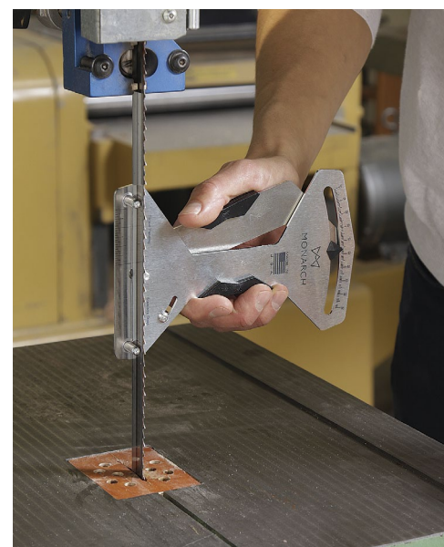
Clip to the blade, then read. The blade is pinched between the three pins, and its tension moves the indicator on the opposite end. An included chart provides tension ranges for various blade widths.
