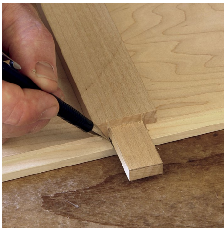
Tenon transfer, step one. With the tenons cut, replace the batten in the panel and mark the location of the tenons on the panel's tongue.
