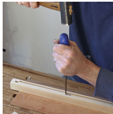
Chop away. Following your layout lines, chop mortises for the batten tenons.
