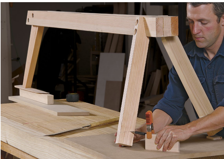
Shim and trim. After shimming the legs until the beam is parallel with the bench, scribe a line around each leg. Then cut them to length.
