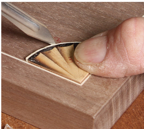
Tack it in place. Van Dyke uses a dab of hide glue to temporarily secure the fan in place while he scores the outline.
