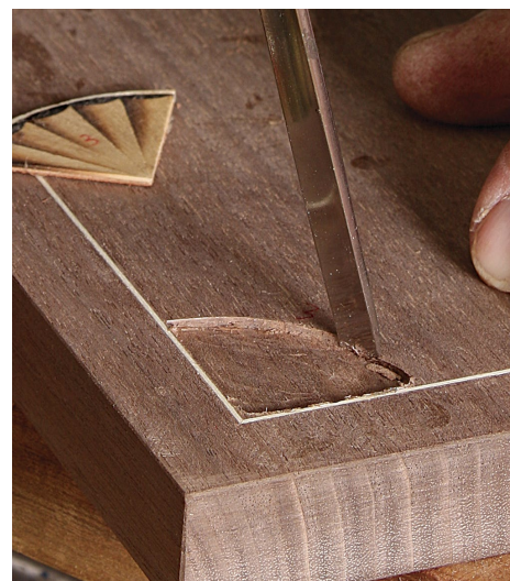
Rout close and clean up by hand. Rout freehand and as close to the line as you're comfortable (left). Then use a gouge (above) to cut to the line.
