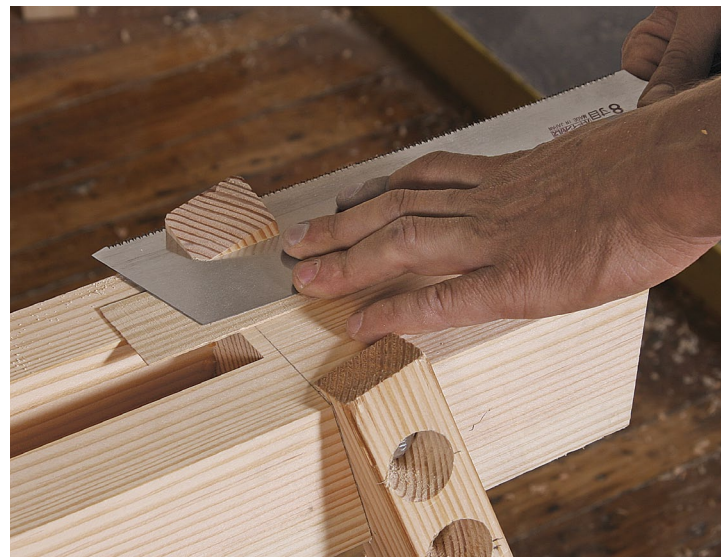
Flatten the tops. A thin shim protects the beam as Manney saws the rear legs nearly flush.
