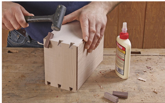
Tap in the key. The key slides in from one side only, but the taper guarantees that it fits tightly into the notch with no gap.
