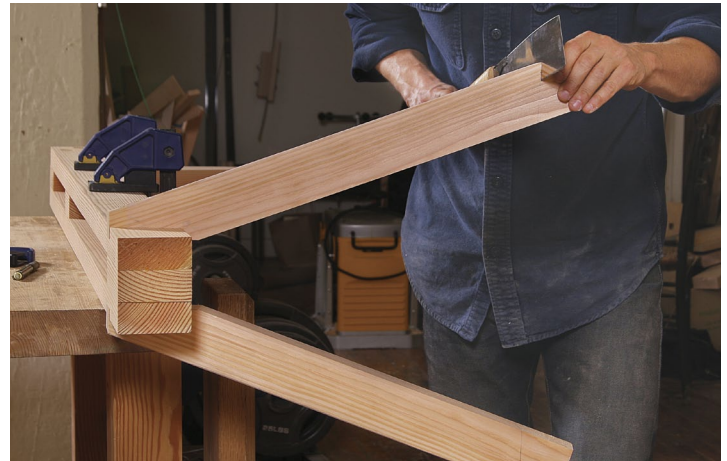
Shim and trim. After shimming the legs until the beam is parallel with the bench, scribe a line around each leg. Then cut them to length.
