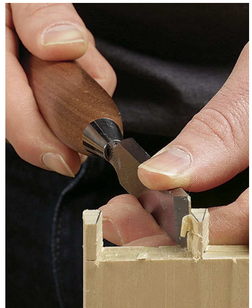
Refined. A long handle attached to the blade improves control, converting the tool into a paring chisel.
