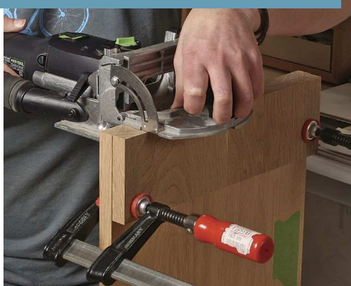
REMOVE SHIM AND MORTISE THE SIDE
