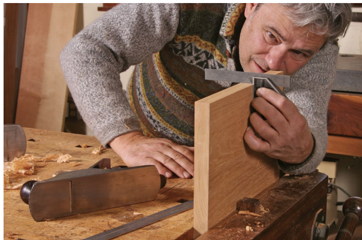
The vital reference. With the faces flat and parallel, square up one long-grain edge. This is the reference edge, used to lay out the other edges.
