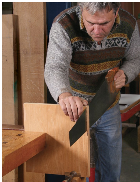
Find the line. Cullen counsels sawing close to the line to develop confidence and to save time in planing. He uses a crosscut saw for this rip because it cuts so cleanly.
