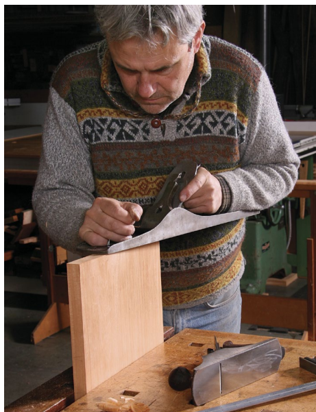
Refine the sawn surfaces. With the edges sawn, plane them smooth and square to the faces (above), and check for flatness with a straightedge (right).
