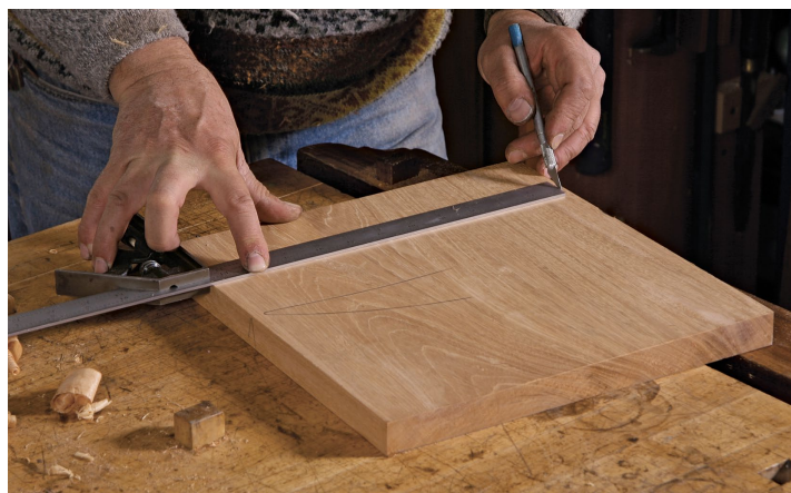
The second side. Using a combination square or a panel gauge, mark a line parallel to the reference edge.
