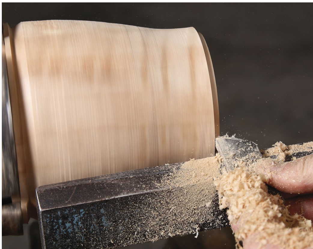
Rabbet the lip. Mahoney uses a skew to cut straight in and create a square corner.
