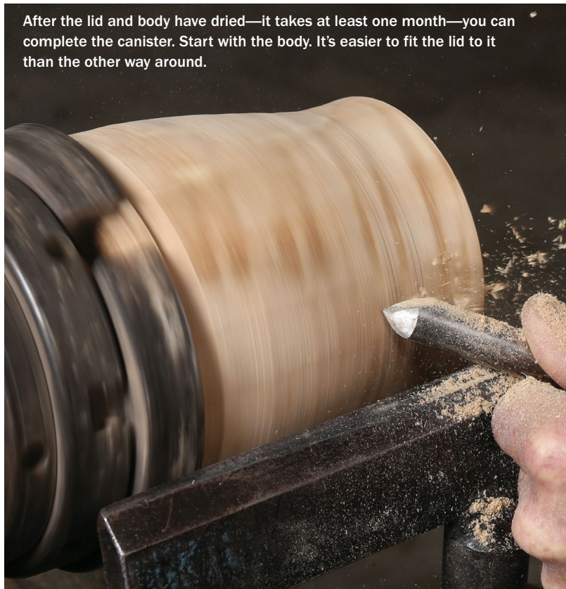
Shape the upper section. Using a \frac{1}{2} -in. bowl gouge, refine the shape. With figured woods, Mahoney keeps the shape simple, allowing the figure to do its thing.
