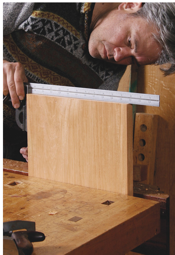
The second side. Using a combination square or a panel gauge, mark a line parallel to the reference edge.
