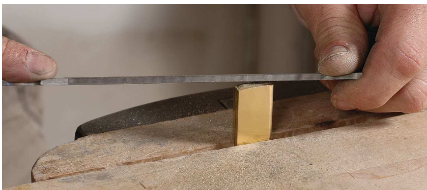
Soften the end. A file quickly and effectively gives the end of the spine a slightly rounded profile.
