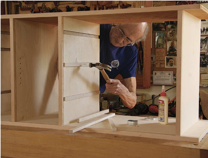
Fix the runners. Becksvoort glues in the maple runners, using brads instead of clamps to hold them in place.
