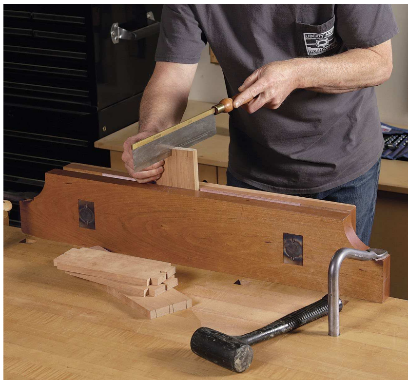
Never in the way. Unlike clamps, holdfasts don't hang off the front of the bench, which means you can position them so that they don't interfere with the work at hand.
