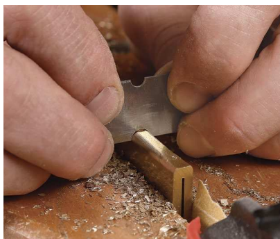
Round over the spine. A shopmade scraper rounds the spine to look like a traditional folded spine. The same effect can be done with files and sandpaper.
