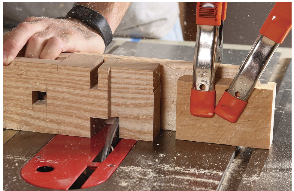
Two mortises in one. First cut the smaller through-mortise from the other side. Then cut the larger, stepped one on the underside.
