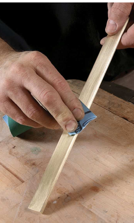
A quick polish. Whether it's a uniform sanding with 320-grit sandpaper or a full polishing, clean up the spine to get it ready for installation on the plate.
