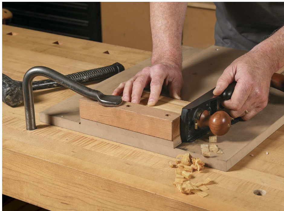
An extra hand for jigs. It takes more than a cleat on the underside of a sawhook or shooting board to keep it steady during use. A holdfast on top of the fence eliminates all movement.
