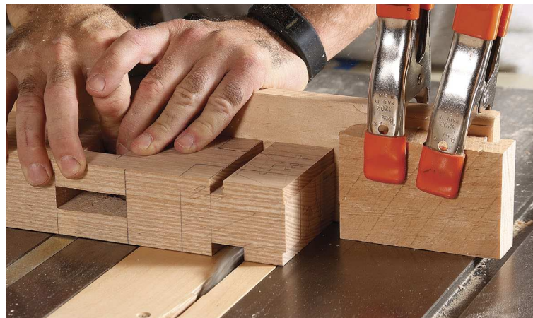
Cut the mating tenon with a dado set. With the blades set to cut the tenon's small shoulders, remove waste from the front and back of the post (left). Then raise the dado set and cut the long, thin tenon (below).
