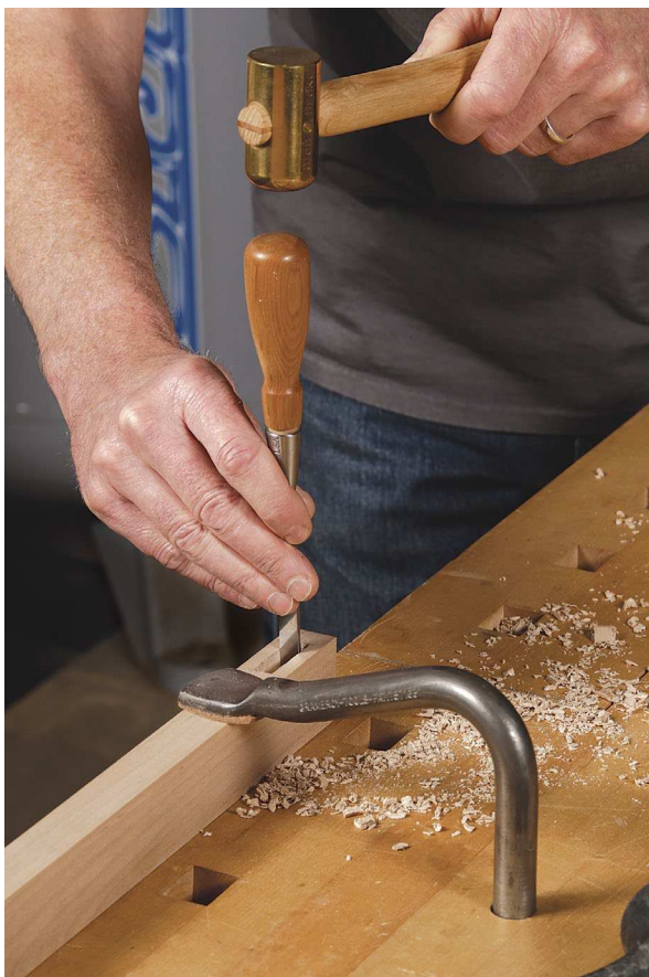
Hold tight for joinery. Whether you're paring dovetails (opposite) or chopping mortises (above), a single holdfast is often enough to prevent the workpiece from moving under the force of the chisel.
