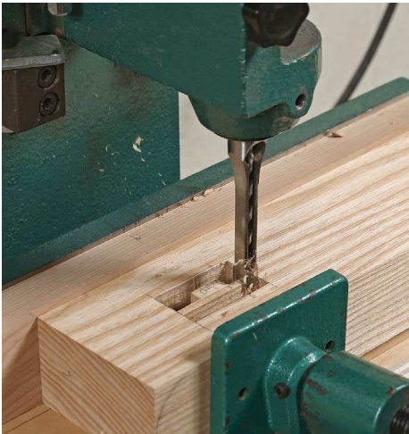
Two mortises in one. First cut the smaller through-mortise from the other side. Then cut the larger, stepped one on the underside.
