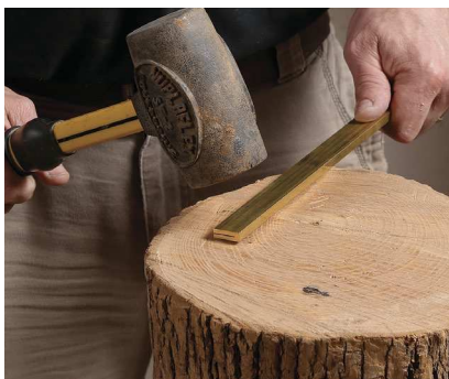
Pinching the spine. A few good smacks with a dead-blow mallet will tighten up the spine. Calisto uses a log as an anvil, but a sturdy bench works too.
