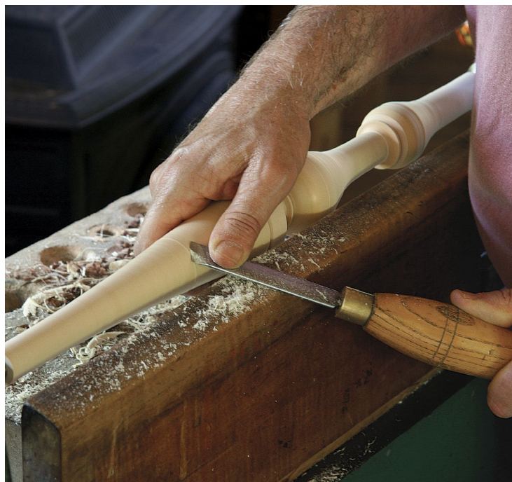
2. Then gradually draw the handle back until the tip engages and shavings appear.
