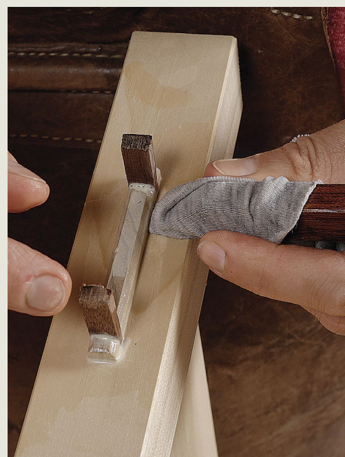
Chisel without the cloth. Shed the damp cloth and the chisel gets right into the corner to clean out the micro residue. This wooden chisel is used only when the glue is wet.
