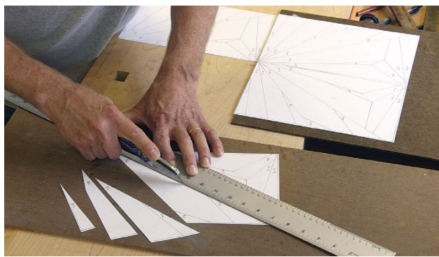
Nature's templates. Having drawn out the marquetry pattern, Lamb cuts up the component pieces to use as templates, which he'll glue to the veneer.
