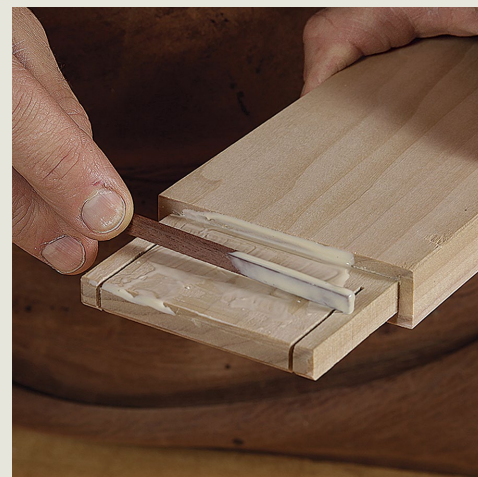
Spread glue with a thin wood scrap. Generously apply the glue inside the mortise and around the tenon.
