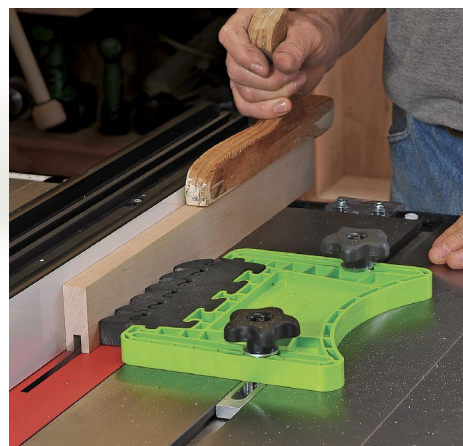
Foam support. The high-density foam fingers of Bow's FeatherPro do a great job holding boards tight against the rip fence for rips and dado cuts (shown).
