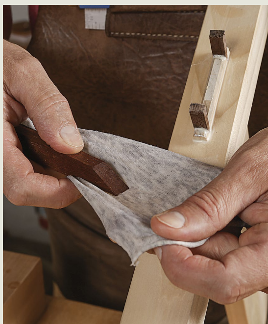
Straw and a wooden chisel again. After removing most of the fresh glue with a straw (above), Rousseau uses a piece of softer hardwood like walnut or mahogany, cut at an angle and wrapped in a damp cloth, to remove what's left (right).
