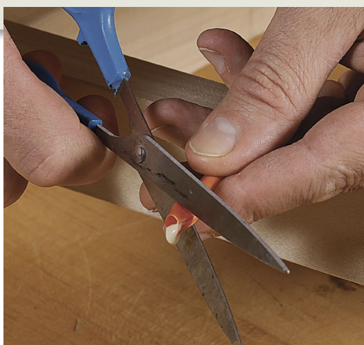
Straw and a wooden chisel again. After removing most of the fresh glue with a straw (above), Rousseau uses a piece of softer hardwood like walnut or mahogany, cut at an angle and wrapped in a damp cloth, to remove what's left (right).
