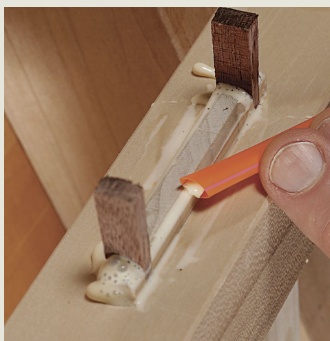
Straw and a wooden chisel again. After removing most of the fresh glue with a straw (above), Rousseau uses a piece of softer hardwood like walnut or mahogany, cut at an angle and wrapped in a damp cloth, to remove what's left (right).
