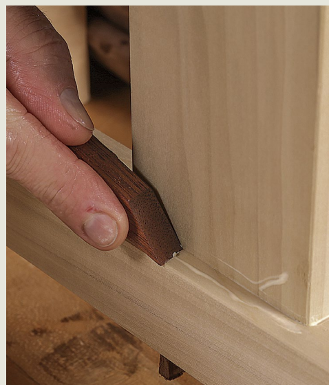
Chisel without the cloth. Shed the damp cloth and the chisel gets right into the corner to clean out the micro residue. This wooden chisel is used only when the glue is wet.
