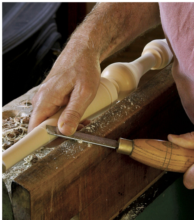
Keep it constant. With the cutting edge angled at about 45° to the long axis of the workpiece and the handle tucked close to your hip, move your body laterally to make a smooth cut.
