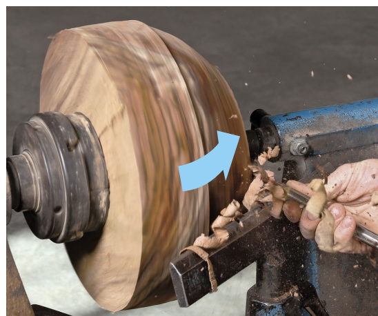
Rough-turn the bowl's outside. After turning the blank round using a ½-in. bowl gouge with a fingernail grind, begin to shape the bottom half so that you can turn a tenon. Cut from the middle of the blank toward the tailstock.
