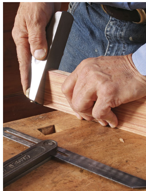
Set the angle with a bevel gauge. This setting (left) will guide the work. Only one end of each drawer front gets angled. Hack marks the angle on the drawer and planes slowly up to it (above).
