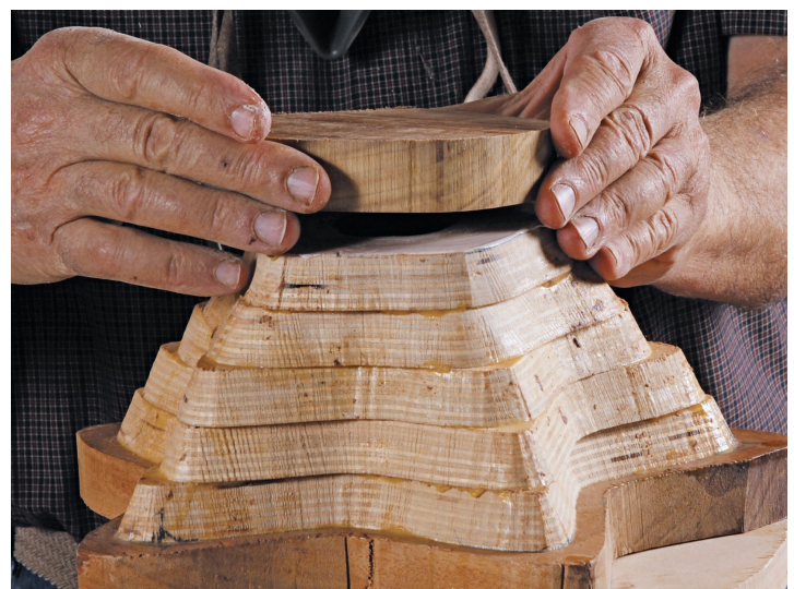
Glue on the bottom. Once the shaping and surfacing of the interior is complete, the bottom gets glued in place.
