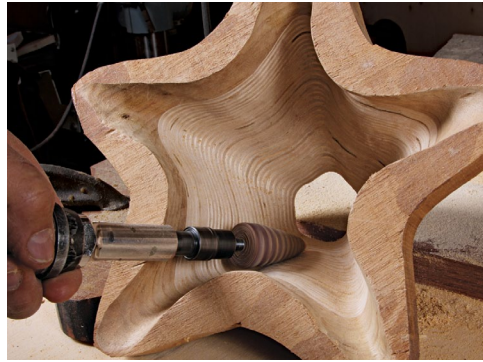
Move to the die grinder. Abrasive cones smooth the transitions between plywood layers and the faceted surface left by the angle grinder.
