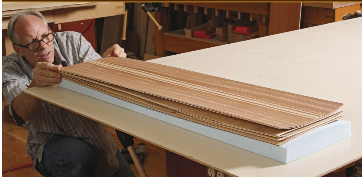
Straighten out the plies. Glue and stack the plies on the form, making sure they are parallel to each other and to the form's edge.
