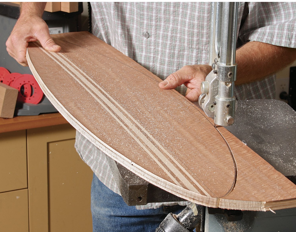
Cut it to shape. Cut the deck shape from the blank at the bandsaw (left), leaving the pencil lines. Then use a spokeshave or sandpaper to level the edges to the traced lines. Ease the top and bottom edges of the deck with a bearing-guided roundover bit (above).
