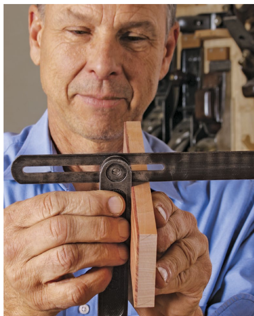
Angle the top and bottom too. The top and bottom edges of the drawer fronts get a small bevel (1°). Again, use a bevel gauge to guide the plane work (left). The drawer front should fit snug in its opening (below) before you cut the joinery.
