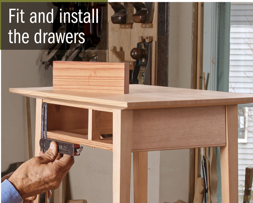
Set the angle with a bevel gauge. This setting (left) will guide the work. Only one end of each drawer front gets angled. Hack marks the angle on the drawer and planes slowly up to it (above).
