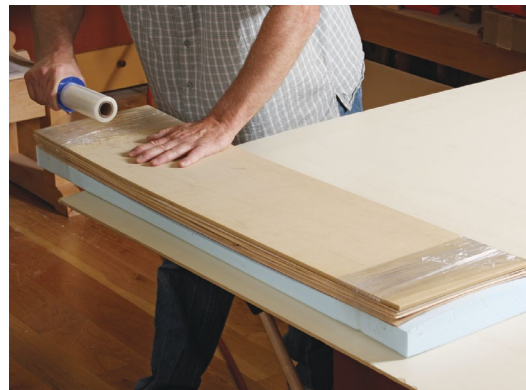
Wrap it. Before putting the whole form in the vacuum bag, wrap each end of the packet with plastic wrap to keep the sheet from moving.
