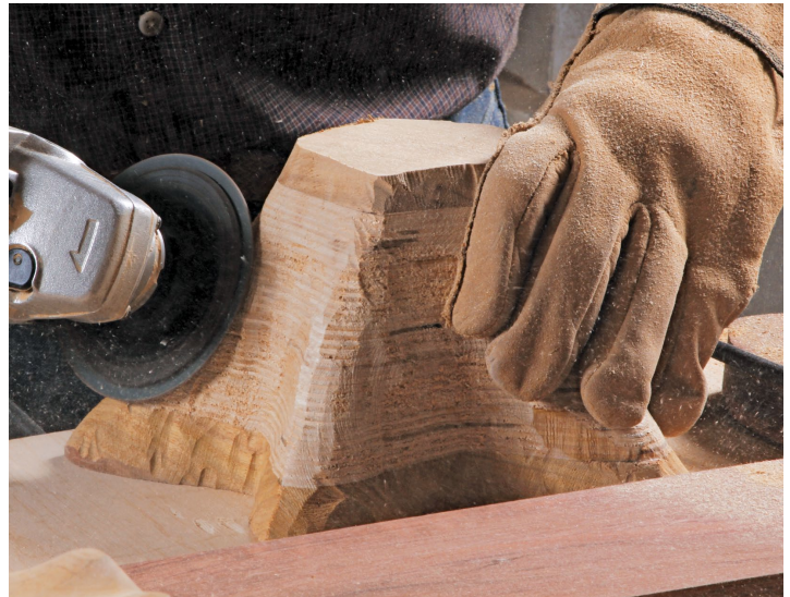
Smooth the transitions. Vesper uses an angle grinder with a resin abrasive disk to refine the shape and smooth the surface.
