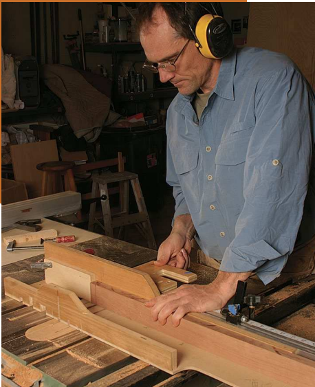
Cut tenon shoulders first. Edmundson uses a narrow, shopmade sled to cut the tenon shoulders, with a stop block clamped to it.
