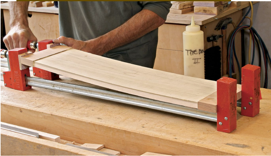
Solid ends on a core of plies. Use biscuits to attach the solid end blocks to the core of poplar plies (left). After the glue-up, plane and scrape the blocks flush to the core (above).
