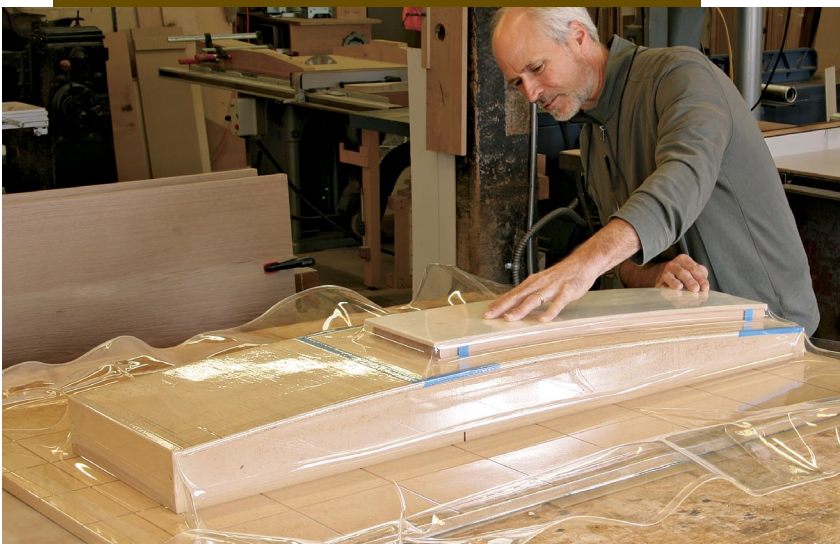
Back in the bag. When it's time to apply the front and back show veneer, the core goes back in the vacuum bag (left). After the glue-up, Wurtz routs the face veneers flush with a laminate trimmer (above).
