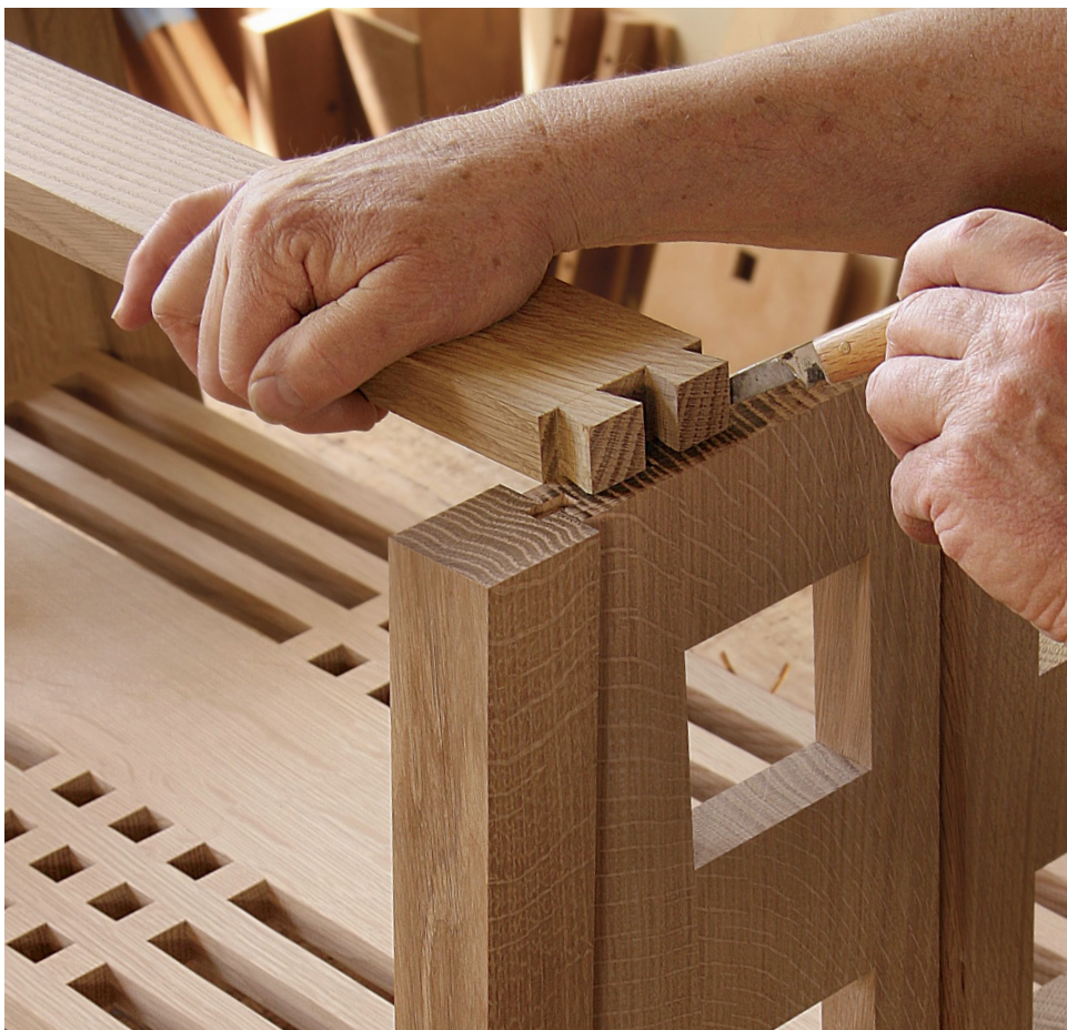
Top lock. Twin dovetails secure the rail to the top of the end panel. Along with the corbel, which acts as a tusk tenon, the rails give the table base mechanical locking at top and bottom.
