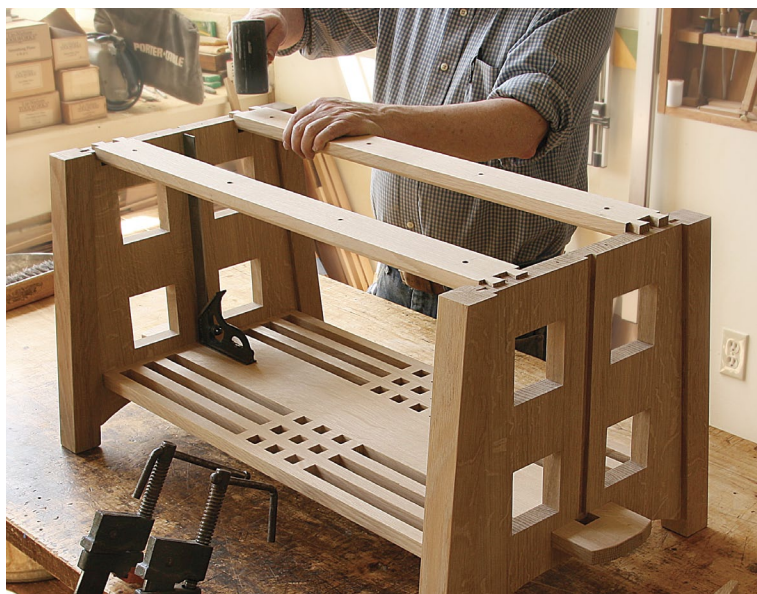
Assembly starts without clamps. Rodel knocks the rails into place and checks the structure for square before applying clamping pressure.
