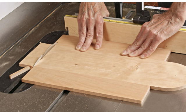
Three-part back. Shape the back's half-round top section before gluing on the two narrower side boards. Then trim the whole back to length and width.
