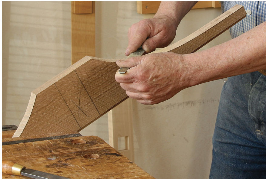
Fair the corbel curves. After bandsawing the corbels close to final shape, use rasps and files to smooth the curves. Then cut the two corbels to length.
