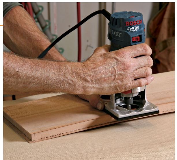
Back in the bag. When it's time to apply the front and back show veneer, the core goes back in the vacuum bag (left). After the glue-up, Wurtz routs the face veneers flush with a laminate trimmer (above).
