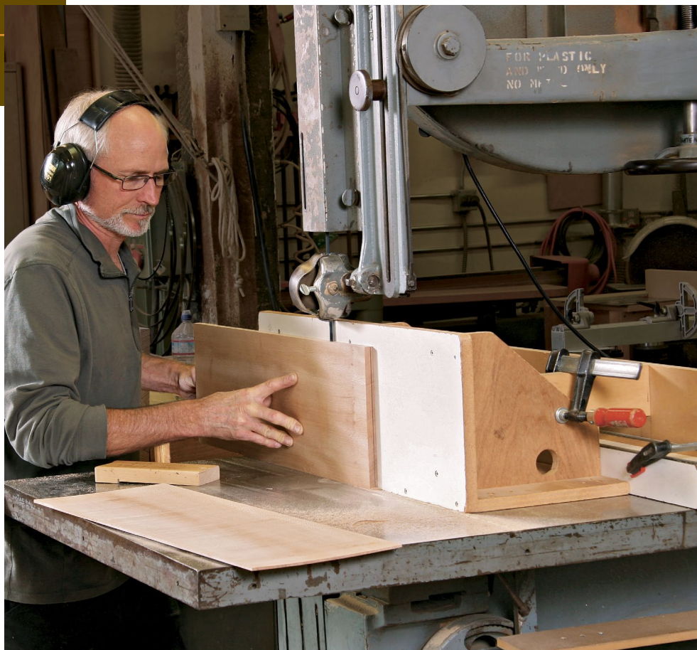
Shopsawn veneer. Cut the show veneers on the bandsaw, jointing the plank between slices. A tall shopmade bandsaw fence dedicated to resawing ensures uniform slices when cutting the \frac{3}{32} -in.-thick show veneers.
