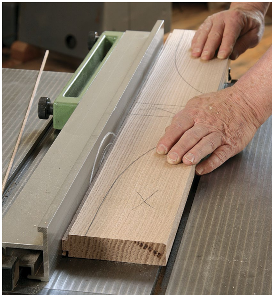
Double-length blank. With both corbels laid out on a single blank, use the tablesaw to cut a tongue along one edge. Then bandsaw the curves.
