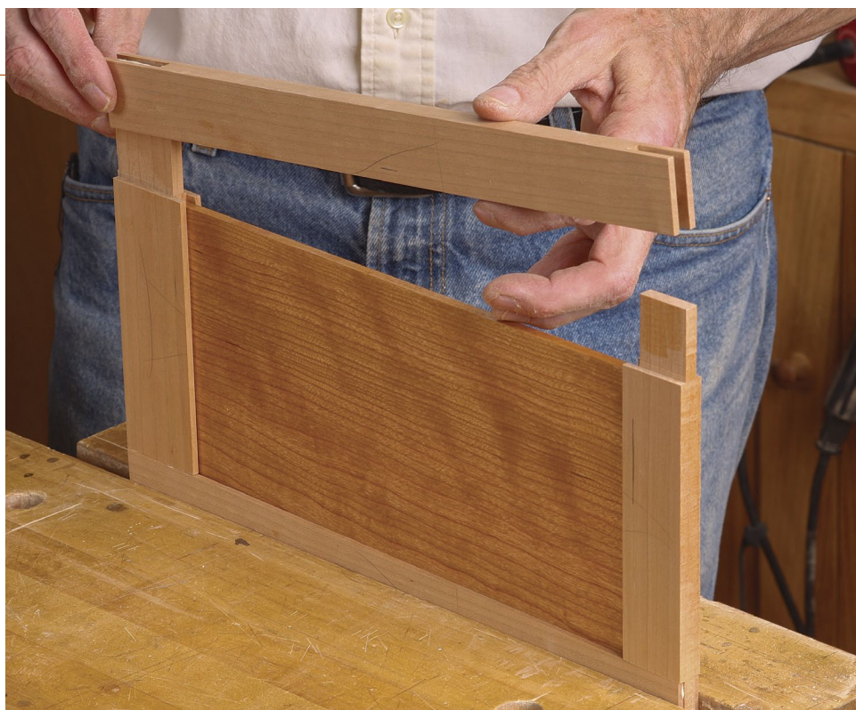
Diminutive frame and panel. After applying finish to the \frac{3}{4} -in.-thick door panel, drop it into place as you assemble the door frame.
