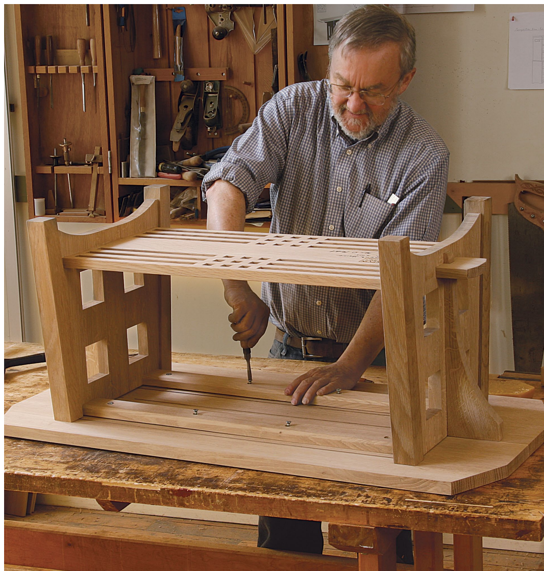
That's it. Rodel screws the base to the tabletop (below). Since the end panels and shelf will move in concert with the top, there's no need to accommodate wood movement with elongated screw holes.
