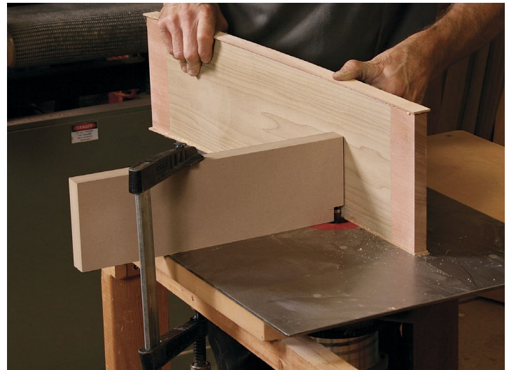
Solid ends on a core of plies. Use biscuits to attach the solid end blocks to the core of poplar plies (left). After the glue-up, plane and scrape the blocks flush to the core (above).
