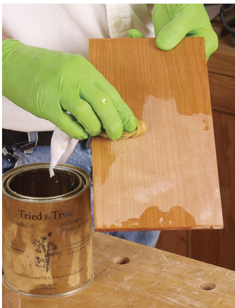
Diminutive frame and panel. After applying finish to the \frac{3}{4} -in.-thick door panel, drop it into place as you assemble the door frame.
