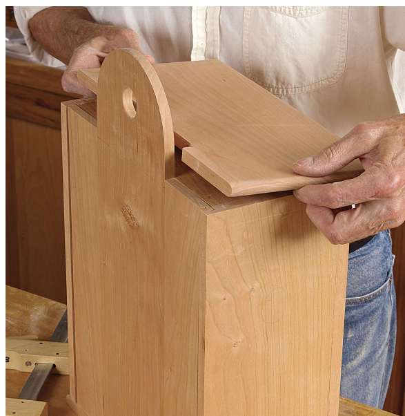
Two tongues. Two passes on the tablesaw—one with the back standing on edge—create the tongues on the sides of the back.
