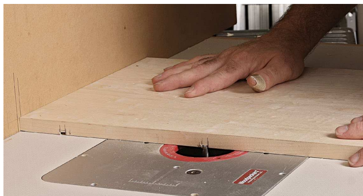
Dadoes for dividers. Use a \frac{1}{4} -in. straight bit to cut the stopped dadoes into the case shelves for the vertical dividers that will form the drawer box.
