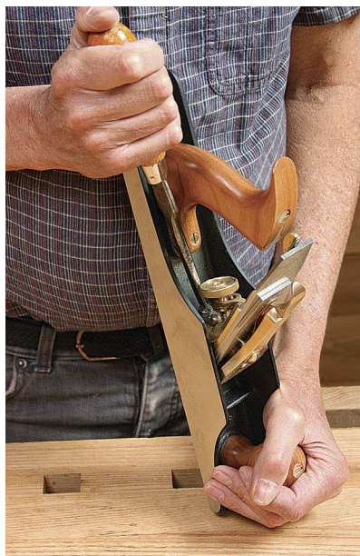
You shouldn't have to remove the blade. Mouth adjustments are made by moving the frog or by sliding a toe, or shoe, at the front of the plane. Planes with a Bedrock-style frog (or similar) let you move the frog with the blade in place by turning screws at the back of the frog. With planes that use a sliding toe to adjust the mouth opening, like the Veritas Custom No. 5, you never have to remove the blade for mouth adjustments.
