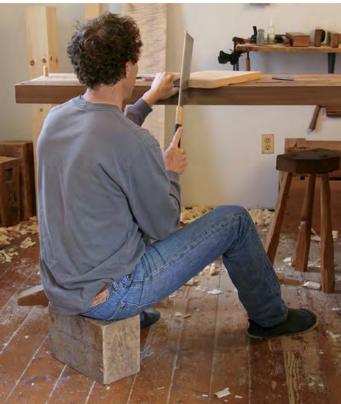
The lowdown on dovetails. Hunter does some repetitive joinery while sitting on a low block or stool. This posture brings his eye close to the layout lines, and the downward stroke pulls the workpiece to the benchtop, eliminating vibration.
