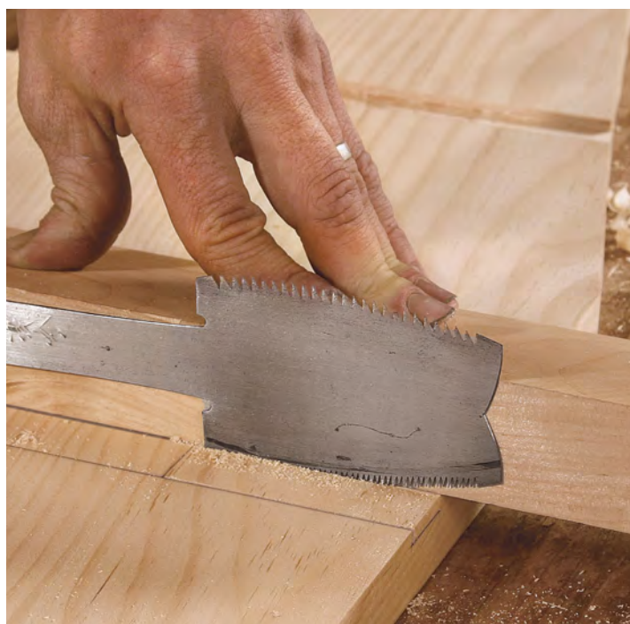
A good guide. The azebiki saw, with its short, wide blade, easily follows a guide block for straight or angled cuts.
