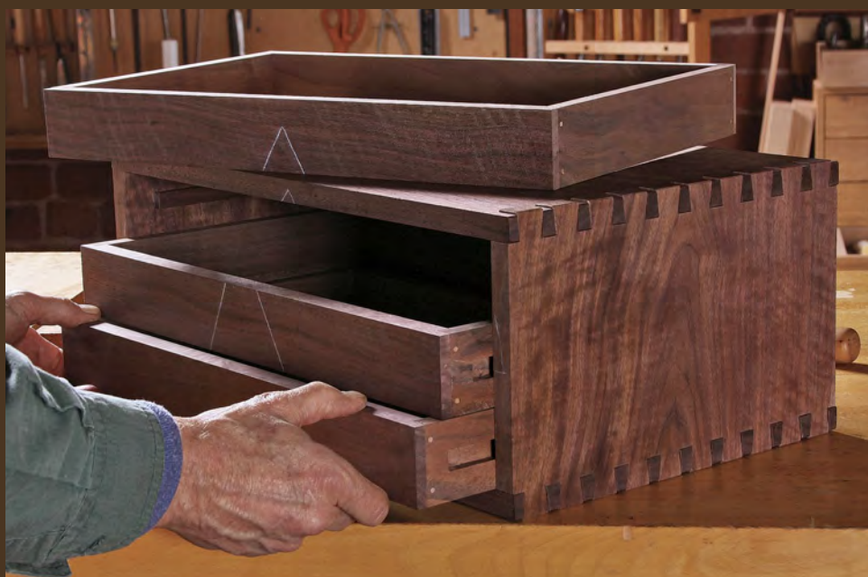
Fit the drawers. Plane the faces of each drawer side until the drawer slides smoothly into its opening. Then plane the bottom edges of the drawer sides, and the top and bottom edges of the drawer fronts, to adjust the gaps between the drawers.
