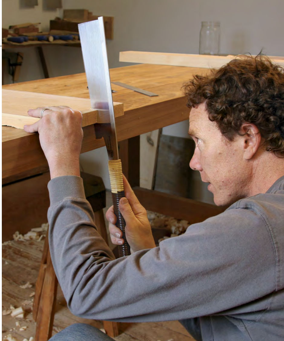
The lowdown on dovetails. Hunter does some repetitive joinery while sitting on a low block or stool. This posture brings his eye close to the layout lines, and the downward stroke pulls the workpiece to the benchtop, eliminating vibration.
