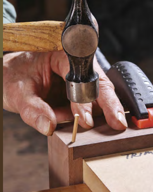
Reinforce the joinery. To add strength and a decorative touch, Rogowski seats two pins made from maple through the drawer side at each corner.
