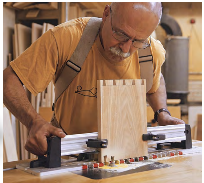
Dovetails on the router table. The Leigh RTJ400 is used with a table-mounted router, which makes for stable and quick dovetailing.
