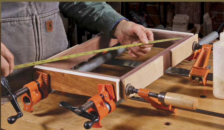
Glue up the drawers. Use cauls, apply even clamping pressure, and check for square.
