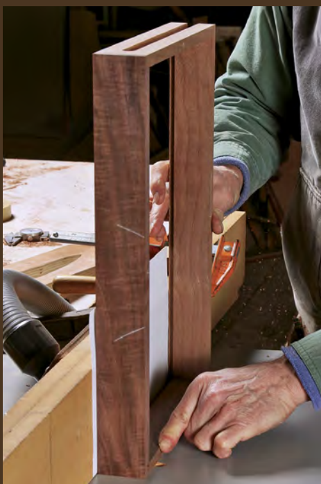
Route the runner grooves. Make them in two passes, shimming the fence for the first pass. Aim for a tight fit.
