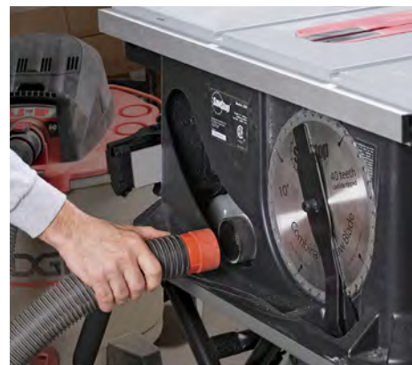
Great dust collection. With a shop vacuum hooked up and the blade guard in place, the saw collected just about all of the dust and chips created.
