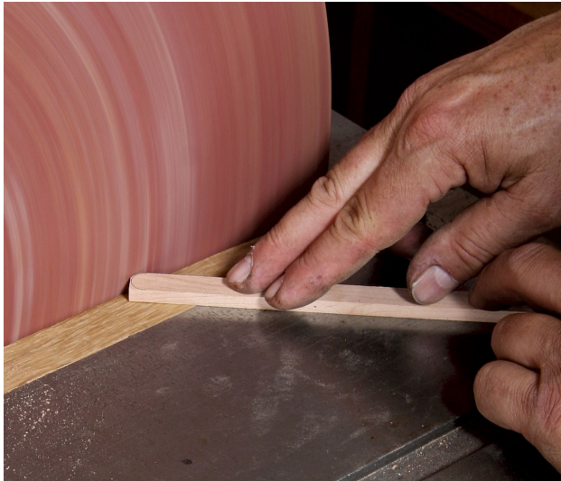
Round the nose. After slicing the blank into runners, sand the leading end round to match the end of the groove. Check the fit with a stopped test groove.
