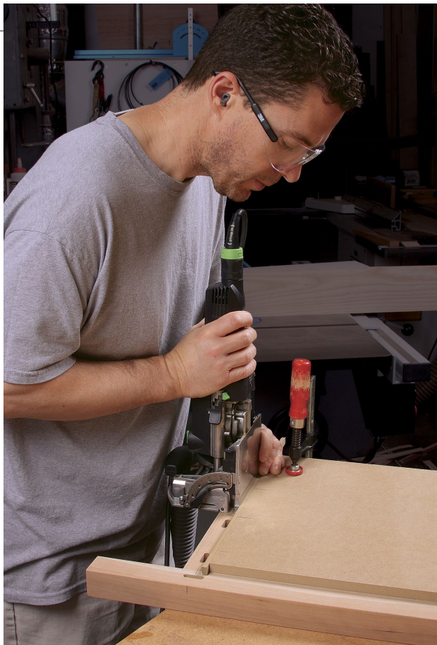
Fence ensures perfect alignment. Thibodeau uses the Domino vertically against the fence, following the tick marks.
