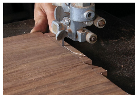
Bandsaw to the haunch line. A slightly rough end-grain cut on the haunch is fine, because it won't bottom out in the housing.
