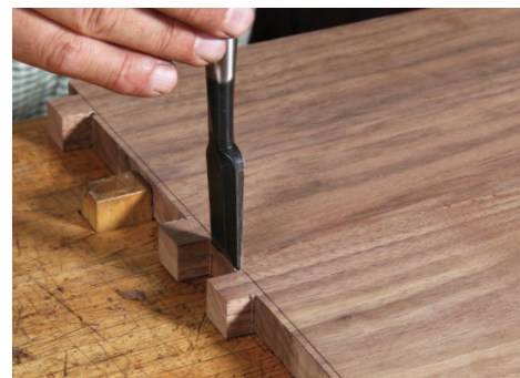
Chisel cleanup. Pare precisely to the baseline on the outside edges of the board and between the center tenons.
