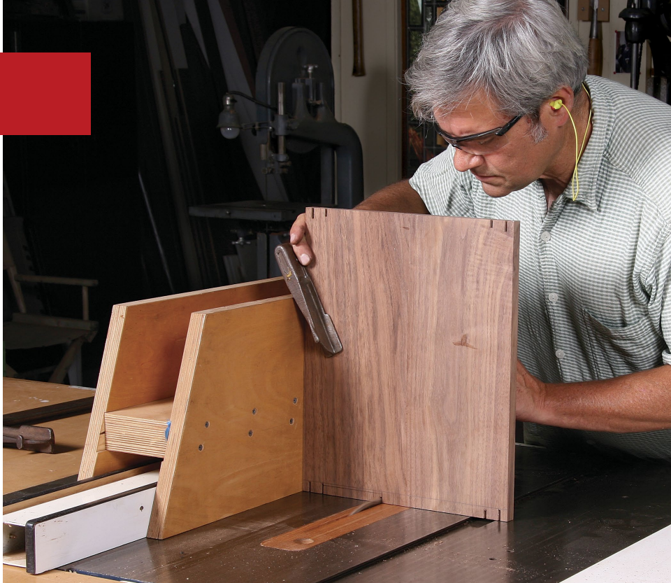
A jig for the cheeks. Cullen cuts the tenons to width on the tablesaw using his shopmade tenoning jig. For drawings of a similar jig, see p. 69.
