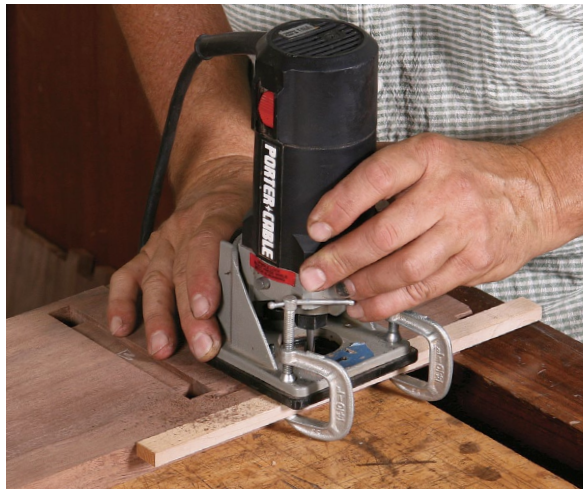
Easy transfer. With the divider dry-fitted into the sides, transfer the location of the groove for the back panel.
