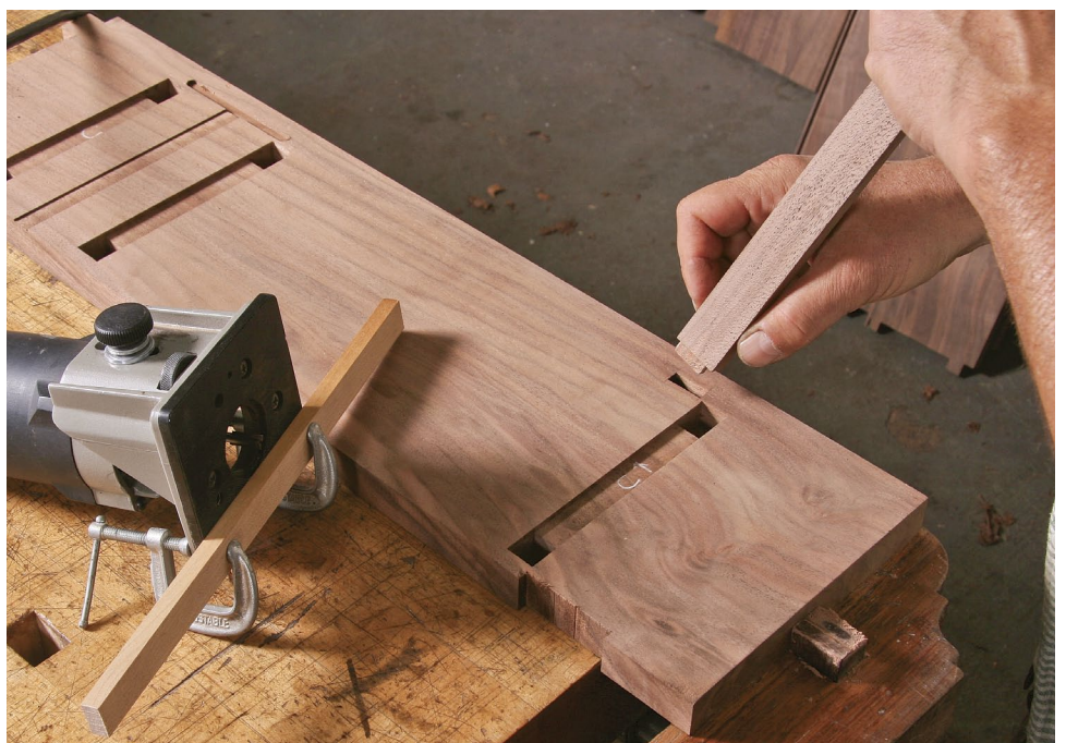
Small router for a stopped groove. Cut the stopped groove for the back panel with a detail router fitted with a fence (left). The small mortise for the book stop's tenon (below) can be routed with the same setup used to cut the stopped groove for the back panel.
