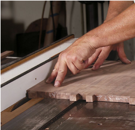
Divider and top shelf get grooved. A dado head creates the \frac{1}{4} -in.-wide groove to receive the back panel of the drawer pocket.
