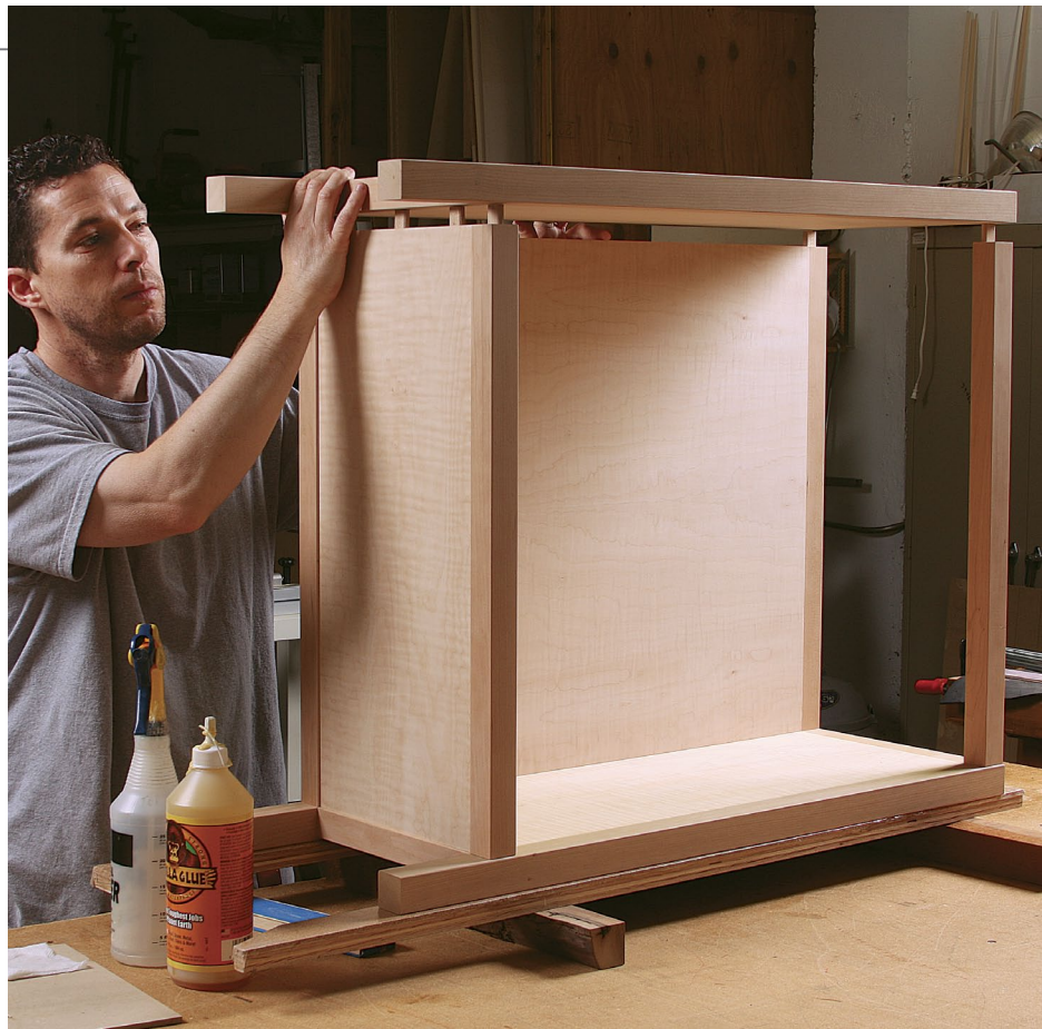
Add one side at a time. Attach one side, clamp it, and let it dry. Then add the front rail and the final side as shown. Again, cauls protect the sanded surfaces.
