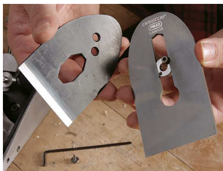
Easy-to-set chipbreaker. The chipbreaker registers on a round "blade carrier" attached to the blade, so you can quickly reattach the chipbreaker after sharpening the blade.
