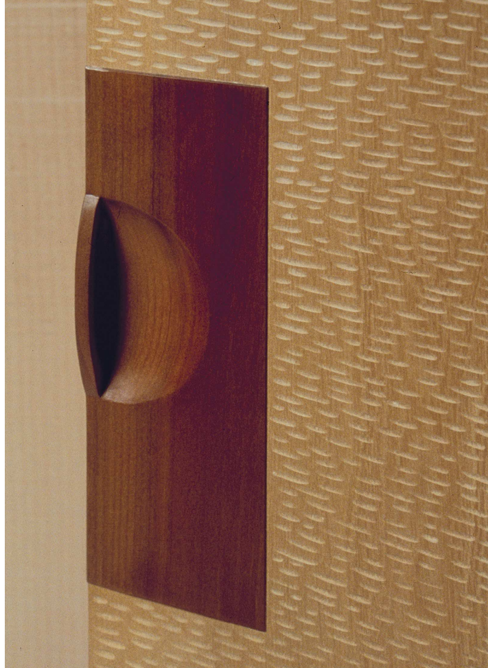
Great gouging. Inspired by the gouged surface of a wall-hung wooden sculpture, Norris experimented with various gouging patterns (left) before settling on the subtle, all-over flecking he used on his liquor cabinet.
