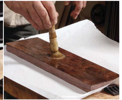
Brush on the glue. Latta spreads hot hide glue on the drawer front and the veneer (left), and quickly sets it in place. Then he brushes glue on the face of the veneer (above) to fill the pores and lubricate the hammer. Placing paper on the benchtop beforehand keeps glue cleanup to a minimum.
