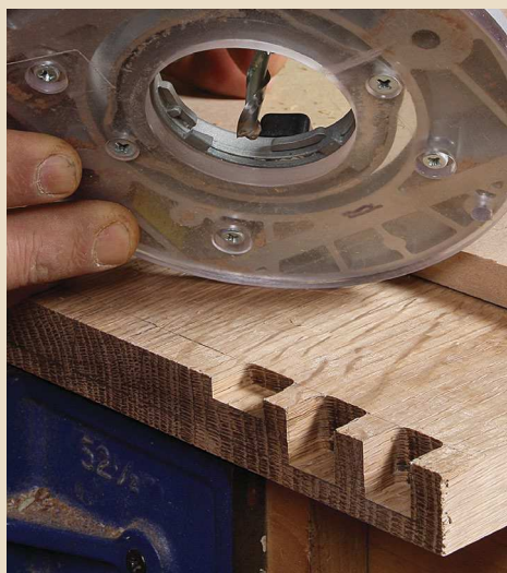
Router work. Rodríguez removes most of the waste between pins using a plunge router.
