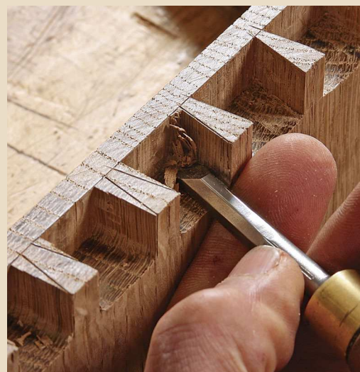
Pare to perfection. Once the router is unplugged, he trims each pin, ensuring that all the corners of the joint are clean and free of debris.
