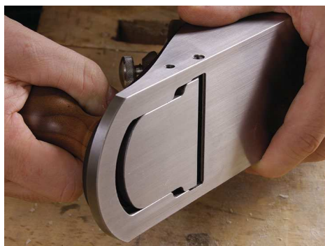
Adjustable mouth. Changing from a narrow opening for light shavings to a wide one for heavy work is quick and simple because you don't have to move the frog, as you would on traditional bench planes.
