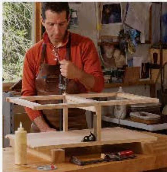
Add dividers. Putting the drawer dividers in place at final assembly would be nearly impossible.
