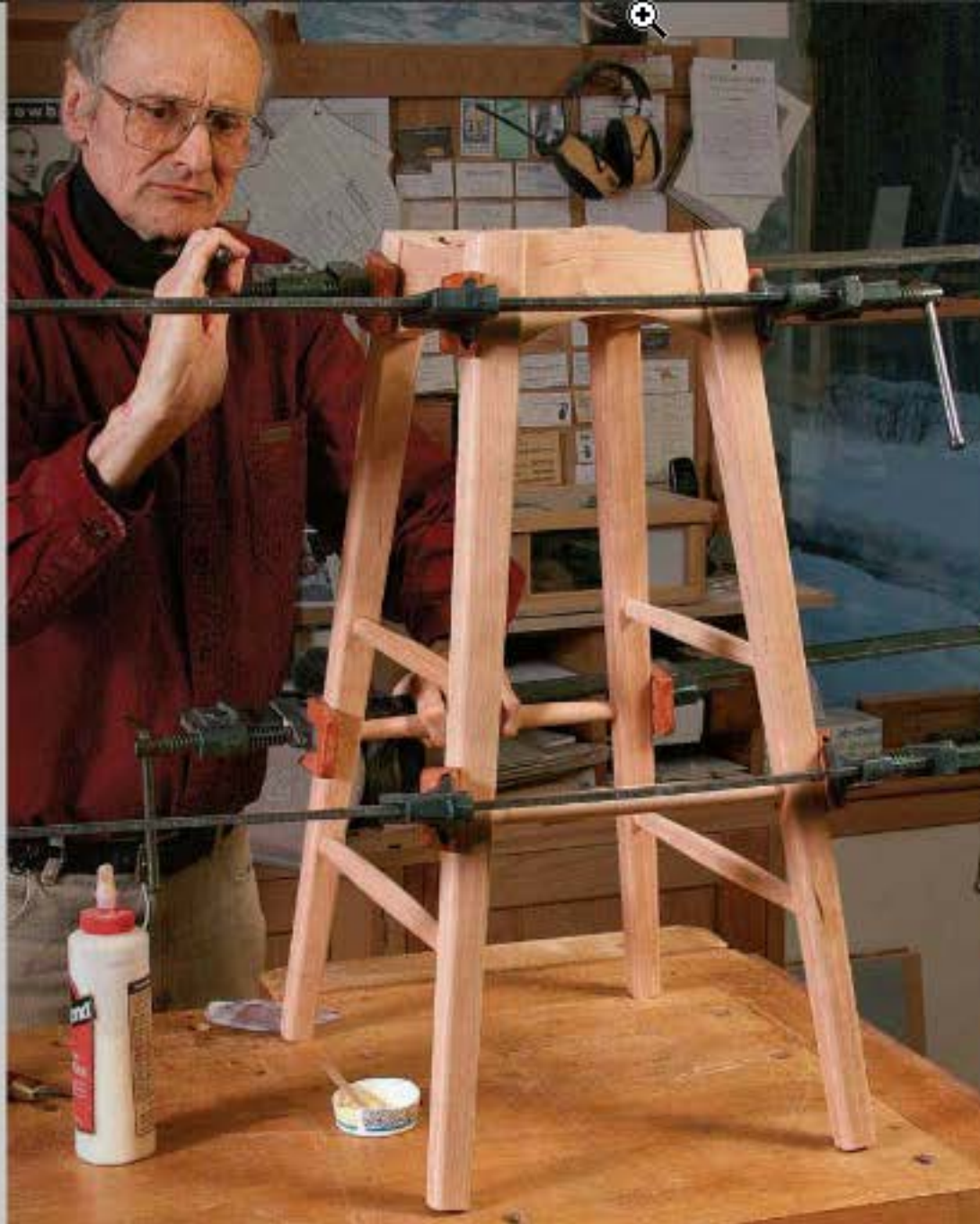
The second gluing. After attaching screw blocks inside the seat rails, do the final assembly of the stool.
