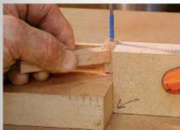
Hold still while I drill. A stepped fence and a stick with a V-shaped notch hold the post for drilling. The hole accepts the metal pin that will be epoxied in and takes the place of a tenon.
