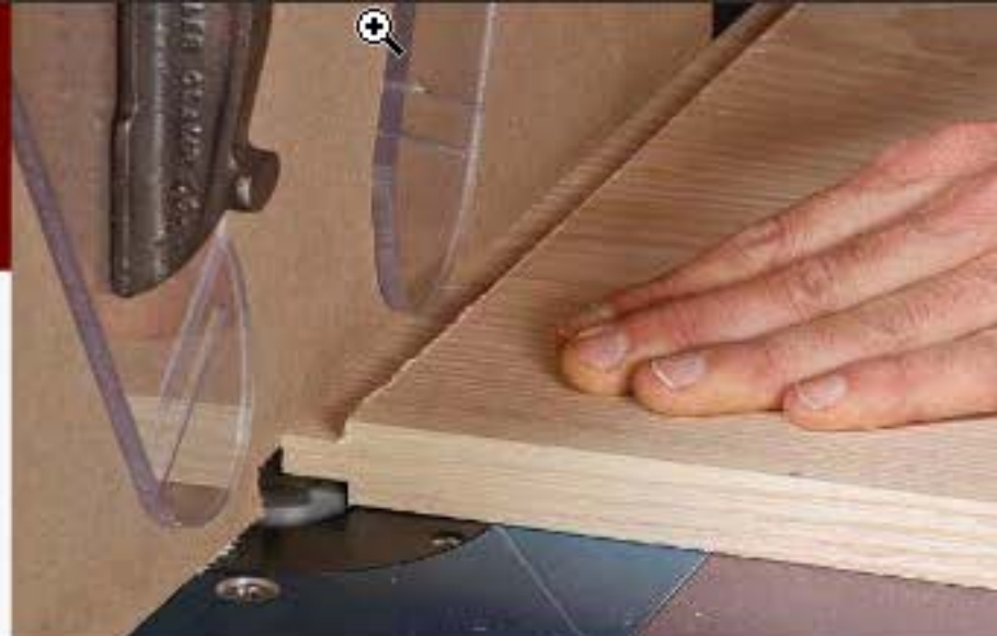
Two rabbets make a tenon. Rousseau cuts to the final depth and width on each side in a single pass.
