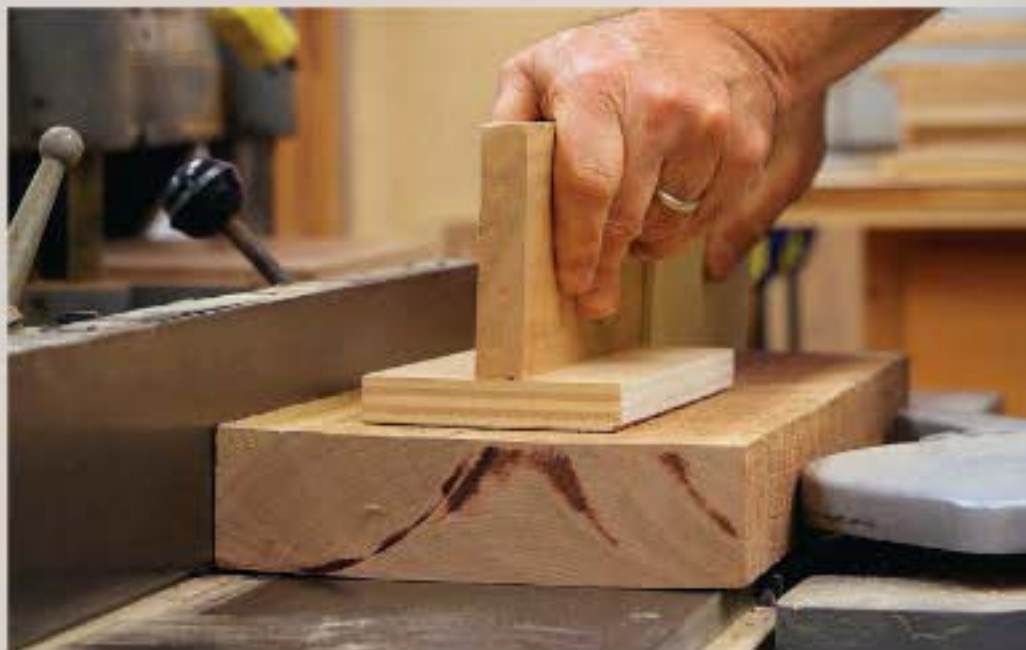
Don't rock it. To keep the board from rocking, apply pressure directly over the center of the board and slowly joint the face.
