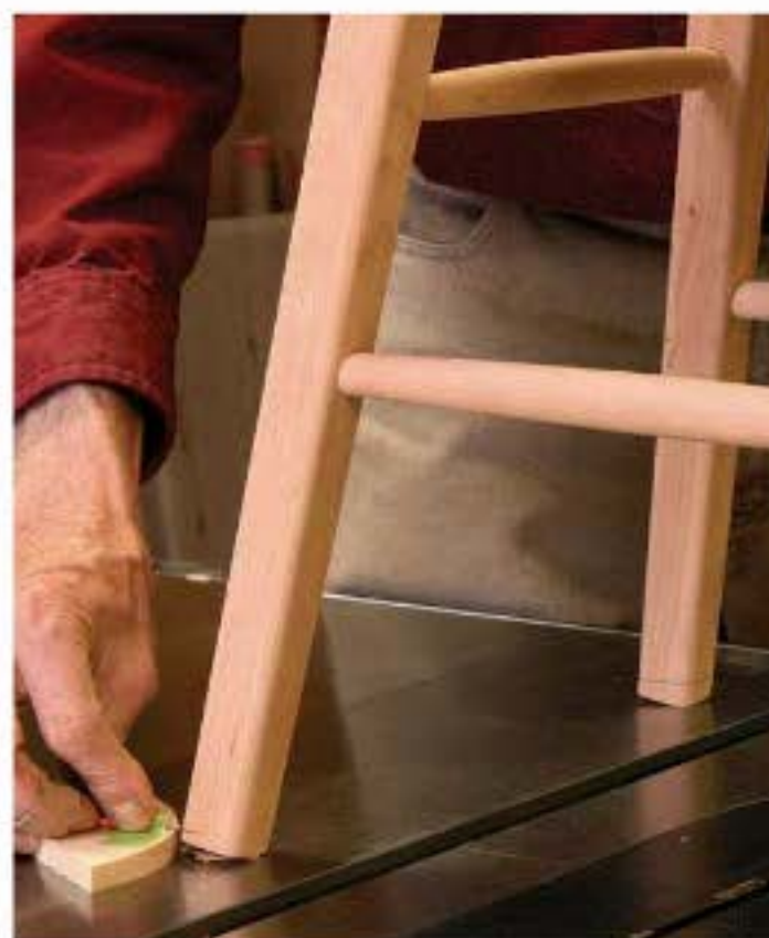
Wobble check. To eliminate rocking, trim all four legs in the same plane. Holding the stool steady on a flat surface, trace around each foot with a pencil held on its side and elevated on a scrap. Cut to the lines on the bandsaw, and follow up with rasps and files.
