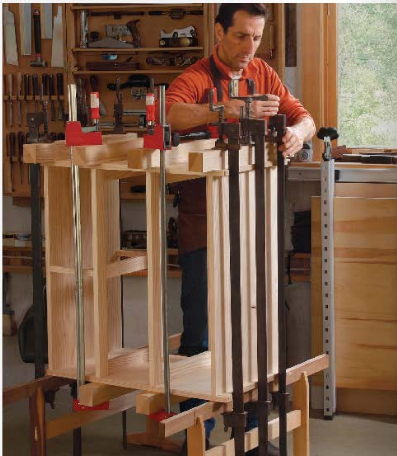
Add dividers. Putting the drawer dividers in place at final assembly would be nearly impossible.
