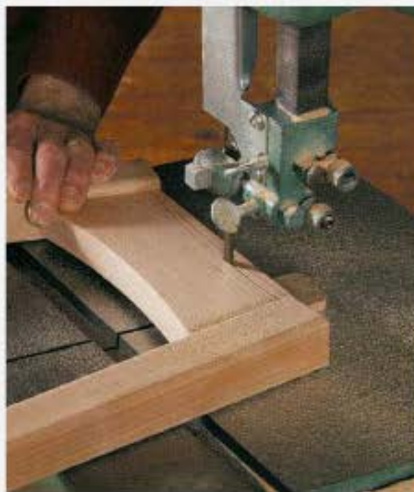
The top edge must mirror the seat. Trace the curve of the seat onto the legs and seat rail of the front and back units (left). With the subassembly riding inside face down, and the bandsaw table tilted 5\frac{1}{2}^\circ , cut along the curved line for the scooped seat (above).
