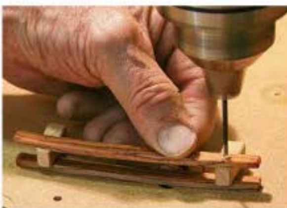
Drill straight through. With the pull dry-fitted and with a sacrificial table to back up the cut, drill right through both bars and the post with a 1/16-in.-dia. bit.
