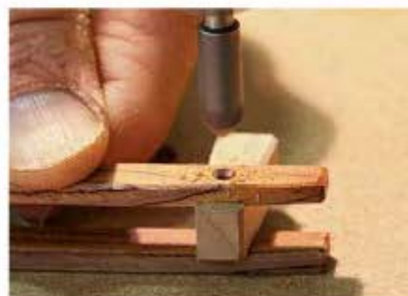
Quick chamfer. A countersink bit in the drill press makes a clean, decorative chamfer at the mouth of the pin hole.
