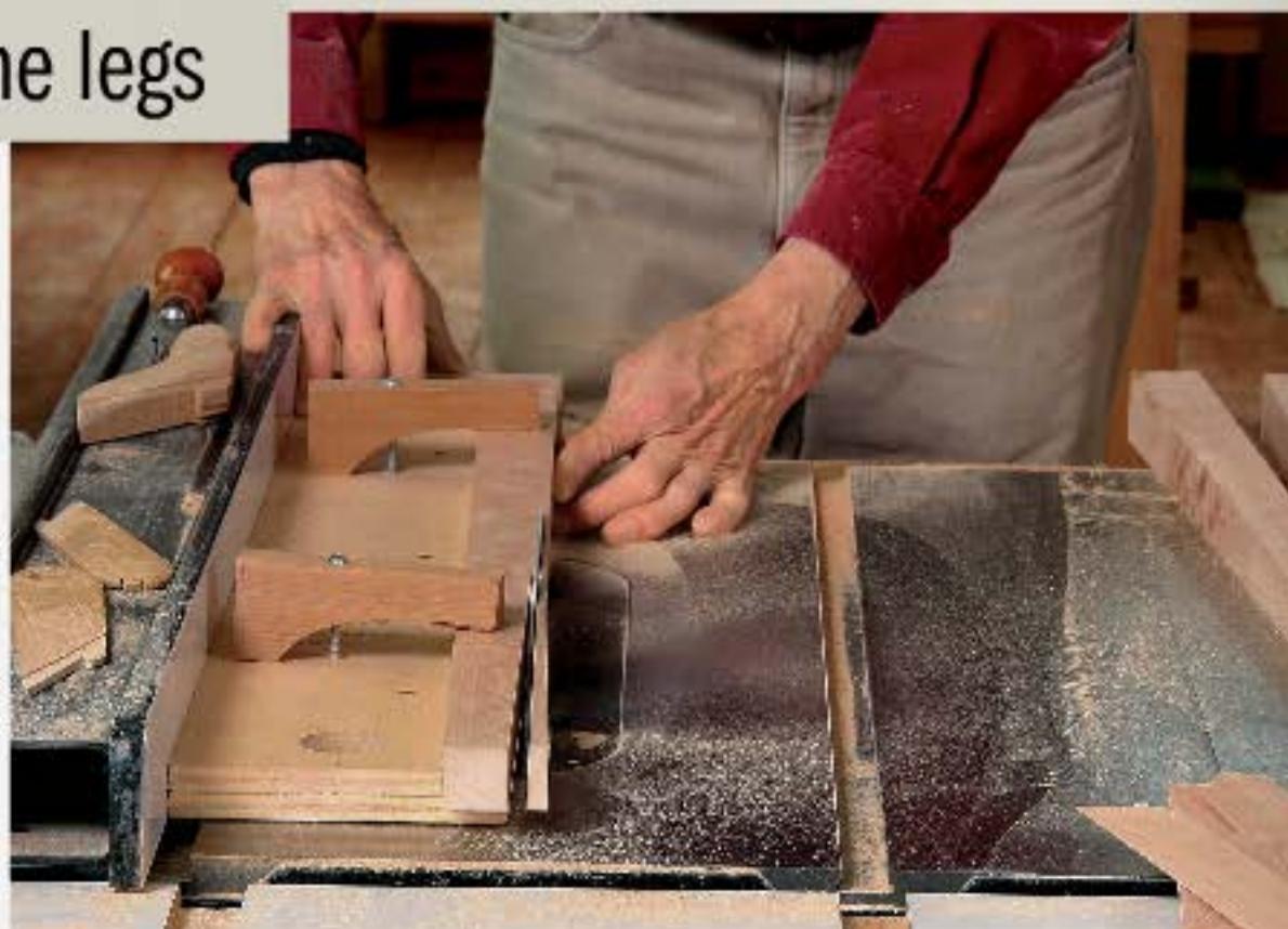
Taper two sides. Using a shopmade tapering jig, Becksvoort tapers the two inside faces of each leg. Then he cuts the mortises and rounds over the long edges of the leg on the router table.
