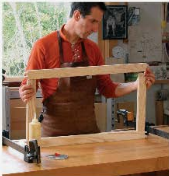
Begin with the web frames. Only the joints at the front get glue. The back joints float to accommodate wood movement.
