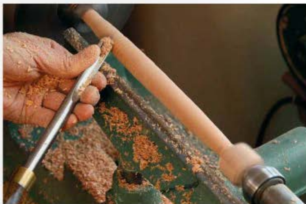
Make that rung a cigar. After turning the square blank to a cylinder with a roughing gouge, use a smaller gouge to taper the rung to a gentle cigar shape.
