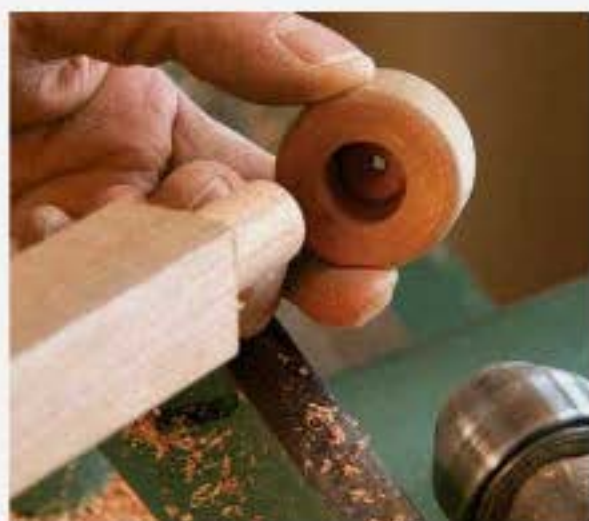
Clever doughnut. A scrap with a \frac{5}{8} -in.-dia. recess drilled into it helps mount the rung on the lathe. The small, through centerhole seats on the lathe's dead center.
