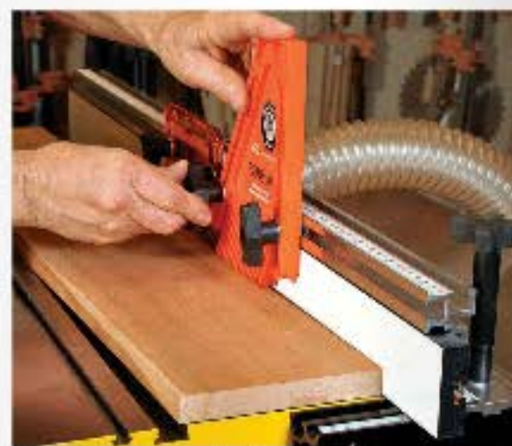
Versatile fence. Featherboards, jigs, and stops can be attached to the front of the fence, and on top of it.
