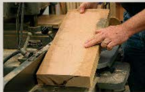
Only the high spot. Joint just enough to create a stable surface for flattening the opposite face or for resawing.
