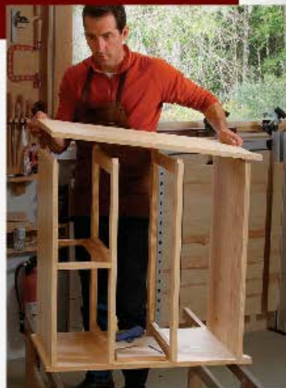
One side at a time. Leave the joints for the second side dry until you have all of the joints on the first side together.
