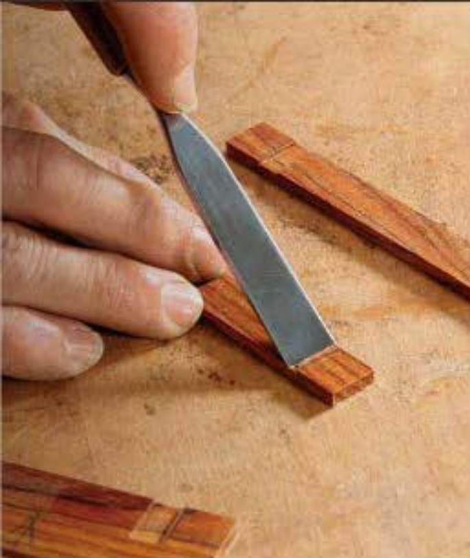
Adjust the shoulders. After dadoing the inside face of the bars at the tablesaw, use a chisel to angle one shoulder to match the post.
