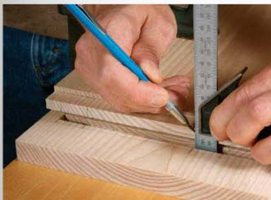
Transfer the mortises. Pressed against the mortise's wall, the blade of a combination or try square shows where to mark for the tenon width.
