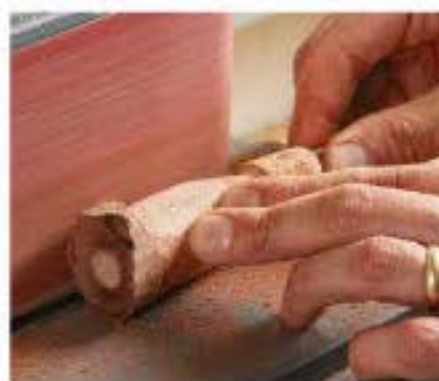
Clean up the leather. With the glue dried, sand the leather flush with the handle (above) and round over the pommel for a comfortable grip. To apply polyurethane to the handles, dip them into the can and then place the handles in a simple shopmade rack to dry (right)
