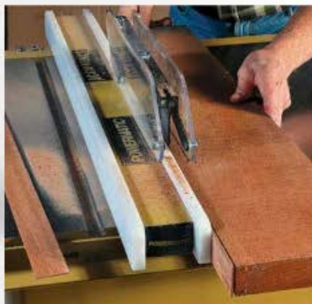
Blade guard works for narrow rips. The split design of the guard allows one side to lift and clear the fence. The other side stays down to cover the blade.
