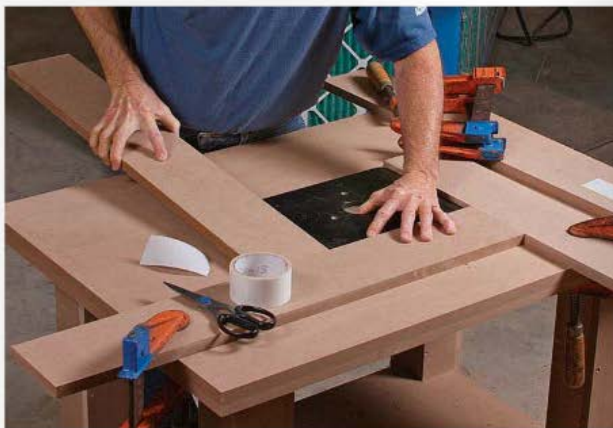
Flip the top and fit the last two strips. Push the first two strips against the base before clamping on the last two, making sure they are touching the base too. If their outside edges don't line up perfectly, just hit them with a flush-trimming router bit afterward.
