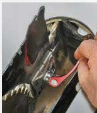
Cam-clamp convenience. The blade-guard assembly and riving knife can be switched out easily by flipping a lever.
