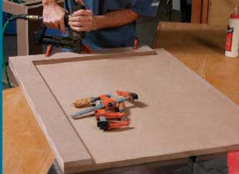
Attach two strips. Glue and nail these on with the tabletop upside down. Line up their edges flush with the top.
