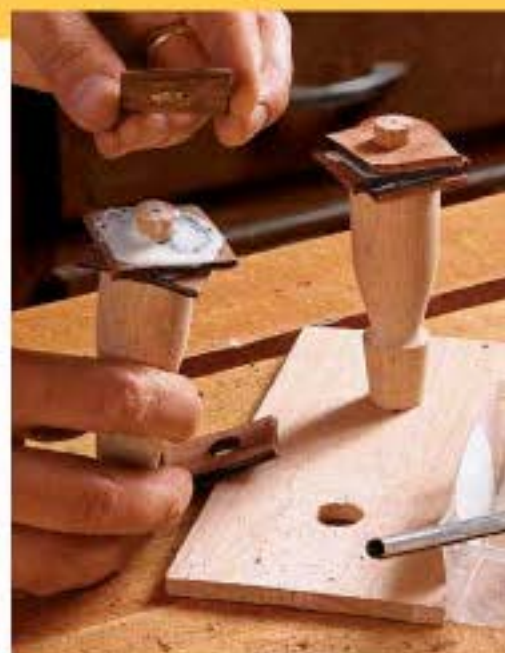
Stack them up. Put a coat of Titebond III between each layer of leather, stacking them three high, and then place the handles in the clamping caul.
