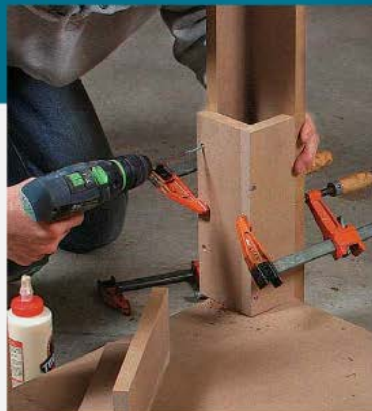
Stage two. Add the next bracket section as before, with glue on every joint, and then attach the second shelf.
