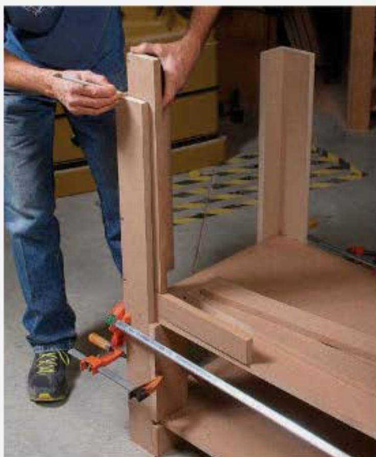
Measure for the final bracket section. To ensure that the tabletop support structure ends up flush with the tops of the legs, Adams puts one piece of that structure on top of the second shelf, stacking the final bracket section on top of it to mark its exact length (above). Do that for each corner of the table individually, in case there are differences, and then cut and attach the final bracket sections.
