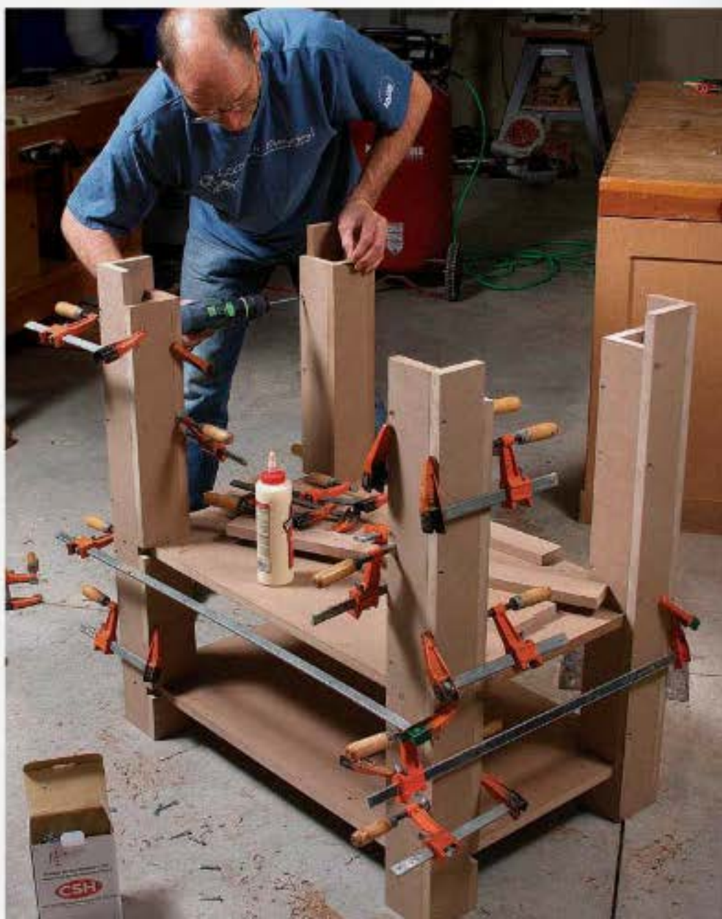
Stage two. Add the next bracket section as before, with glue on every joint, and then attach the second shelf.
