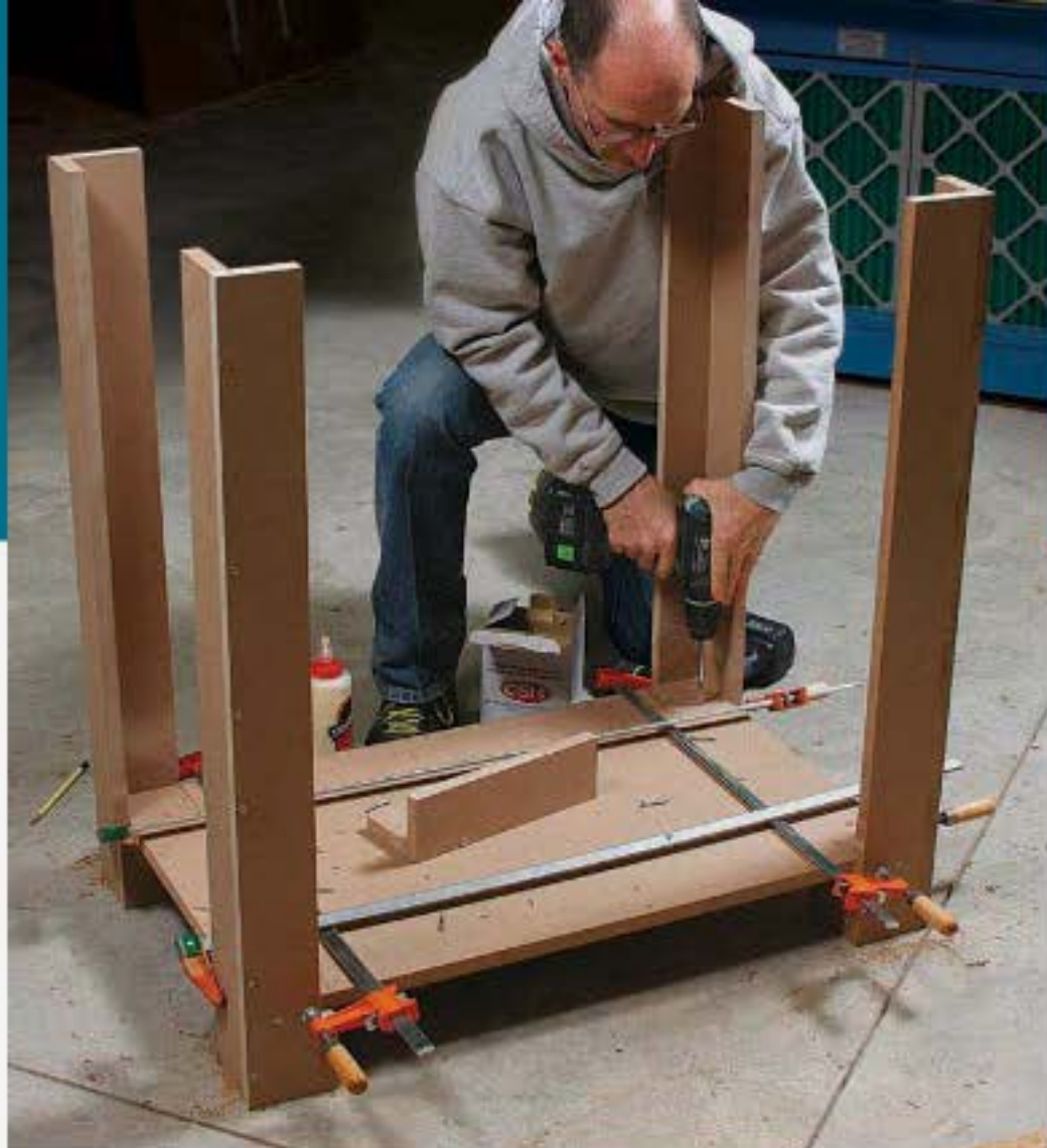
The first shelf connects the legs. Attach it by screwing in from the outside of the legs first, then down through the shelf as shown into the bracket section below.
