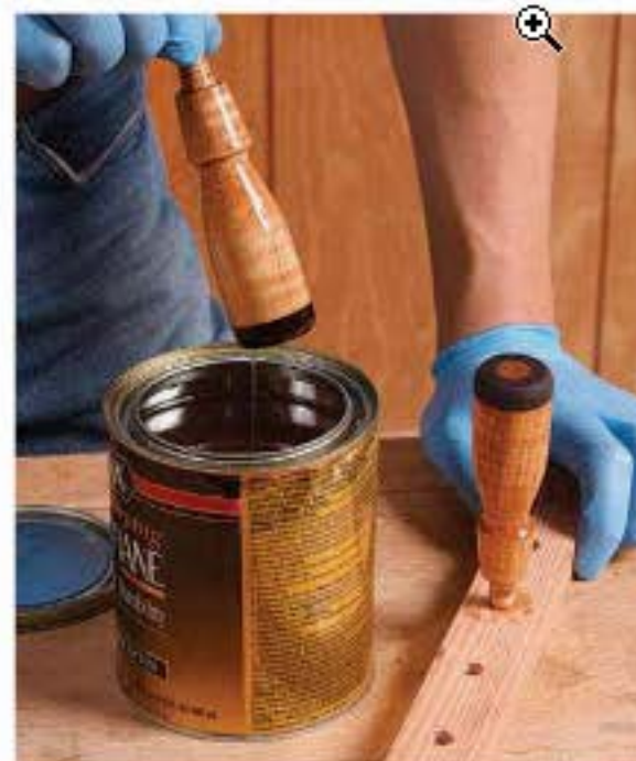
Clean up the leather. With the glue dried, sand the leather flush with the handle (above) and round over the pommel for a comfortable grip. To apply polyurethane to the handles, dip them into the can and then place the handles in a simple shopmade rack to dry (right)
