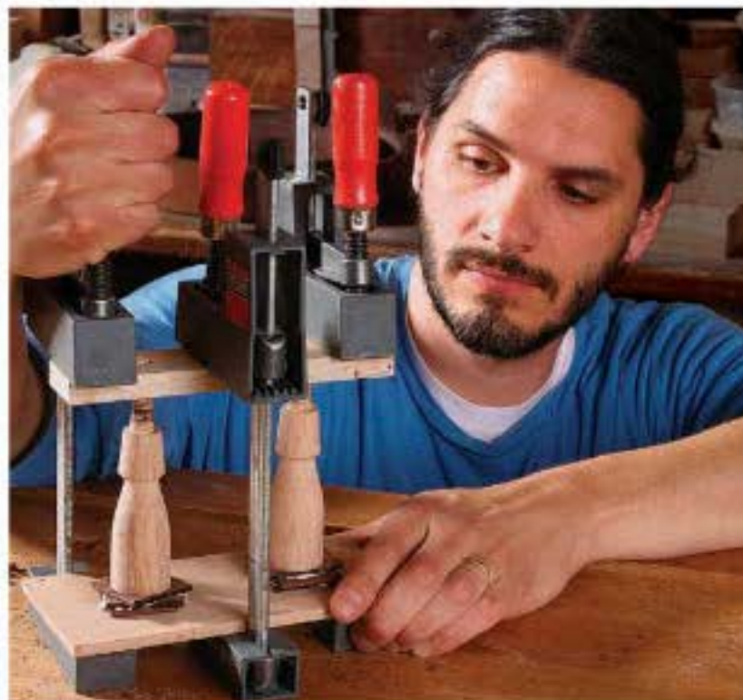
Clamp them tight. A simple caul allows Tetreault to apply even pressure on the washers, snugging them down onto the tenon for a tight, even fit.
