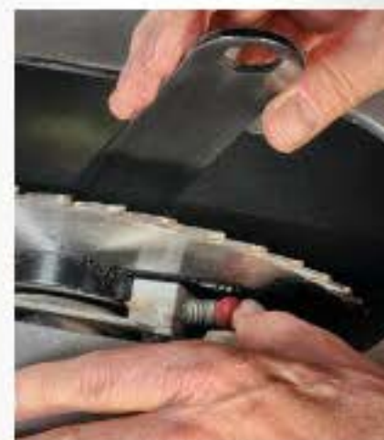
Single-wrench blade changes. Push in a plunger to lock the arbor, then loosen the arbor nut with the wrench.
