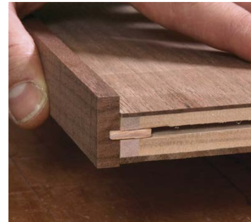
A little proud on the bottom. Raise the slot-cutter \frac{1}{32} in. before you groove the pencil roll to create a tiny reveal on the lower edge.
