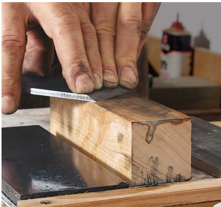
On your back. Using your normal sharpening action, alternate between stropping the bevel and the back.
