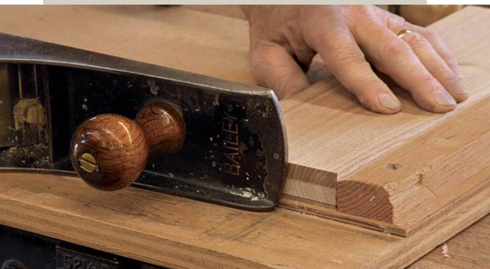
Square the ends. To make sure you don't build a twisted drawer, shoot the front ends of corresponding drawer sides, two at a time so they match. Re-label them if necessary.
