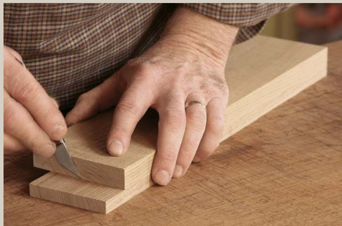
Match the back to the front. After ripping the back narrower (see p. 43), lay the drawer front on it, lining up the top edges. Then scribe the ends of the drawer back to match—both length and angle—and use the tablesaw and shooting board to trim them precisely.
