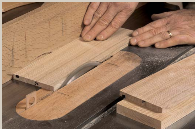
Trim the sides. Rip the drawer sides to the same width as the drawer front. Curry marks the end of each piece to keep track of its mating part and orientation.
