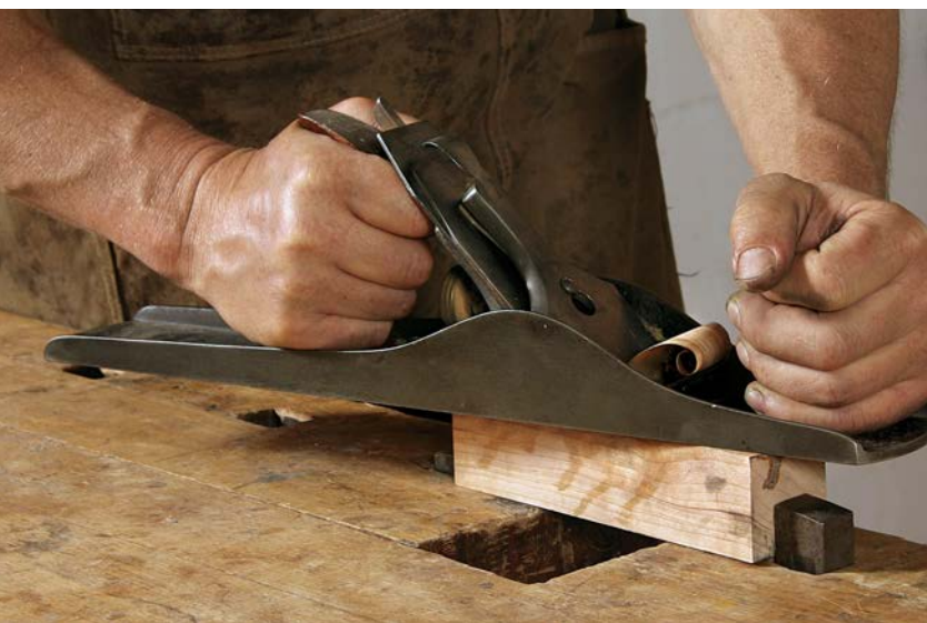
Make a flat strop. Plane the top of a hard-maple scrap to prepare the surface for use as a stropping block.
