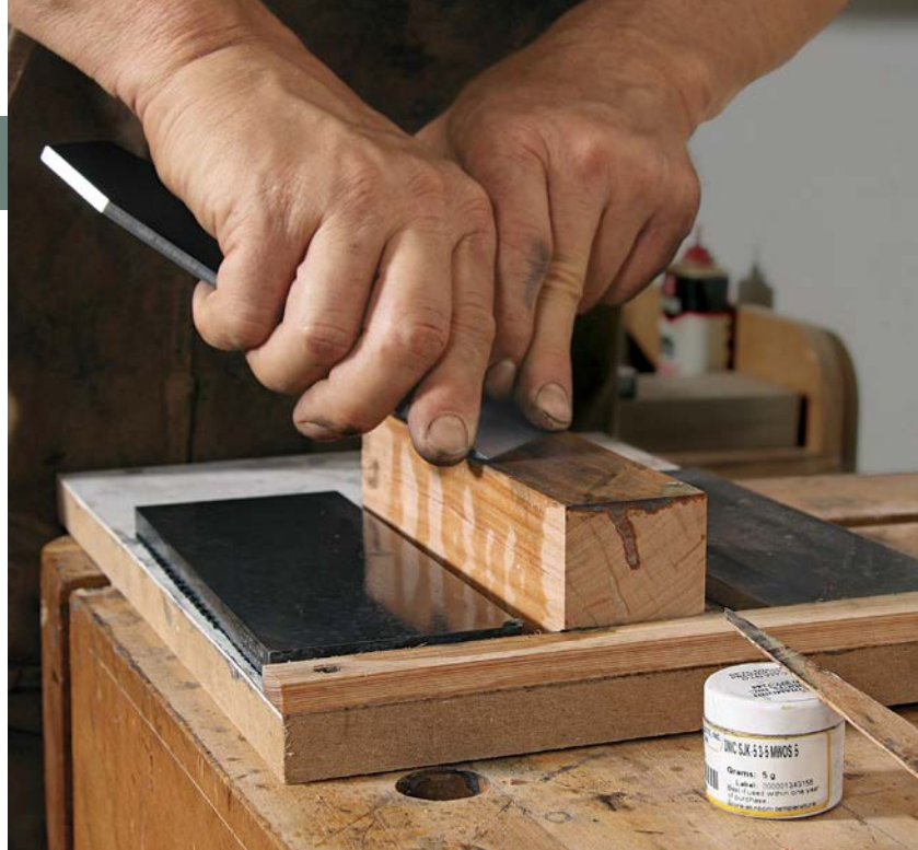
Final polish and deburring. To cap off his regimen, Boggs strops the blade with 4-micron diamond paste lubricated with oil. The diamond particles become slightly embedded in the wood, producing a finer abrasion.
