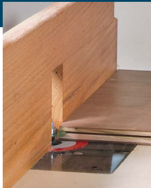
Get your groove on. Start by grooving all four edges of the top using a \frac{1}{8} -in. wide slot-cutter.
