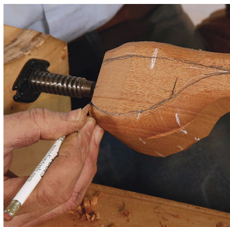
Draw the claws. After making a horizontal pencil line to mark the top of the ball, Breed defines the outlines of the claws.
