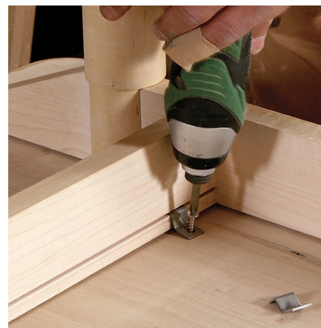
Clip it good. Metal clips hooked into the groove in the cross rails fasten the base to the tabletop.
