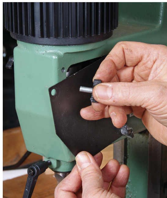
Thumbscrew is tedious. Having to completely remove a thumbscrew to gain access to the chuck, like on the General International 75-040, complicates bit changes.
