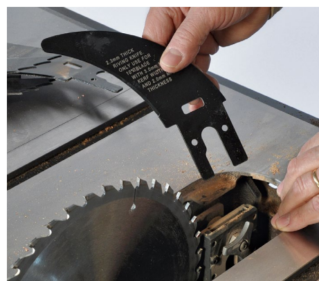
Quick-change riving knife. With the twist of a star knob, you can change from the blade guard to the riving knife in no time at all.
