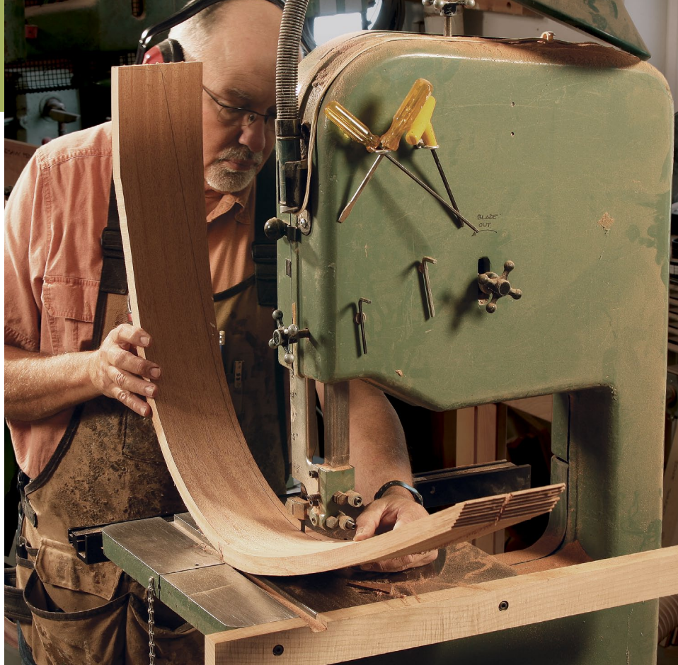
Curves on curves. The bandsaw is the perfect tool for cutting curved profiles on curved parts. Just make sure the workpiece is always touching the table in the area where the blade is cutting. Quick tip: A bit of side pressure on the back of the blade will help you control the path of the cut.
