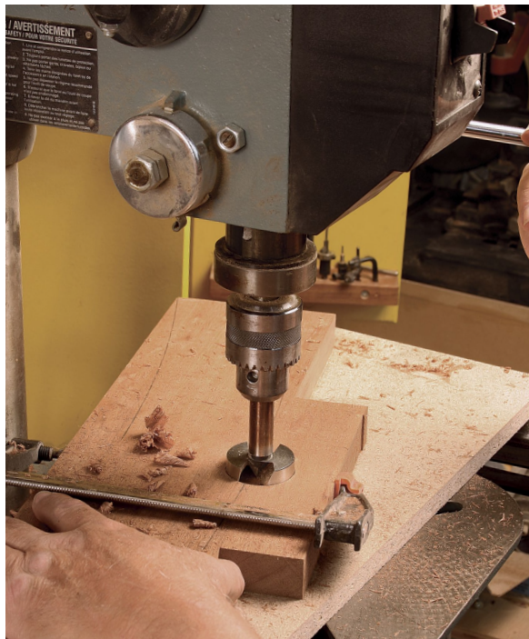
Decorative detail. Clamp on a scrap block and use a Forstner bit on the drill press to drill a clean hole through the edge of the workpiece (left). Then saw the curves to reveal the final look (bottom).
