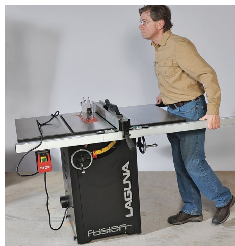
Unique mobility. Lift up on the fence rails like a pair of wheelbarrow handles, and the saw is ready to roll. The casters lock, so the saw doesn't move when in use.
