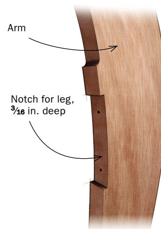
Arms need notches. The legs rest in a long, shallow notch on the inside edges of the arms. A simple router jig is the best way to make this shallow notch. Mark the notch on the arm and set it on a piece of softwood, at the location of the notch. Trace both edges of the arm (left), and cut along those lines. Throw out the middle section, glue coarse sandpaper to the curved edges, and clamp the arm flush between the pieces. Use a plunge router and straight bit to rout close to your layout lines, cutting into the jig as needed (bottom left). Finish up with chisel work.
