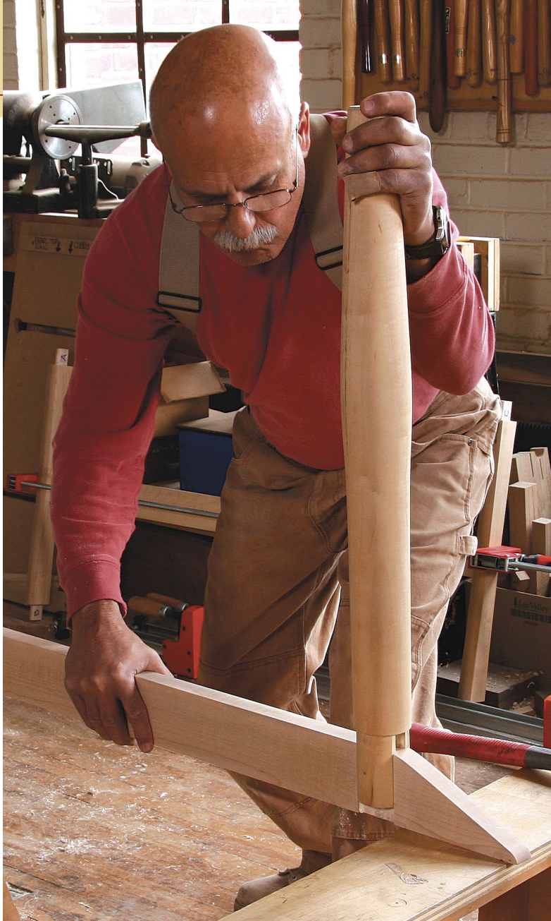
Assembling the undercarriage. With the H-stretcher already glued up and set aside to cure, Rodríguez assembles the bridle joints.
