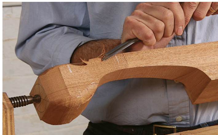
Incurve at the ankle. The rear claw has an inward curve that begins above its one knuckle. Create the curve with a #7-20mm gouge, making cuts from the bottom and top that meet in the middle. Alternatively, this curve can be shaped with a rasp or a spokeshave.
