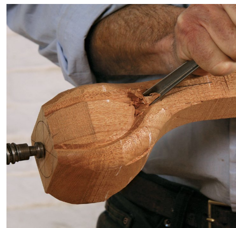
Claw carving. Cut in the claws with a #12-8mm V-gouge, working down to within \frac{1}{8} in. of the circle on the bottom of the foot, then back up the ankle. Use the same V-gouge (right) to establish the recess formed between the top of the ball and the crotch of the claws.
