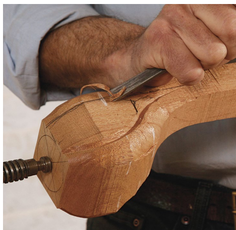
Claw carving. Cut in the claws with a #12-8mm V-gouge, working down to within \frac{1}{8} in. of the circle on the bottom of the foot, then back up the ankle. Use the same V-gouge (right) to establish the recess formed between the top of the ball and the crotch of the claws.
