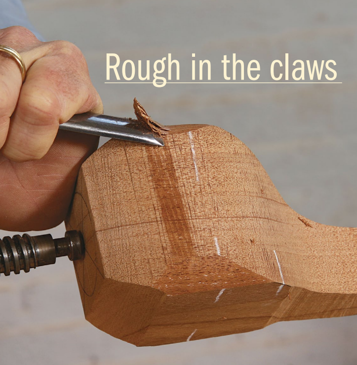
Chamfer and check. Using a #7-20mm gouge, knock off the corners of the foot until the gouge fits over them.
