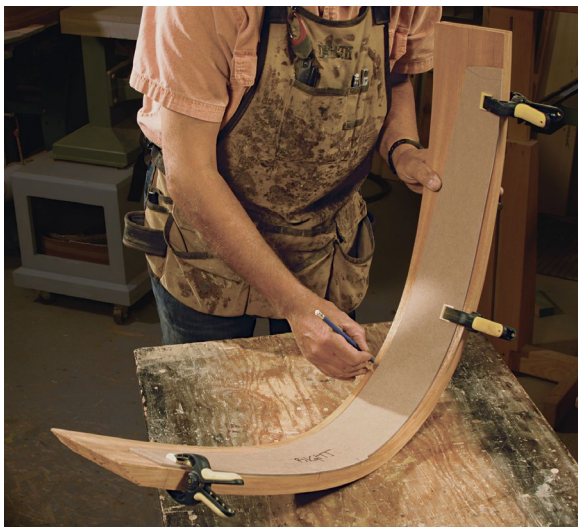
Simple tracing job. Use spring clamps to hold the pattern in place on the bent-laminated arms while you trace the edge profile.
