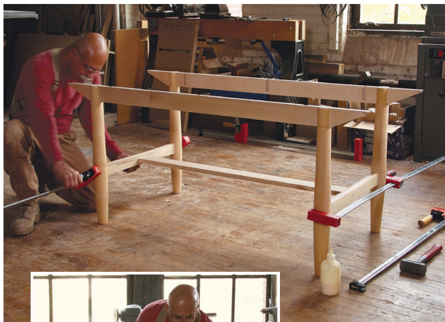
Connect the sides. Once the bridle joints are cured, glue the H-stretcher to the legs (above). Then complete the base by knocking in the dovetailed cross rails (left).
