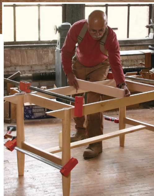
Connect the sides. Once the bridle joints are cured, glue the H-stretcher to the legs (above). Then complete the base by knocking in the dovetailed cross rails (left).
