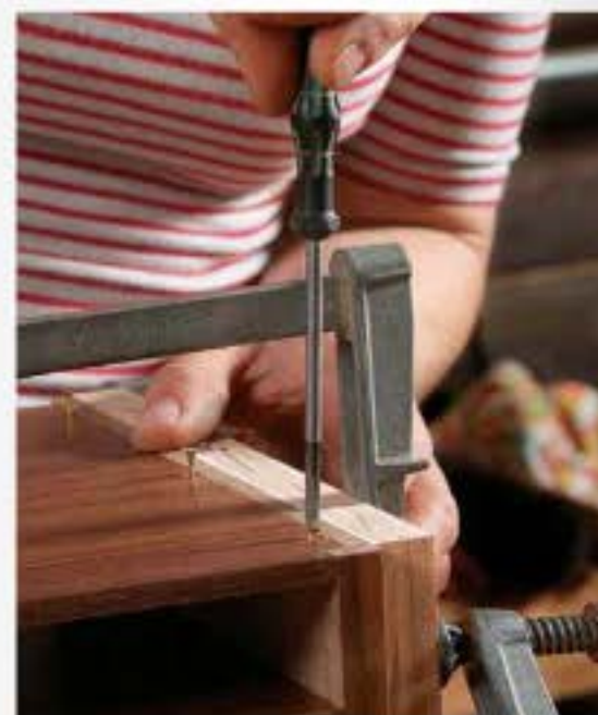
End blocks are next. These blocks frame the front of the drawer compartment and are joined to the uprights with dowels.
