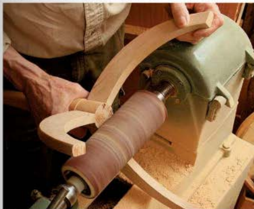
Joint cleanup. After the glue cures, smooth the bottom of the post with a drum sander.
