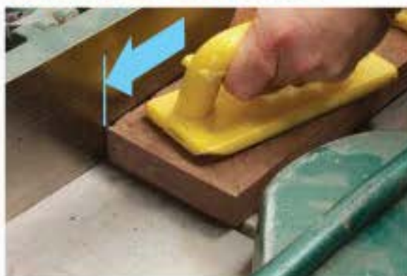
When boards go bump. Sometimes a bowed board will bump into the outfeed table and stall.
