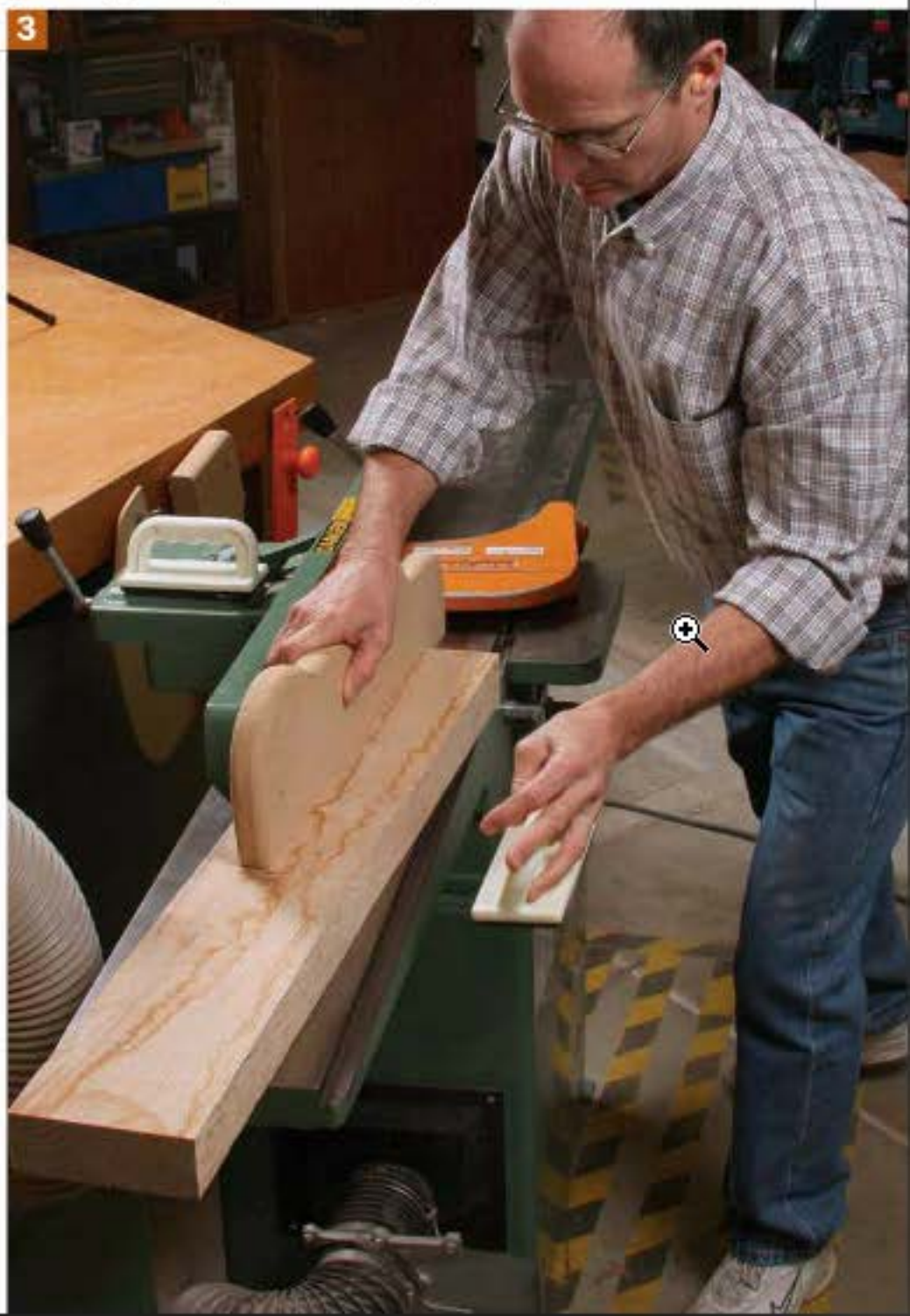
Push and walk. Adams generally starts with a push stick in his back hand for a good grip on the end of the board, and a push pad in the other for good downward pressure (1). On most boards you can keep your hands as they are, and just walk forward (2), finishing with the push stick alone (3).
