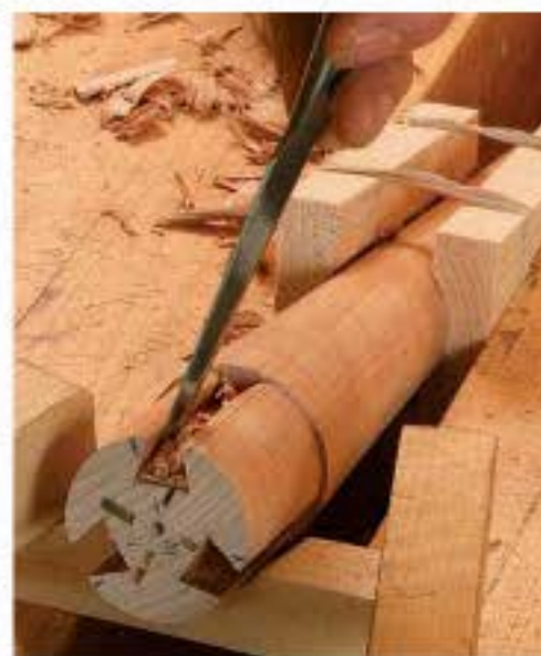
It's chisel work from here. Establish the shoulder of the socket with several mallet hits (far left), then remove long chips of waste, working from the end with the chisel horizontal. Extend the cheeks beyond the sawkerfs with vertical (left) and horizontal chops.
