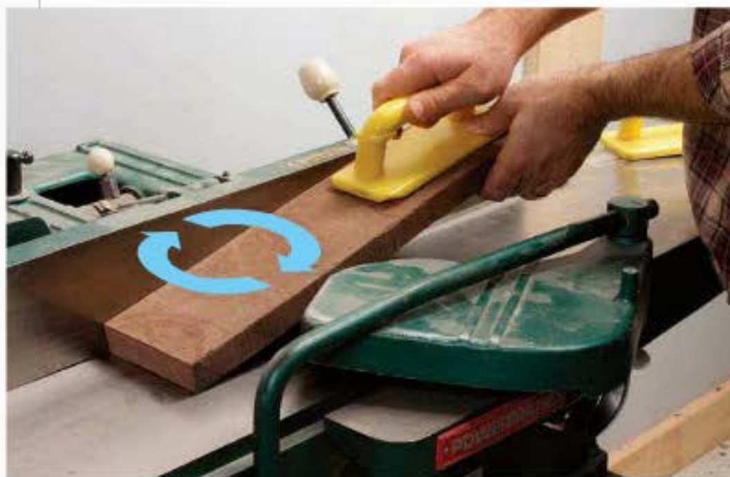
The flip trick. Now rotate the board end for end, set it halfway across the cutterhead, and lower it as shown. Push it forward to joint away the problem area. Now you should be able to turn the board right-way-round again and joint the entire face with no problems.
