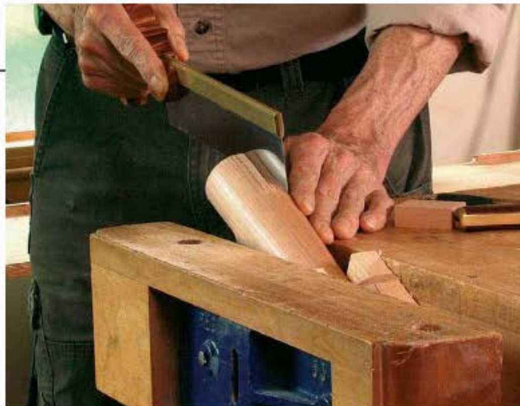
Saw the socket. With a rip dovetail saw, cut a kerf just inside the pencil lines and as deep as you can without hitting the shoulder.
