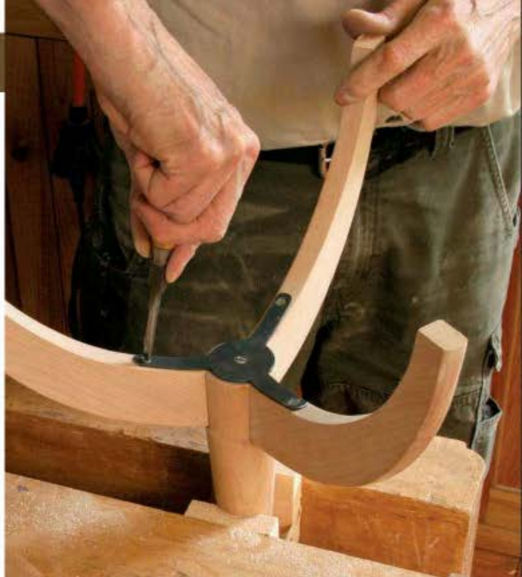
Bottom needs support. Screwing in a metal brace, or spider, reinforces the sliding dovetails. Becksvoort bought his spider and modified it, cutting several inches off each of its legs.
