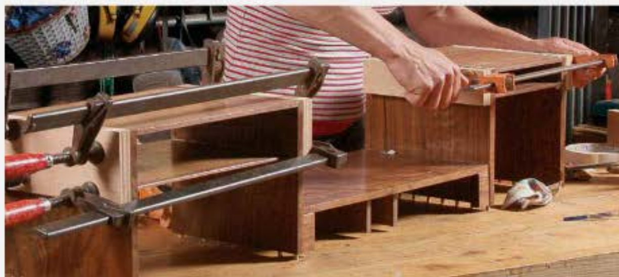
Glue up the side compartments. Clamp the assemblies together with shelves and bottoms in place (above). Secure the bottoms with screws (right). These strengthen the connection of bottom to sides, which would otherwise rely on the narrow glue surface of the stopped rabbet.
