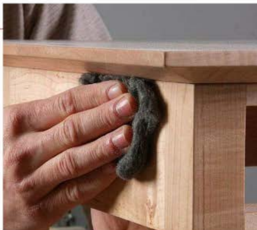
Rubdown before the topcoat. Rub down the surface with steel wool to level any remaining imperfections.
