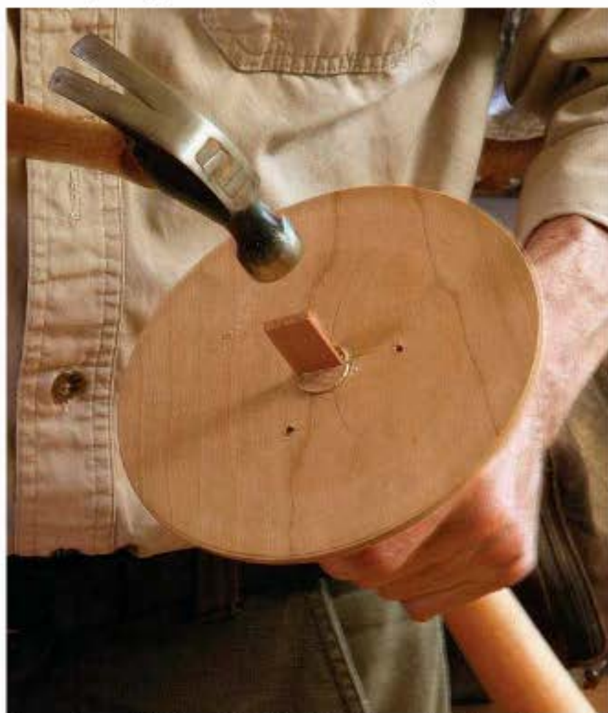
Crosswise wedge. To avoid splitting the subtop, orient the wedge perpendicular to the grain. After the glue cures, saw off the wedge and chisel the tenon flush. Then attach the top with screws through the subtop.
