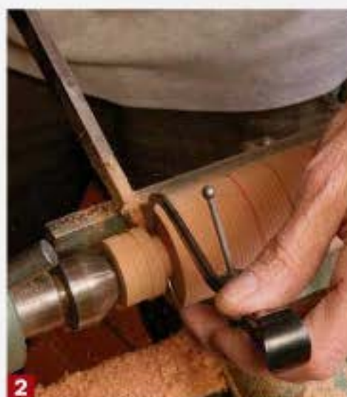
Marked and measured. After turning the cylinder, use a pencil to transfer diameter marks from a story stick (1). Then turn the tenon (2) and the bulb at the top of the post (3).
