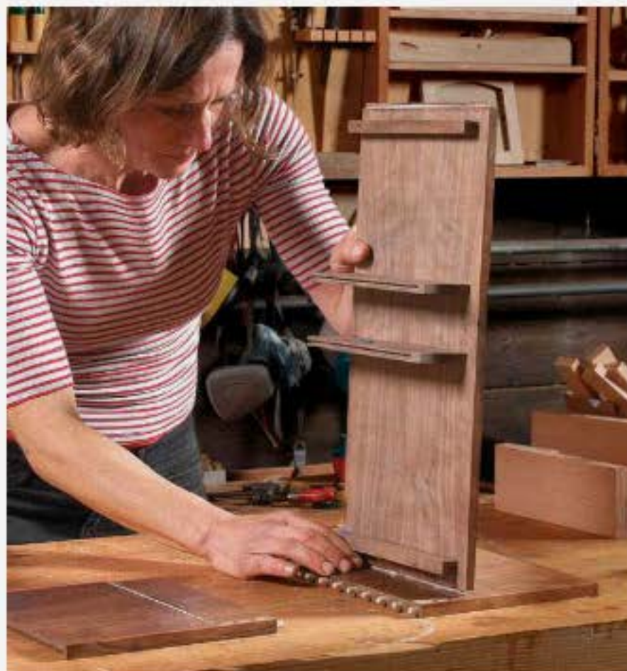
Work your way outward. Next, glue the uprights to the drawer compartment bottom.
