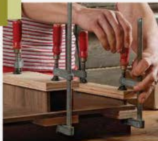
Start with the drawer compartment. Glue the guides to the bottom.
