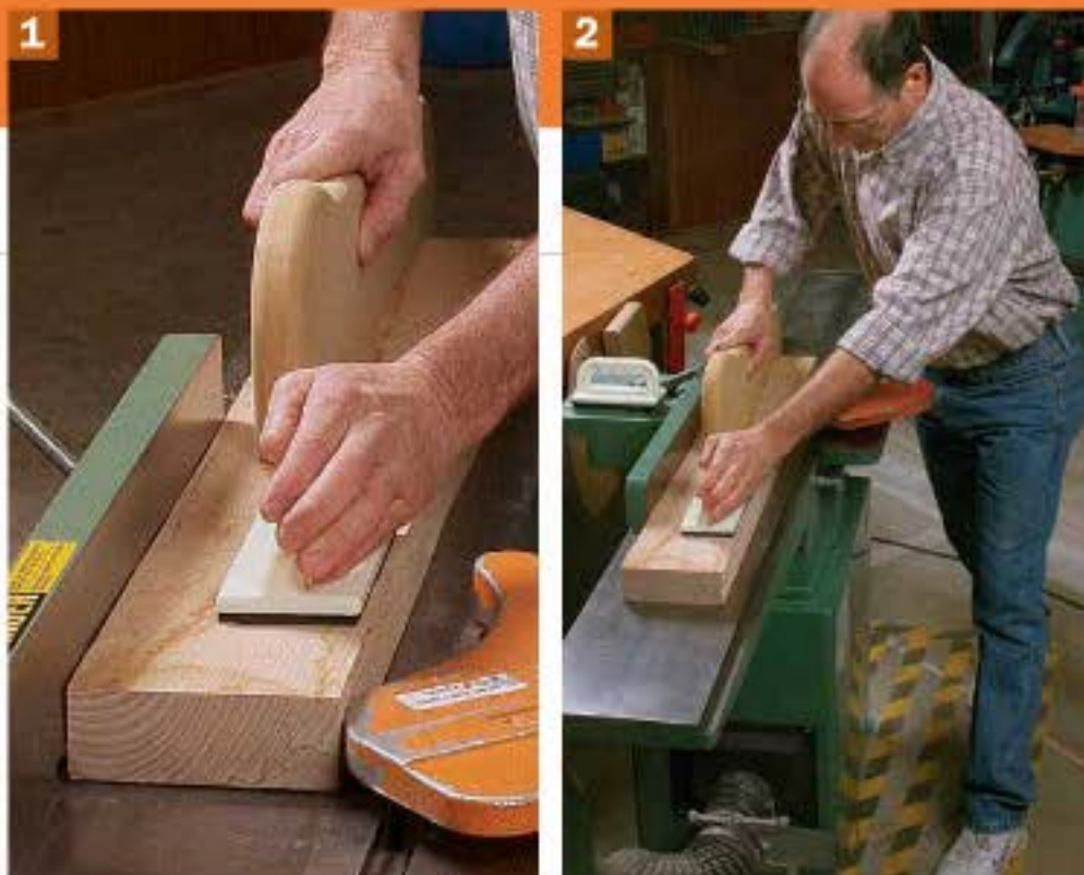
Push and walk. Adams generally starts with a push stick in his back hand for a good grip on the end of the board, and a push pad in the other for good downward pressure (1). On most boards you can keep your hands as they are, and just walk forward (2), finishing with the push stick alone (3).
