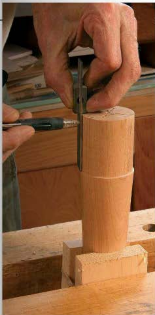
Extend the layout lines. Use a small square and a pencil to carry the scribed lines down to the shoulder.
