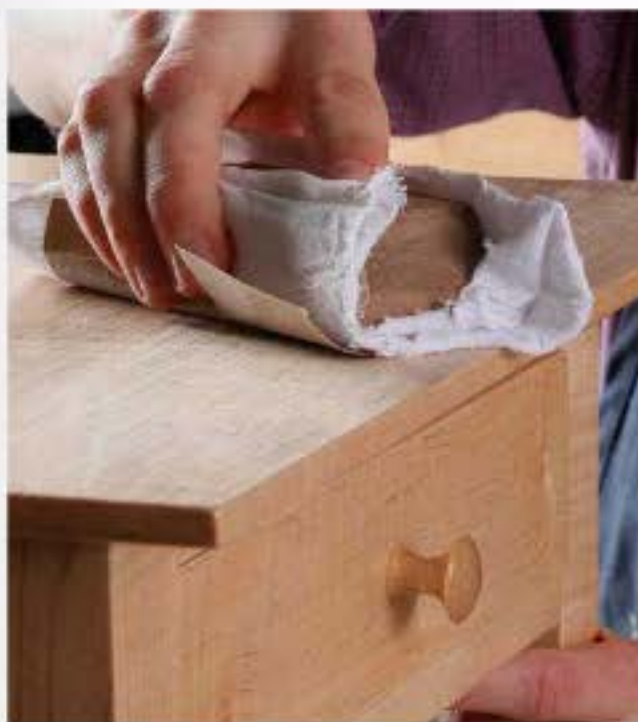
Rubdown before the topcoat. Rub down the surface with steel wool to level any remaining imperfections.
