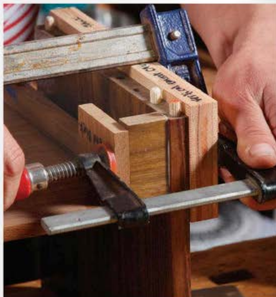
End blocks are next. These blocks frame the front of the drawer compartment and are joined to the uprights with dowels.
