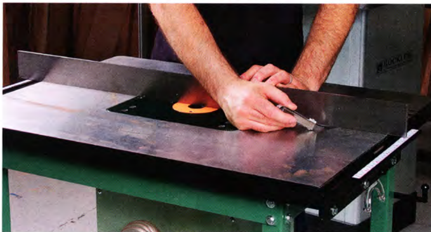
Perfectly flat is hard to find. Most of the tables had a dip, but the cast-iron tables had a slight crown. In practice, a crown is better than a dip.
