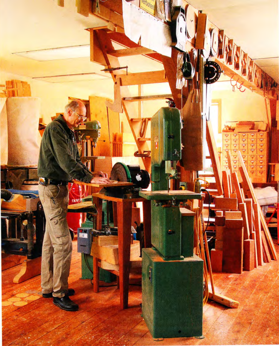
Little island at the support post. Becksvoort turned an obstruction into an asset by attaching power outlets to it, and clustering his bandsaw, jointer, and sander nearby. Related accessories hang on the post, too.
