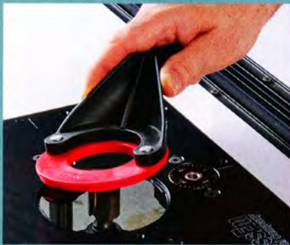
Twist and lock works well. Most of the lift plates use a spanner wrench to lock and unlock the insert ring. It's a fast and easy system.
