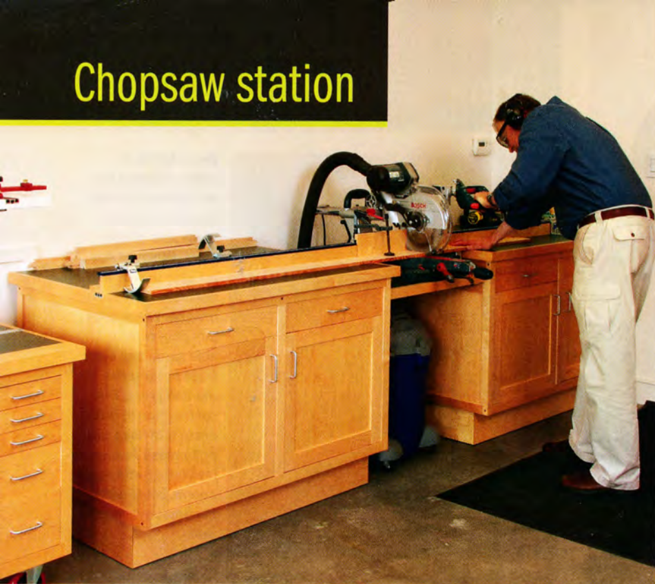
Support plus storage. A pair of cabinets with a lowered shelf between them provides a home for the chop saw. The fence system, which fastens in the T-track, can be quickly removed. O'Brien has French-fitted the drawers to hold some of his hand tools (see below).
