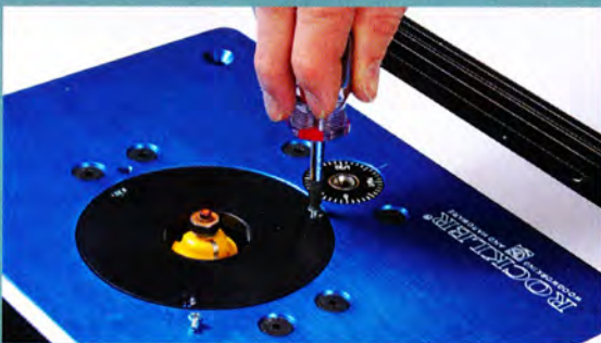
Twist and lock works well. Most of the lift plates use a spanner wrench to lock and unlock the insert ring. It's a fast and easy system.
