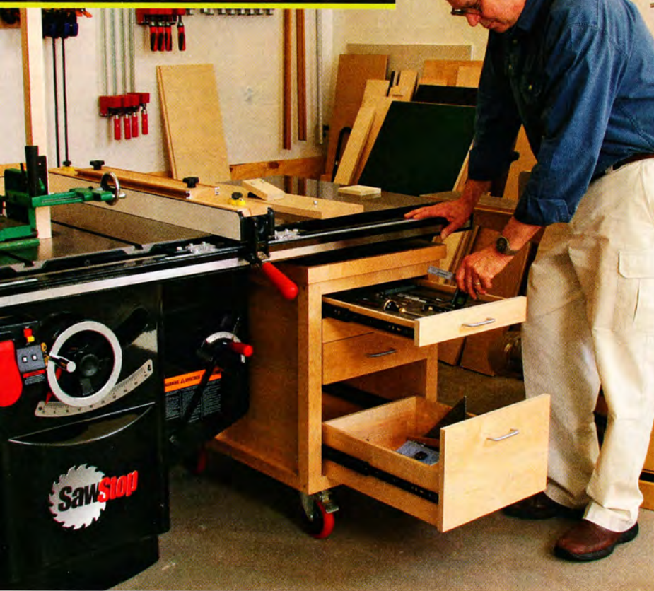
Saw supplies within reach. O'Brien's tablesaw cart, holding measuring tools, jigs, and saw accessories, slips beneath the side extension table.
