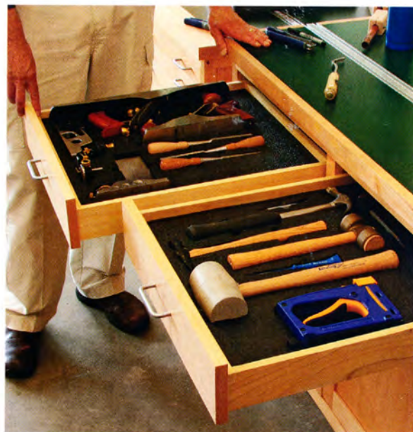
Support plus storage. A pair of cabinets with a lowered shelf between them provides a home for the chop saw. The fence system, which fastens in the T-track, can be quickly removed. O'Brien has French-fitted the drawers to hold some of his hand tools (see below).
