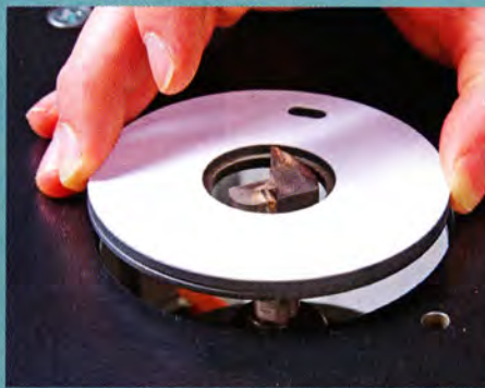
Snap-in rings are even easier. The insert rings for the Woodhaven EZ Lift have a rubber O-ring around them that keeps them in place. A screwdriver removes the ring.
