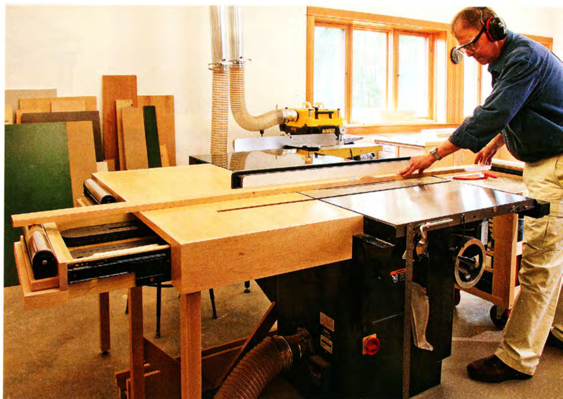
Saw supplies within reach. O'Brien's tablesaw cart, holding measuring tools, jigs, and saw accessories, slips beneath the side extension table.
