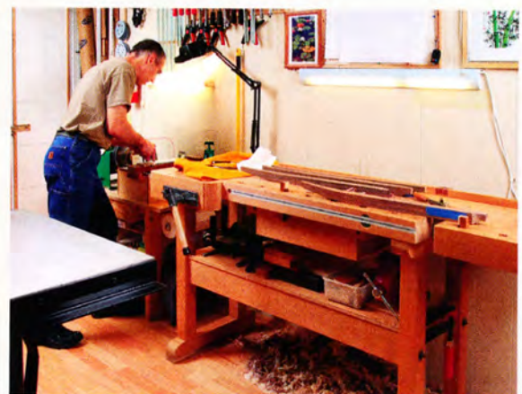
Flexible lighting. A desk lamp attaches to the left side of the workbench (above) for the sharpening station, and to the right for the small fold-down drafting table (below).
