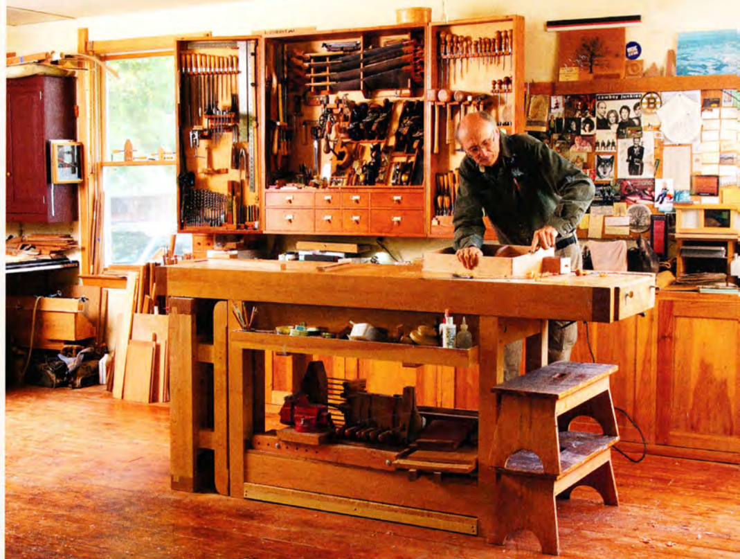
Hand tools within easy reach. One corner of Becksvoort's shop is dedicated to benchwork. His custom-height bench is located near his wall-mounted tool cabinet. And counter-height cabinets along the wall provide ample storage for handheld power tools.
