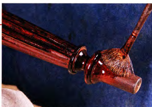
Every finisher needs a fan. The broom-like bristles of this brush are used to pounce and daub glaze into hard-to-reach areas.
