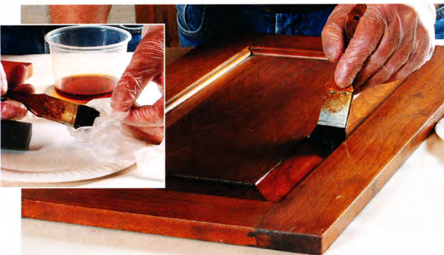
For small, flat surfaces. This brush is great for narrow, flat surfaces. Gedrys puts the brush inside a disposable glove (inset) to keep it from drying out between coats.
