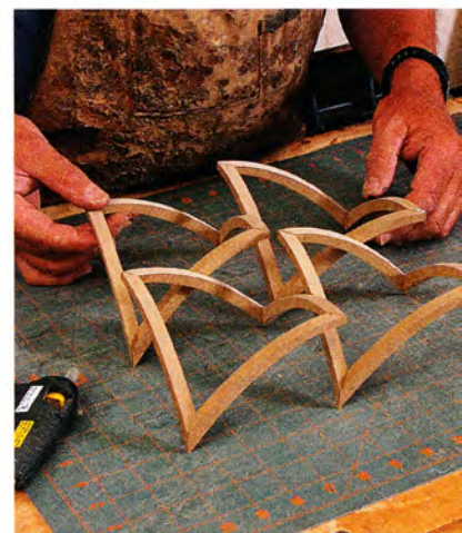
A little MDF goes a long way. Fortune cut short, curved pieces from a small scrap of \frac{1}{4} -in. MDF and hot-glued them together to make these models. He made extras and tried various groupings until he found the linked pairing he settled on.
