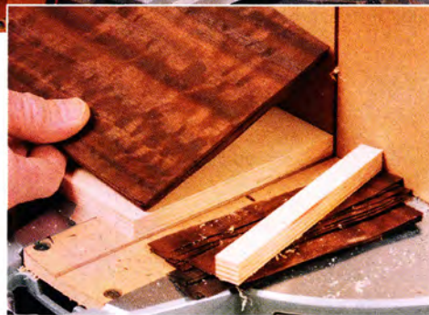
Trim veneers cleanly. Veneers (and plastics) will shatter on the miter saw, but if you hold them down with a sacrificial board (above), you can get a perfect cut on a whole stack (left).
