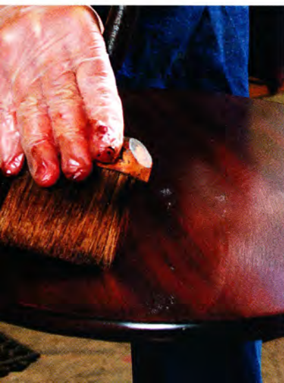
A brush for blending. The softener removes excess color and blends what remains. Wipe the excess glaze onto a paper towel dampened with solvent.
