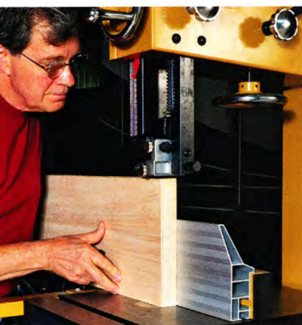
Big mouth. With 14 in. of resaw capacity and a 14½-in. throat, the PM1500 can handle big boards.
