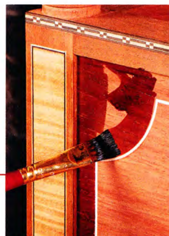
Flat and straight. The rectangular shape of this brush helps it follow a line—even a curved one—very accurately.
