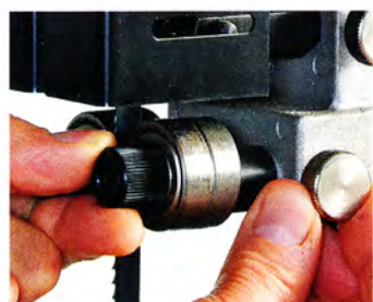
Tool-free. Guide adjustments are made without the need for tools, and they hold their settings.
