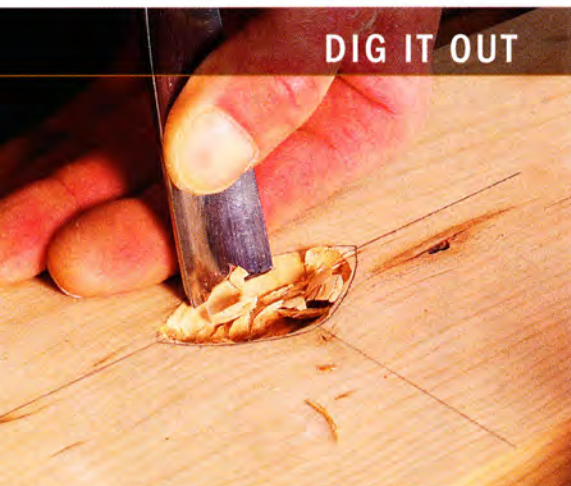
Work around the rim. Use a #8-20mm and #7-27mm gouge to rough in the perimeter. Work across the grain first (left), then with it (above).
