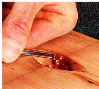
Get under. You need a smaller gouge to create the undercut at the top of the pull (left). Coleman uses a #8-4mm gouge there. In the middle (right), he uses a #8-10mm and a #5-10mm.
