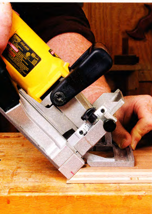
Two ways to slot a miter. The DeWalt fence doesn't adjust past 90°, so to biscuit a standing miter, you angle the fence to 45° and cut the slot with the workpiece clamped flat (left). But workpieces can shift, so O'Malley prefers to slot these parts while they're clamped in a vise (right). The material won't move, and there are no clamps to get in the way, but you need a fence that adjusts to 135°, like that on the Porter-Cable (shown at right).
