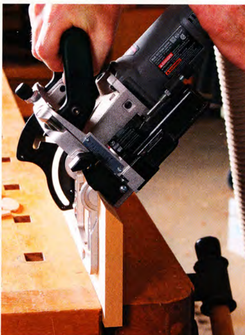
Two ways to slot a miter. The DeWalt fence doesn't adjust past 90°, so to biscuit a standing miter, you angle the fence to 45° and cut the slot with the workpiece clamped flat (left). But workpieces can shift, so O'Malley prefers to slot these parts while they're clamped in a vise (right). The material won't move, and there are no clamps to get in the way, but you need a fence that adjusts to 135°, like that on the Porter-Cable (shown at right).
