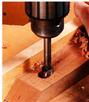
Drill slotted holes for screws. The screws attach the top to the base. Start with the counterbore, slightly overlapping three holes (left). Then drill the clearance hole the same way (right).
