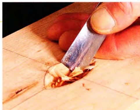
Work around the rim. Use a #8-20mm and #7-27mm gouge to rough in the perimeter. Work across the grain first (left), then with it (above).
