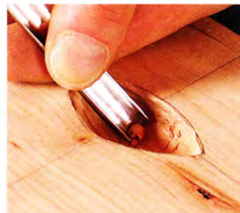
Get under. You need a smaller gouge to create the undercut at the top of the pull (left). Coleman uses a #8-4mm gouge there. In the middle (right), he uses a #8-10mm and a #5-10mm.
