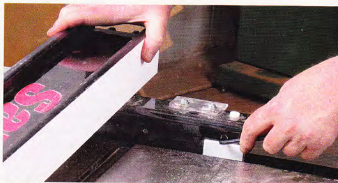
Rip fence is easy to correct. Use the adjustment screws to align the fence with a miter slot, and it should stay parallel in any position.
