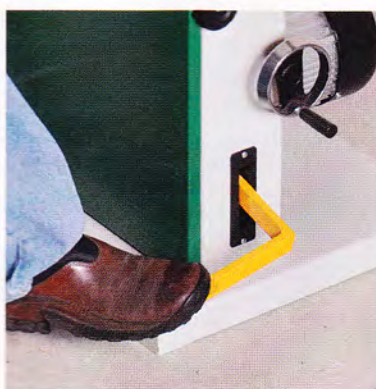
Quick stop. The foot brake is a welcome addition, and an uncommon feature on a 14-in. saw. It turns off the motor, too.
