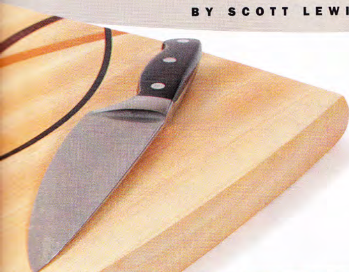
Thin strips make sweet curves. Lewis uses sandwiches of \frac{1}{8} -in.-thick strips to create the S-curved stripes that pass through the entire board.
