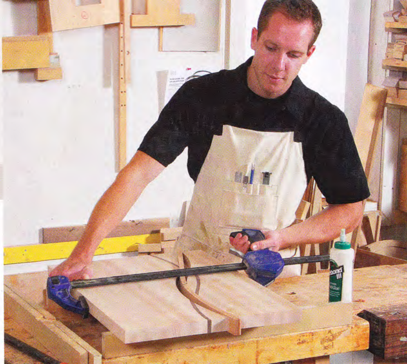
Thin strips make sweet curves. Lewis uses sandwiches of \frac{1}{8} -in.-thick strips to create the S-curved stripes that pass through the entire board.
