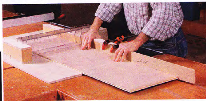
Set the stop. The long MDF auxiliary fence lets you set up a stop at the far end for cutting a series of workpieces to the same length.
