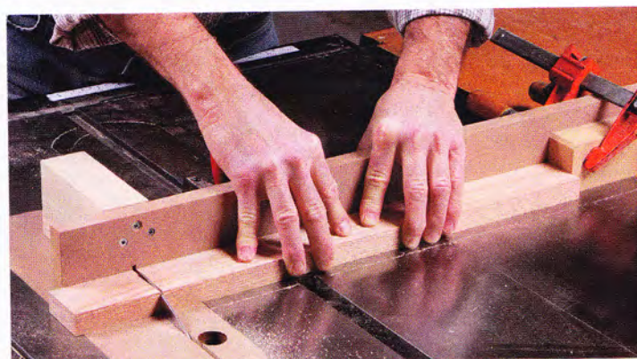
Set the stop. The long MDF auxiliary fence lets you set up a stop at the far end for cutting a series of workpieces to the same length.
