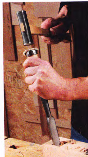
Precision paring. Japanese bench chisels are superb for paring, but shouldn't be used with a prying action, which could chip the very hard cutting edge.
