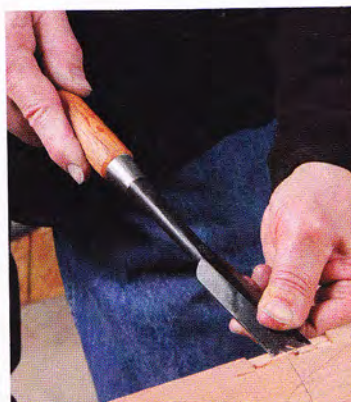
Specialty tools in action. The shinogi push chisel (above) excels at paring wide recesses like hinge mortises; the ultra heavy duty tataki (right) excels at hand-chopping large mortises.
