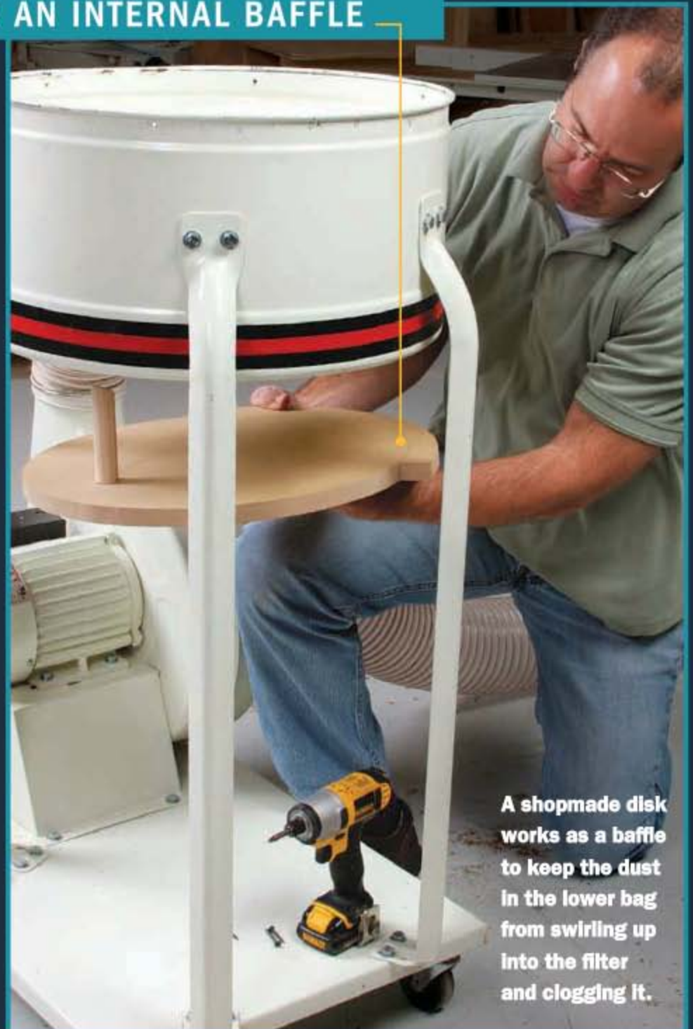
A separator stage grabs the vast majority of the dust before it reaches the dust collector, keeping even the finest filters clean and the suction strong.
