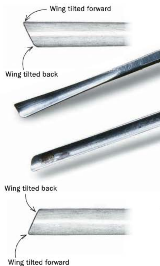
Mirror-image gouges. Each of these paired gouges will make an asymmetrical, crescent-shaped cut, deeper on one side than the other, like this one on the edge of a leaf.
