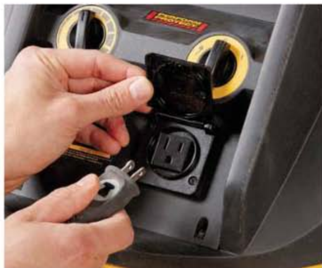
Plug and go. The power-tool actuation outlet turns on the vacuum when the plugged-in tool starts. To clear the hose, the vacuum runs for 15 seconds after the power tool is turned off.
