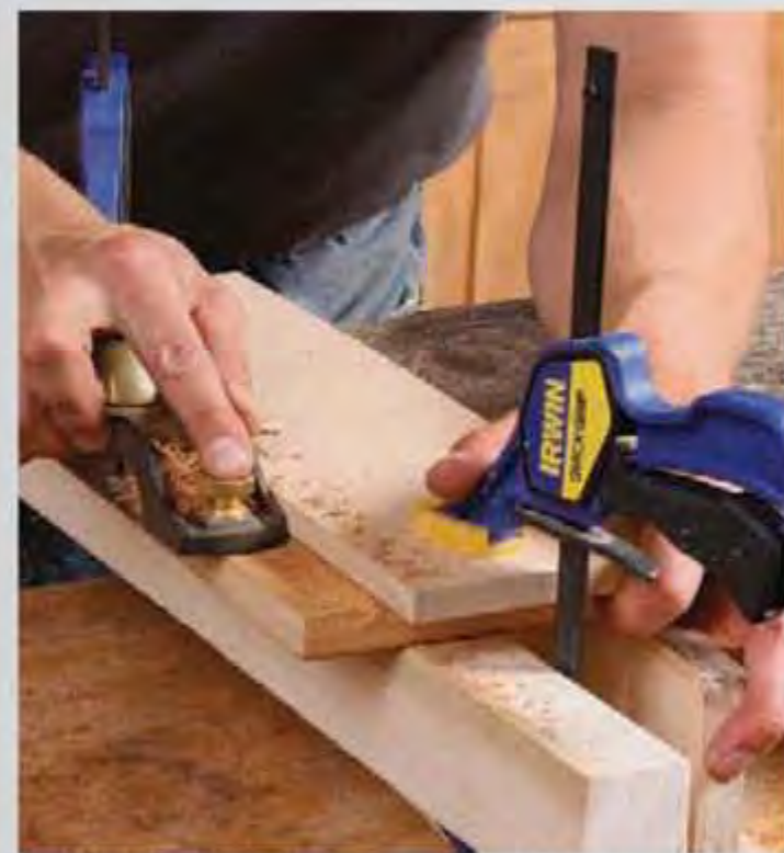
Rabbet the shelves to fit. The jointed bottoms of the shelves create a reference face for scribing perfectly even rabbets (left). Tetreault rabbets the shelf using a thick piece of wood to guide a rabbeting block plane (right).
