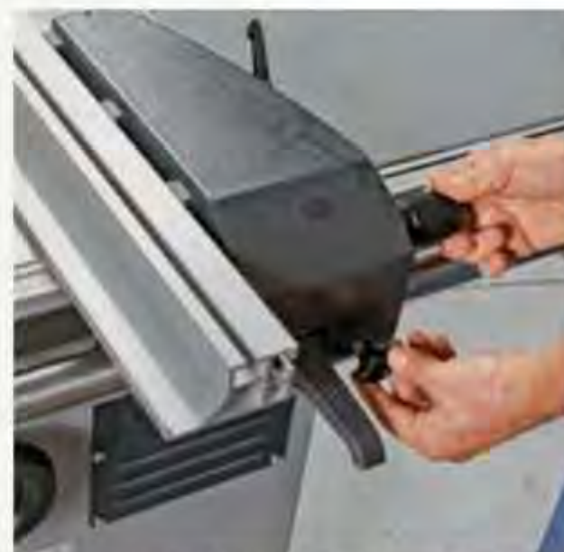
Micro-adjust rip fence. The Euro-style fence lets you dial in the cut with precision.
