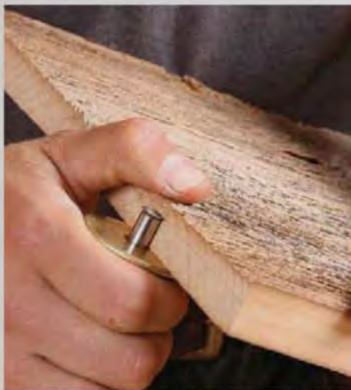
Rabbet the shelves to fit. The jointed bottoms of the shelves create a reference face for scribing perfectly even rabbets (left). Tetreault rabbets the shelf using a thick piece of wood to guide a rabbeting block plane (right).
