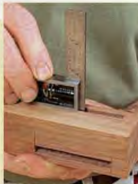
Find depths. Check the depth of a mortise by extending the rule all the way to the bottom.
