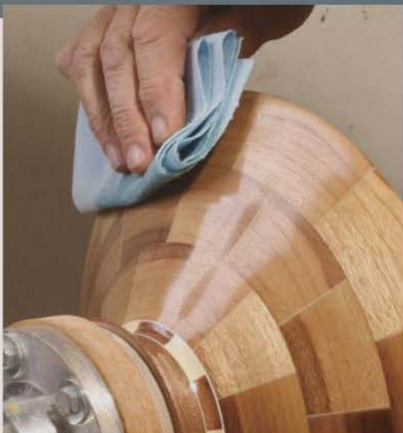
Keep it on the lathe. Sand and finish the top of the bowl, outside and in, while it is still spinning on the faceplate.
