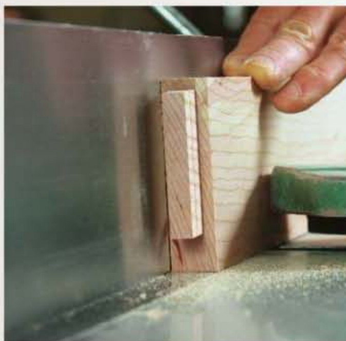
Flatten the apron tops. With the jointer fence at a 2° angle, trim the apron tops so they'll be flush against the tabletop.
