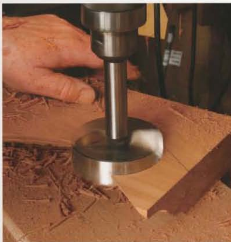
Period details. This traditional gooseneck molding gets a few more touches. Use the master template and a nail (above) to mark the location of the rosette at the top, and bore the hole using a Forstner bit whose diameter matches the rosette (right).
