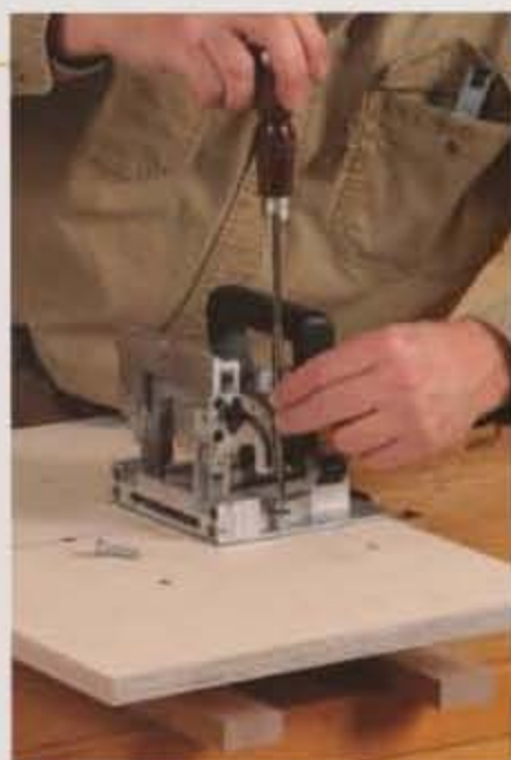
Bolt it down. Attached to a table, a biscuit joiner is easier to control and produces spot-on joinery.
