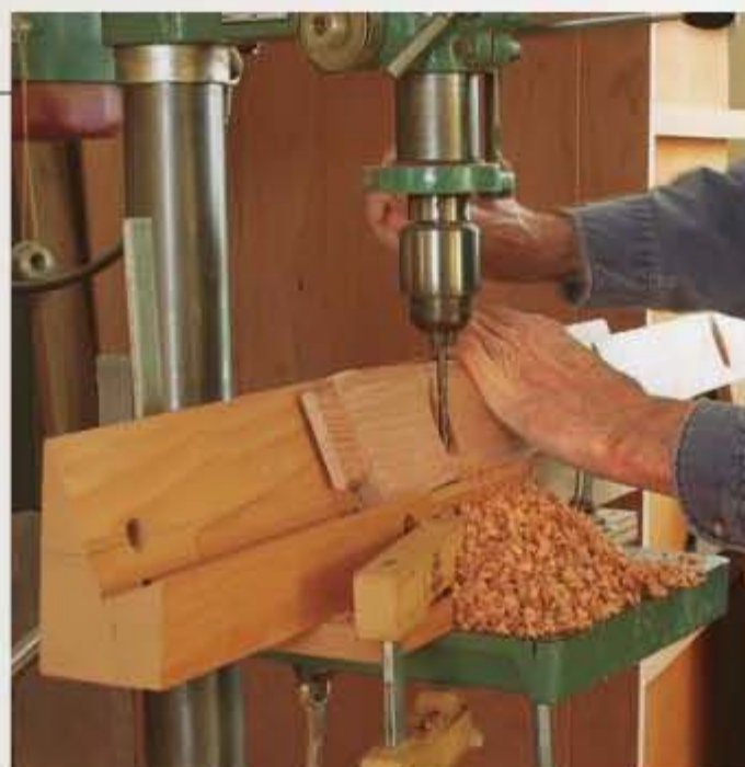
Pocket-hole jig for the drill press. A shop-built fence holds the inverted aprons at an angle to drill for the screws that will anchor the top to the base.
