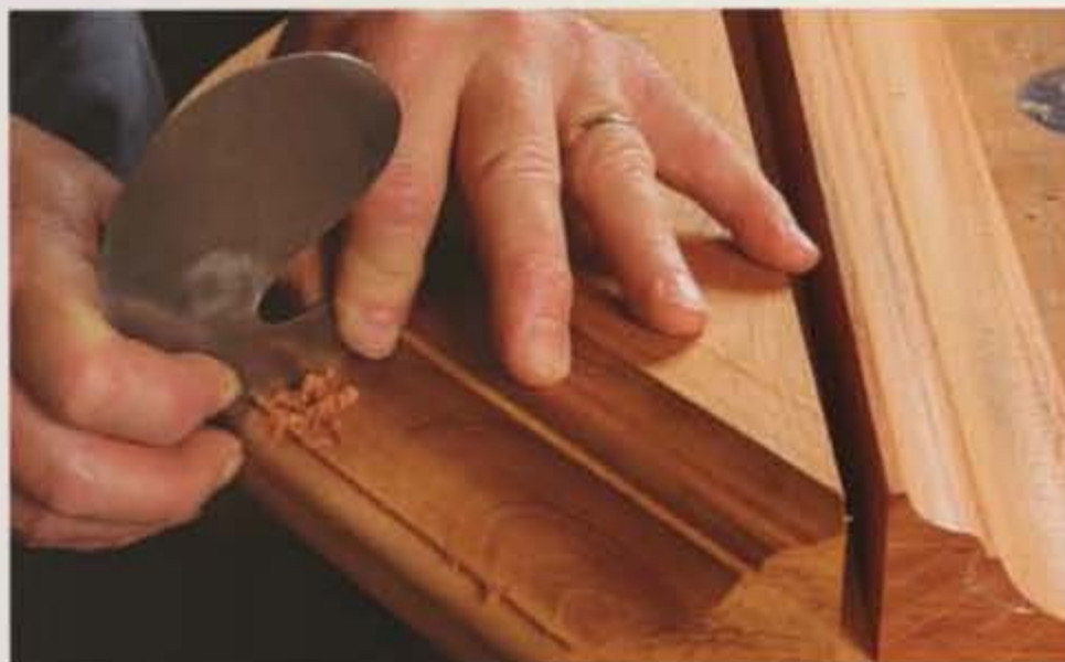
Blend and smooth with a scraper. A gooseneck scraper is ideal for cleaning up the different parts of the profile.
