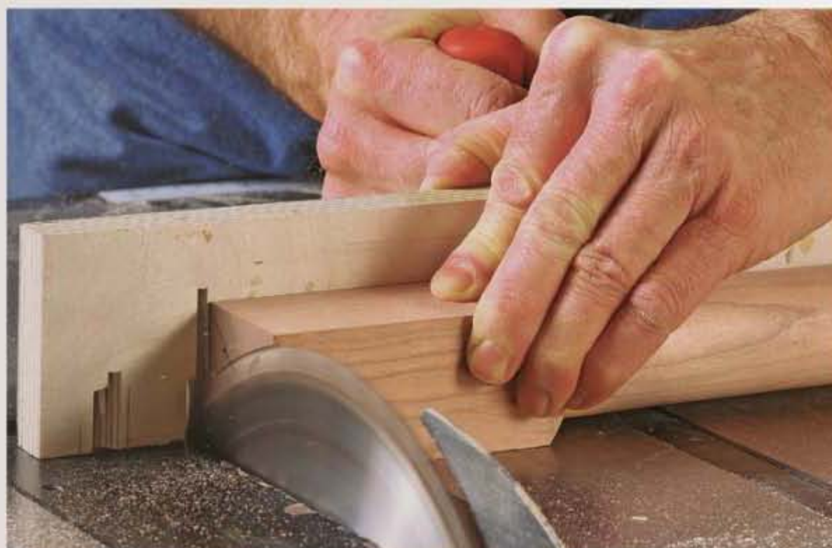
Two degrees of separation. With the highlighted corner at the bottom rear, a compound cut on the tablesaw removes a thin wedge of material.
