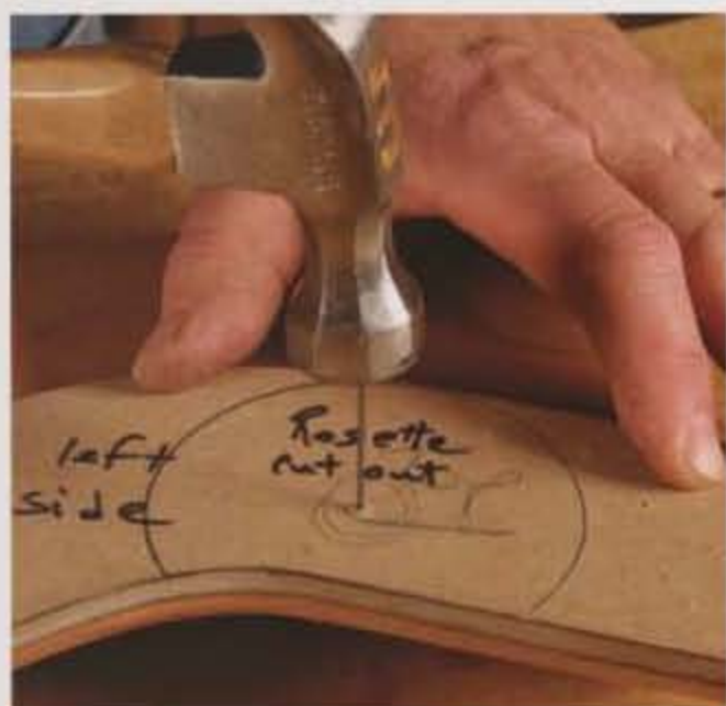
Period details. This traditional gooseneck molding gets a few more touches. Use the master template and a nail (above) to mark the location of the rosette at the top, and bore the hole using a Forstner bit whose diameter matches the rosette (right).
