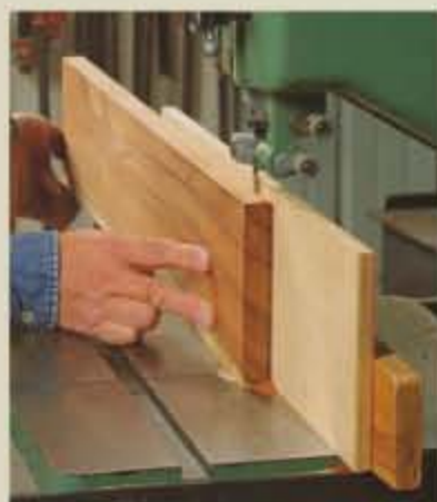
Perfect slices. The bandsaw resaws quickly and smoothly, with very little waste.
