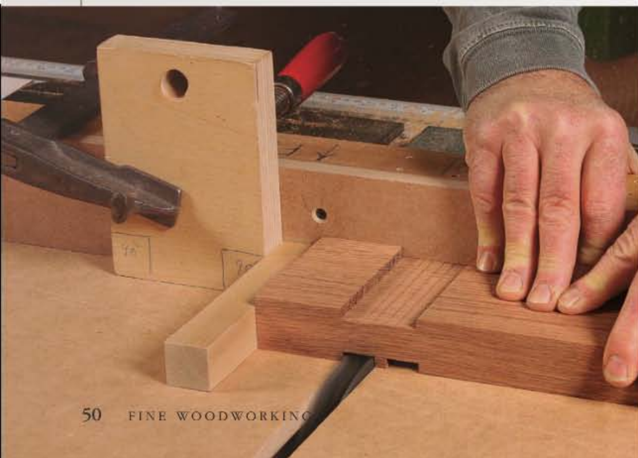
Spacer block for the other side. After you've made the first cuts on both sides of the rail, add the spacer to make the cuts at the other end of the dados. Then just nibble away the wood between them.
