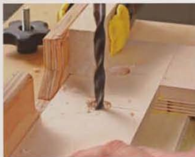
Drill and counterbore. Drill the larger holes in the fence first, to accommodate the heads of the carriage bolts, and then bore through-holes.
