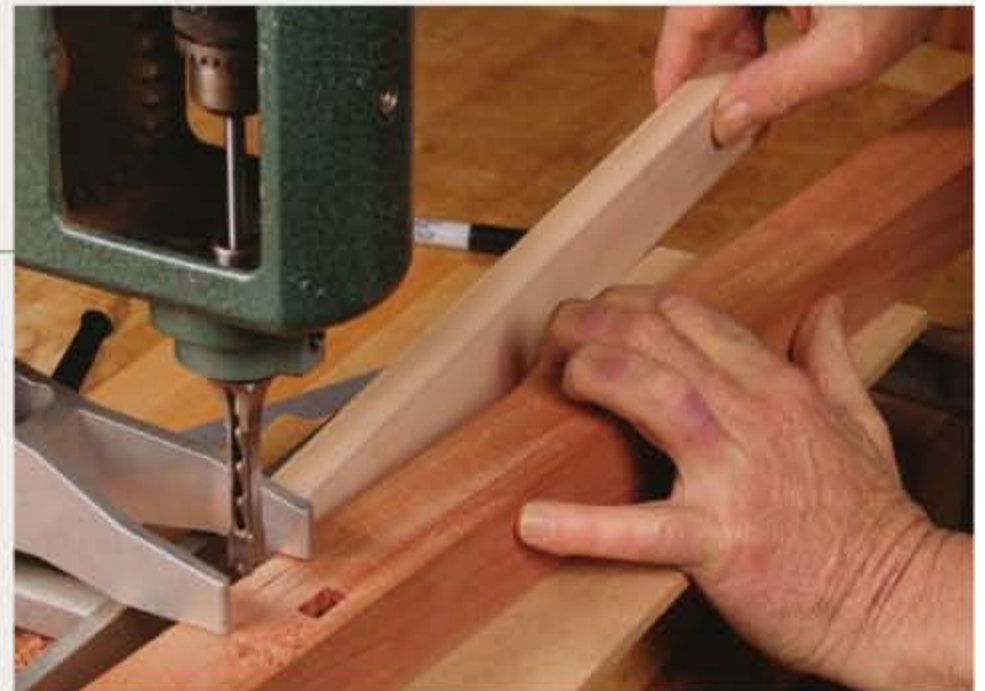
Add a second spacer and repeat. This spacer sets the distance between the mortises and is cut long to fully support the workpiece. Note that if the mortises are not precisely centered on the leg, you'll have to reverse the setup for the opposite leg.
