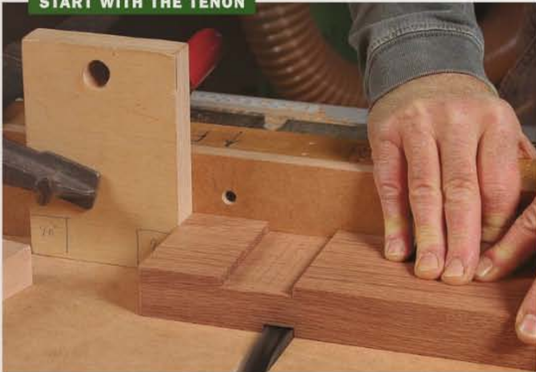
Stop block for one side. Cutting against the stop block defines the first wall of the two opposite dados.
