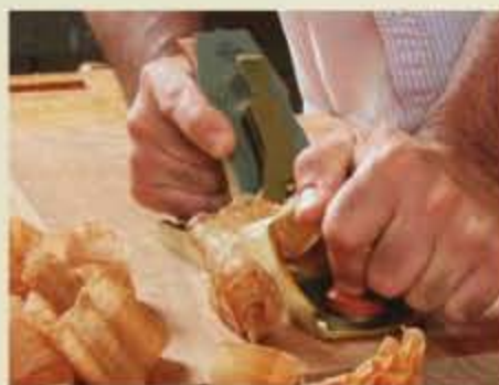
Surface prep. My No. 4 removes milling marks instantly, leaving behind a dead-flat surface.
