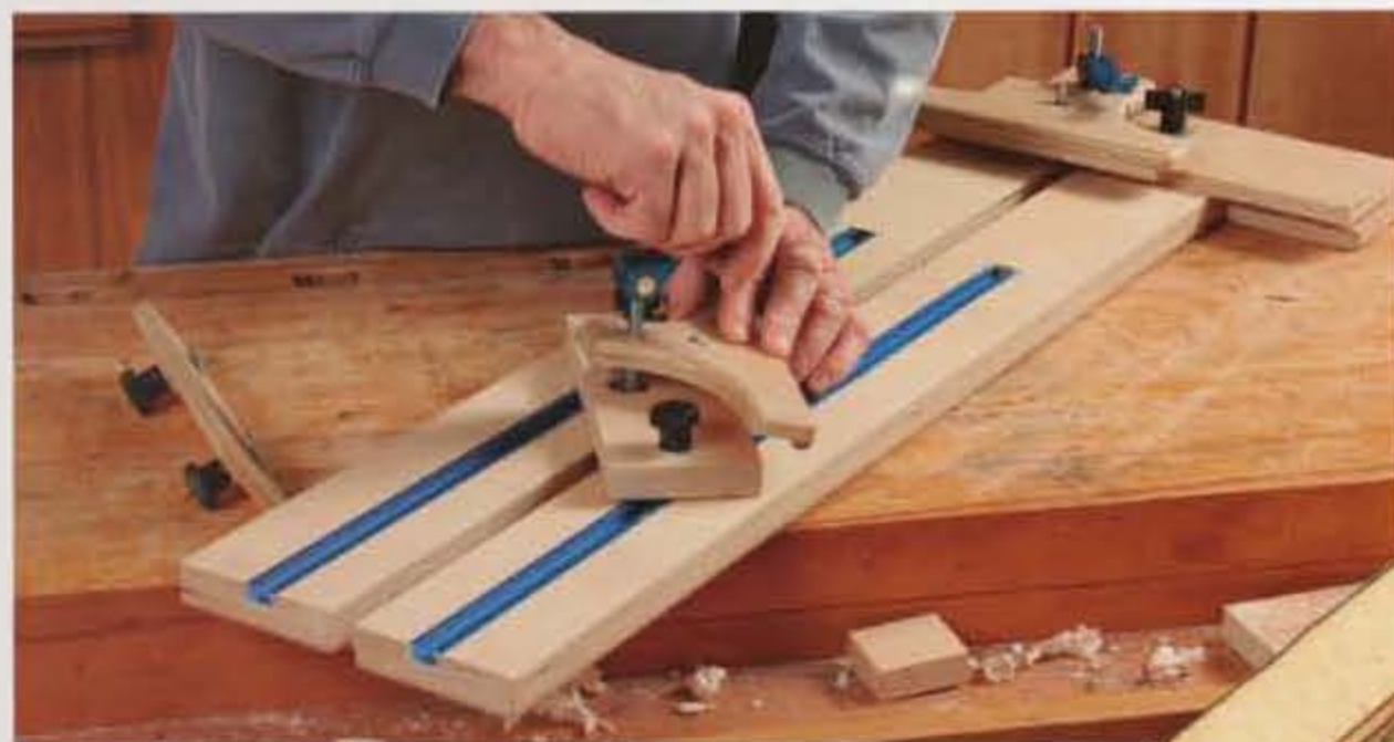
Assemble the clamps. They are a smart assembly of cam clamps, pins, bolts, knobs, and springs.
