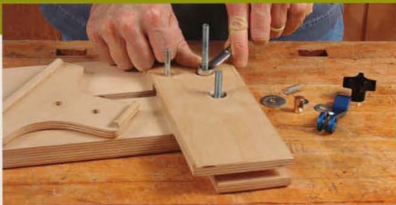
Attach the hardware. The bolts hold the cam hold-down for grasping the workpiece and the star knob that secures the adjustable rail.
