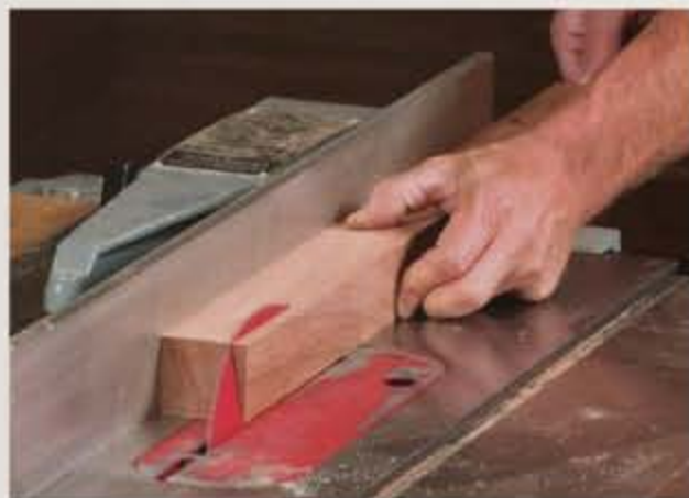
Trapped workpiece. With the blade tilted toward the fence, the workpiece can jam and shoot backward if allowed to lift slightly.
