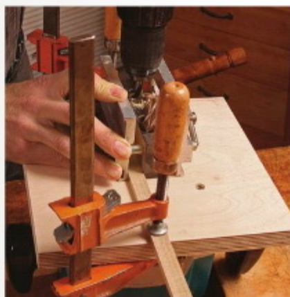
Rotate the jig. After drilling the first hole, spin the jig 180^\circ to locate the opposite hole.
