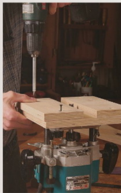
Smaller flush-trimming base. This square base is great for flush-trimming tenons and pegs. It offers support for the router on both sides of the bit.
