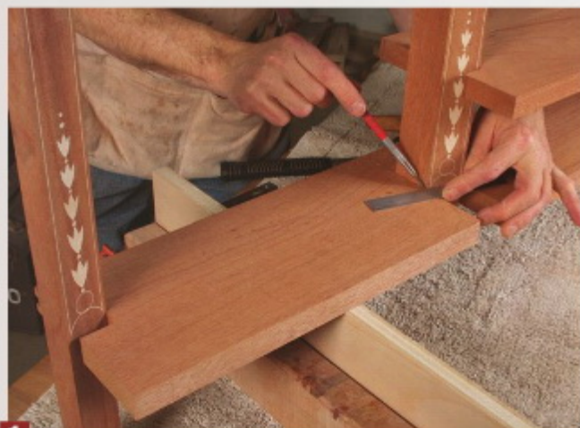
1 Where leg meets curve. With the front of the sideboard dry-fit, lay a straightedge across the front of each leg and mark where it meets the rails and the dividers.
