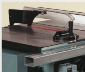
U.S. safety mandate. The UL issues a mandate (UL 987) on safety gear, adding anti-kickback pawls to the traditional gear—not much of an improvement.
