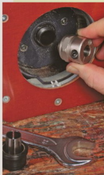
Easy replacement. The Musclechuck threads right in to the router's existing chuck.
