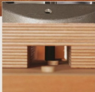
Sure-footed. The base straddles a series of screw-hole plugs, for example, with the twin support rails preventing the bit from tipping into the work surface.
