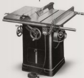
Unisaw sets the standard for American saws. Introduced in 1939, the Delta Unisaw features a blade guard and splitter by 1949, as shown in this catalog image.
