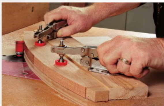
One size fits all. Bessey toggle clamps can hold workpieces of any thickness within their capacity without fussy adjustments of the clamp head.
