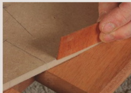
1 Where leg meets curve. With the front of the sideboard dry-fit, lay a straightedge across the front of each leg and mark where it meets the rails and the dividers.
