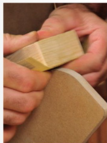
Final prep. Use a sanding block to clean up the edges and shape the templates as perfectly as possible. Defects in the template will transfer to the workpieces during routing.
