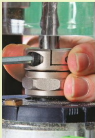
Quick-change bits. Paolini was able to install and remove bits in 7 seconds with an Allen wrench.
