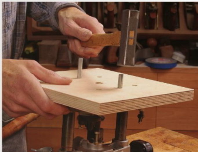
Pins center the router. Add some glue, drive in two \frac{3}{4} -in. dowels or metal pins, and the jig is done.
