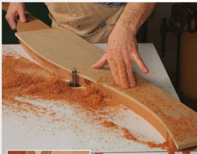
3 Shape the top rail. Attach the template to the bandsawn top rail and trim it flush (above), stopping just over halfway to flip the workpiece and reattach the template to rout the rest of the profile. Then dry-fit the legs and check that the upper rail is set back just enough to leave the veneer slightly proud of the leg (left).
