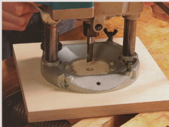
First, plunge through a square base. Put a \frac{1}{2} -in., plunge-cutting bit in the collet, and plunge down through the base.
