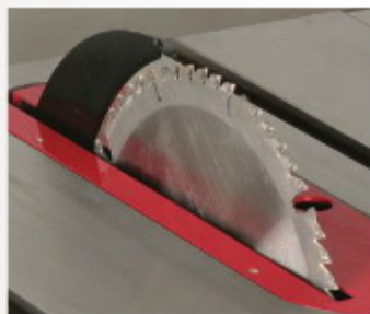
Riving knives required in Europe. Common on European saws for decades, this effective anti-kickback device was not adopted by U.S. manufacturers.
