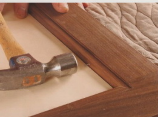
The trouble with miters. Mitered glass stops look great and go in just fine, but they are difficult to pull out later.
