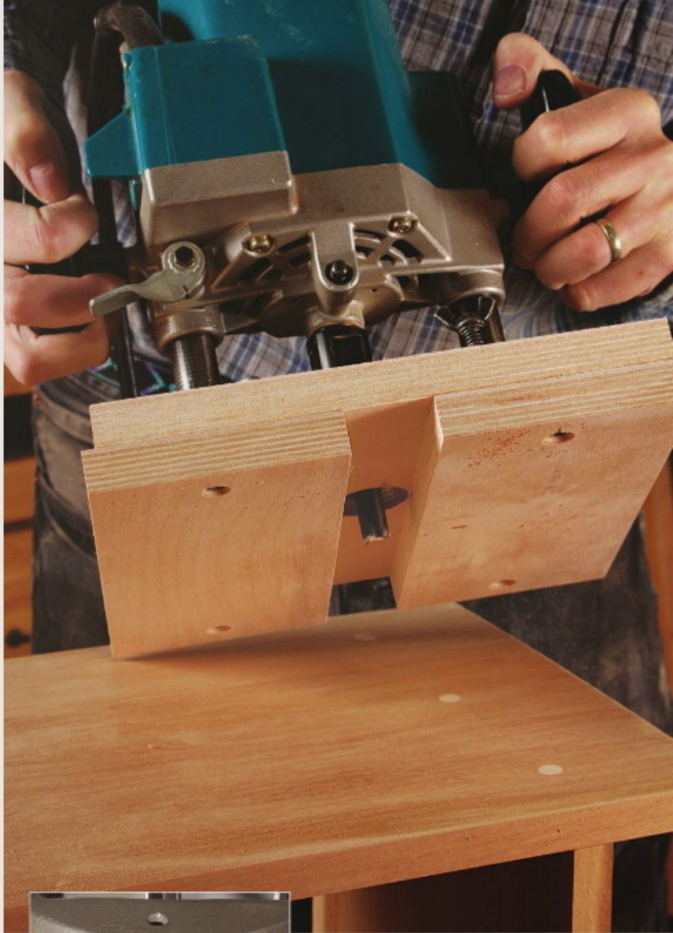
Smaller flush-trimming base. This square base is great for flush-trimming tenons and pegs. It offers support for the router on both sides of the bit.
