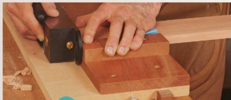
Clean up the bottom edge. This is your reference edge, so you don't want to touch it again.
