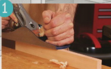
Clean up the bottom edge. This is your reference edge, so you don't want to touch it again.
