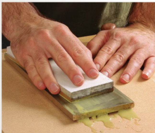
Bigger is better. A large diamond plate works the entire surface of the stone at once, so it's sure to be dead flat.
