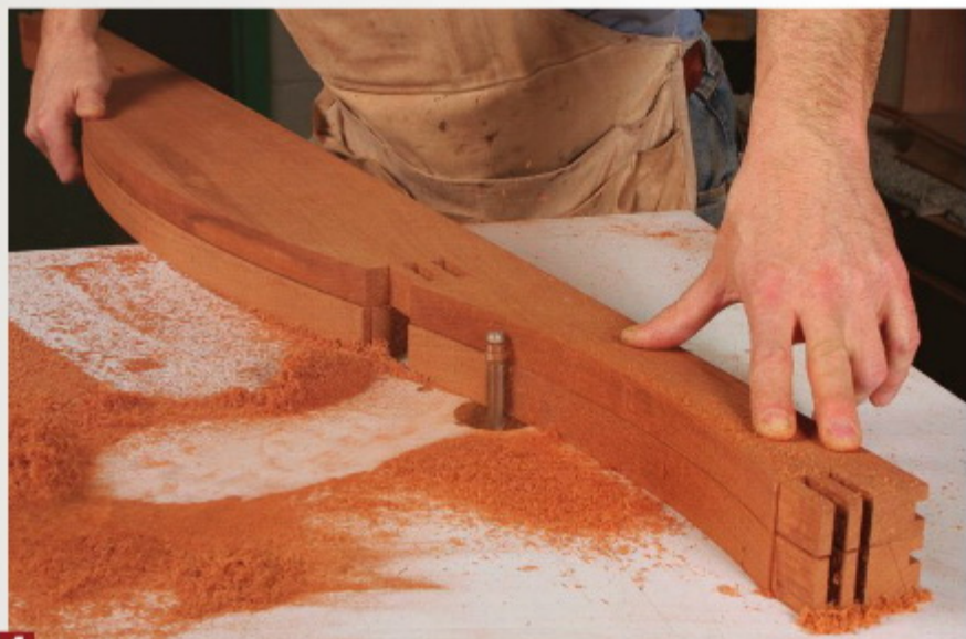
4 The rail becomes the template. Use the top rail to shape the lower rail and then the two drawer dividers to give all four pieces the same profile.
