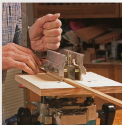
Register the jig on a straight strip. Clamp the strip in place and align the jig with it before marking and drilling the first hole.
