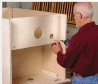
Add aprons for stiffness. Screw through the face into the cleats. On the cyclone end, pre-drill holes for the vacuum hose and power cords with a circle cutter.
