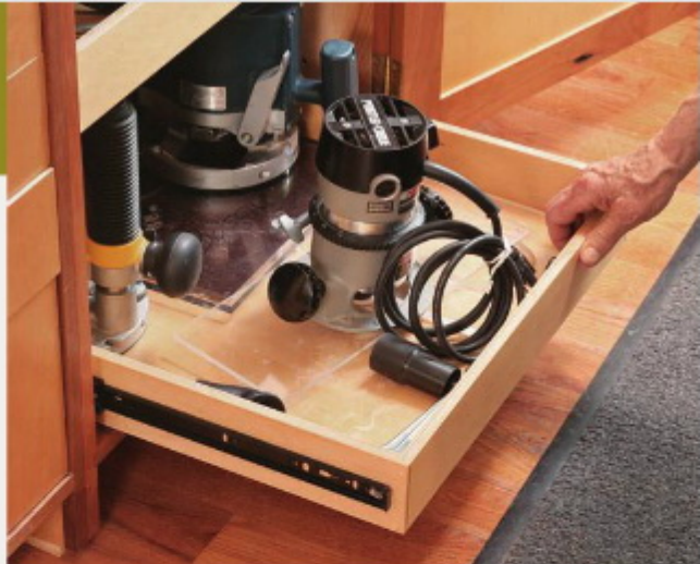
Behind the doors, more drawers. Shallow trays on heavy-duty drawer slides provide easy access to handheld power tools and other bulky items.
