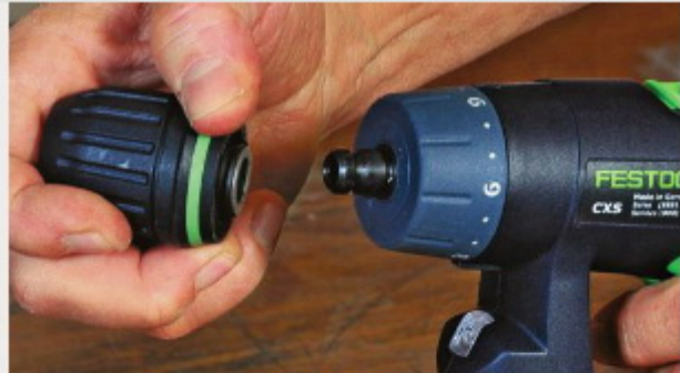
Quick-change chucks. Festool's FastFix system lets users change out chucks in seconds, without tools.
