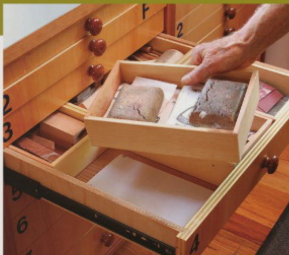
Behind the doors, more drawers. Shallow trays on heavy-duty drawer slides provide easy access to handheld power tools and other bulky items.
