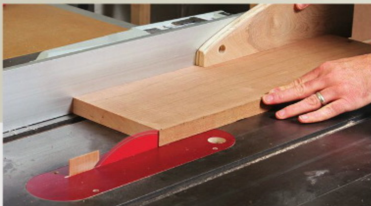
A shopmade splitter is the next best thing. It can't move with the blade, but it works for the majority of cuts, which are made with the blade at 90°.
