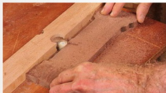
Rout halfway, then flip. There is no stop on the outfeed side, so don't risk getting too close to the foot on the trailing end.
