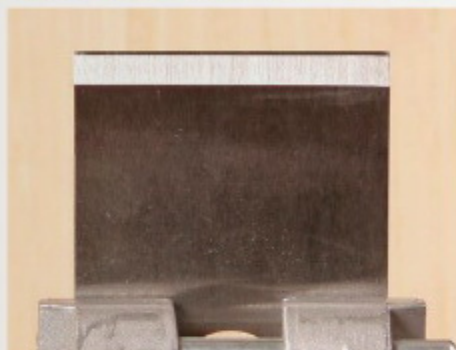
Not hip to be square. A blade sharpened with a square profile will dig in at the corners, creating ridges in the handplaned surface, called tracks.
