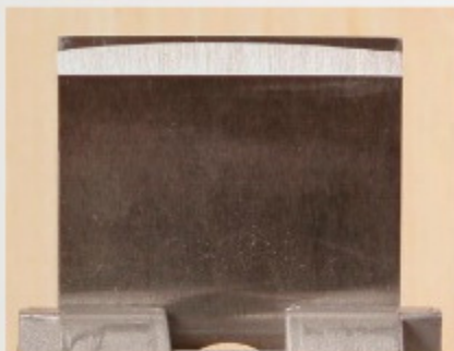
Perfect curve. The degree of camber for a smoothing plane is slight—between 0.001 in. and 0.002 in.—but it's very visible on the bevel.
