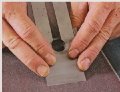
Rock and roll. A single-roller honing guide with a narrow wheel makes it easy to rock the blade to exert pressure where needed for cambering.
