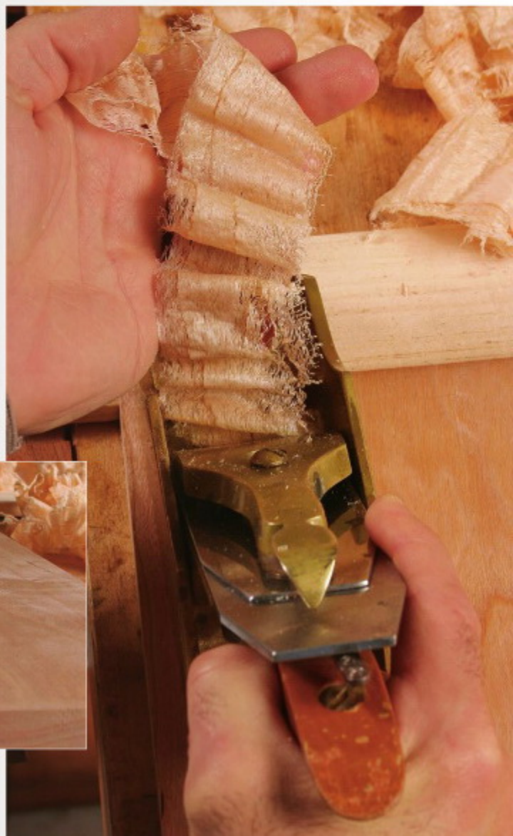
Perfect curve. The degree of camber for a smoothing plane is slight—between 0.001 in. and 0.002 in.—but it's very visible on the bevel.
