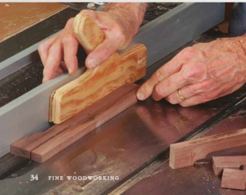
Use a stop for symmetrical feet. After routing the lower arch on the foot, move the stop and fence to rout the higher one.
