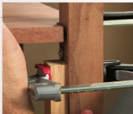
Locate the shelf. A support block clamped to the leg holds the shelf in place.
