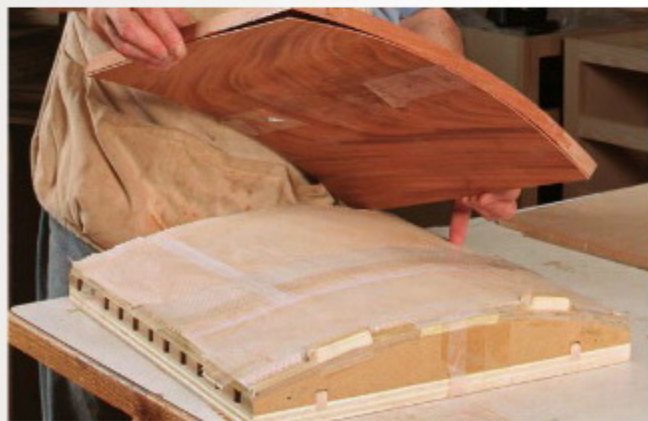
Veneer the doors. After laminating the crotch veneer to backer veneer, vacuum-press it onto the door using the same form used for the core. A layer of rubber shelf liner covered with wax paper evens out the pressure.
