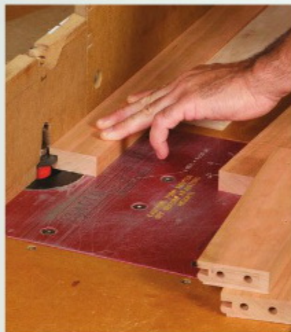
Rout the sticking. It goes on the inside edge of all four frame parts, as shown. Then rout the cope. It shapes the end grain of the rails so that they nest over the sticking on the stiles.
