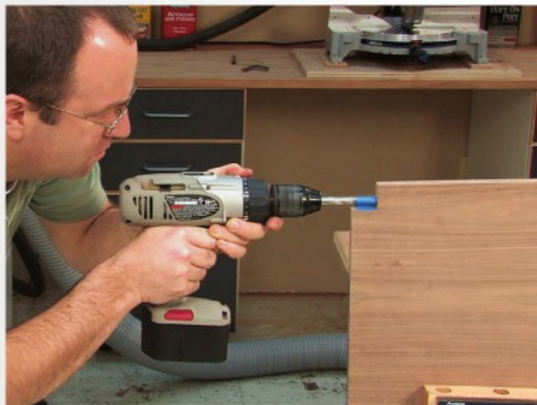
Drill the shelf edge. Eyeball the drill and the edge of the shelf to make sure the hole is straight and square.
