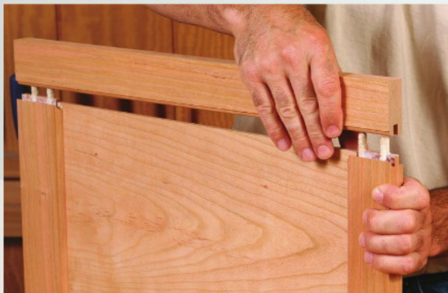
Assemble the door. Glue the dowels in the rails first. Then spread glue over the coped end grain and the exposed dowel before adding the stiles and panel.
