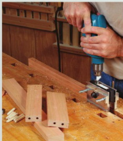
Drill holes for the dowels first. On the rails, they need to be far enough in from the edge that you don't cut into them when forming the sticking.
