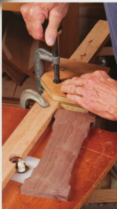
Use a stop for symmetrical feet. After routing the lower arch on the foot, move the stop and fence to rout the higher one.
