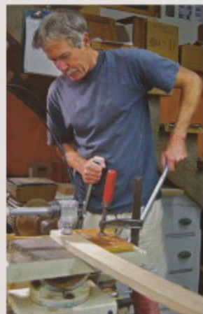
Slip tenons simplify joinery. Warner, seen here at his slot-mortiser, employs curves extensively in his furniture. Using slip tenons makes joining the curved parts far simpler.
