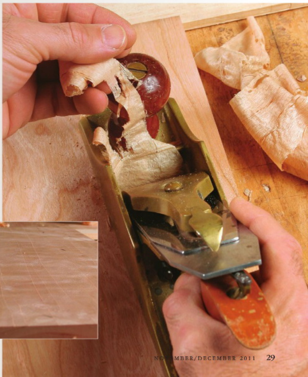
Not hip to be square. A blade sharpened with a square profile will dig in at the corners, creating ridges in the handplaned surface, called tracks.
