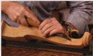
Stay in control with short cuts. They prevent the chisel from cutting too deeply and causing tearout.
