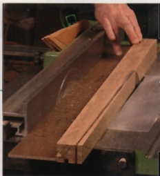
Backward taper is next. Rodel uses a simple L-shaped jig to cut the taper on the leg. Make sure your saw has its splitter in place (left).
