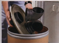
Simple assembly. Each two-part section is threaded through the lid and oriented to create a cyclone effect in the drum.
