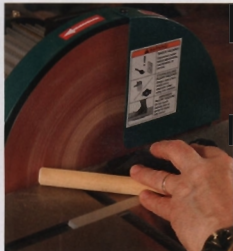
Different approach. With the miter gauge angled, you can chamfer dowels and through-tenons. Just use a light touch.
