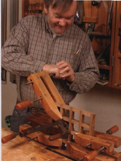
Grooves for splines and corner blocks. Use the same setup, a dado blade on the tablesaw, to cut the grooves for the spline and the corner blocks. The corner-block groove can go through, but the spline groove is stopped, so set a stop block on the rip fence and pivot the work up when you hit it. Square up the end with a chisel.
