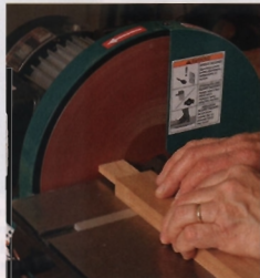
Quick trim. A disk sander trims tenons quickly. Use the miter gauge to keep the workpiece square to the disk.
