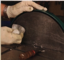
The PSA-backed sanding disks often require a fair amount of scraping to get the paper off, and leave a bit of residue behind. You can remove any adhesive residue with a solvent, such as naphtha.
