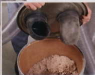
It's in the drum, not the bag. Most of the debris lands in the drum, keeping it out of the filter, where it impedes airflow.
