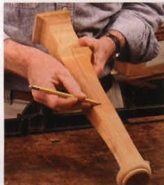
Start with layout lines. Lowe draws a center-line and two quarter lines on all four faces, so he'll know how much material to remove.
