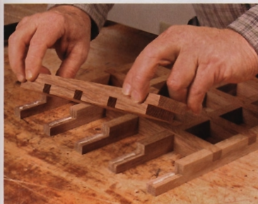
Putting the grids together. Glue and clamp the entire grid at the same time, joining the center pieces first and then moving outward (above). To avoid crashing clamps, use a vise to hold the grid and apply clamping pressure to part of it, and add clamps to the rest of the intersections (right).
