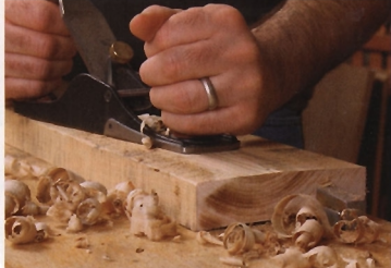
Go over the hump first. Flatten the convex side. On most boards, that removes about 1/8 in. Then put your planes to work on the concave side.
