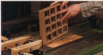
Grooves for splines and corner blocks. Use the same setup, a dado blade on the tablesaw, to cut the grooves for the spline and the corner blocks. The corner-block groove can go through, but the spline groove is stopped, so set a stop block on the rip fence and pivot the work up when you hit it. Square up the end with a chisel.
