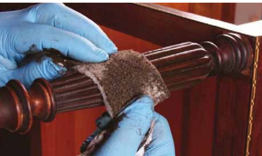
Fill grain on carvings, too. A clever way to fill the pores on carvings is to take a pad used to remove surplus filler from flat surfaces, and rub it over the carving, working it into the recesses, too.
