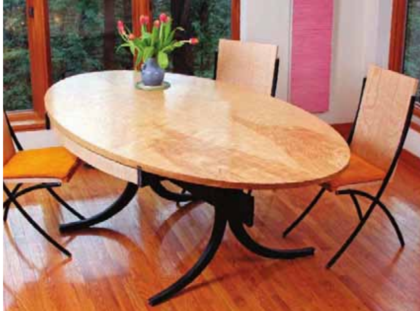
Big boards, beautiful book-match. It takes a bit more work than veneer does, but this table by Rob Hare shows that you can get a great looking book-match from sequential boards cut from the same log.
