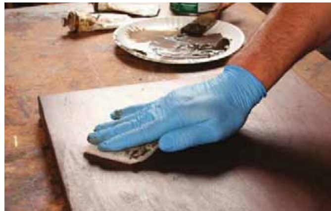
Clean the surface. A white abrasive pad does a great job scrubbing any remaining filler from the surface while leaving the pores filled. Don't wait or the filler will harden on the surface.
