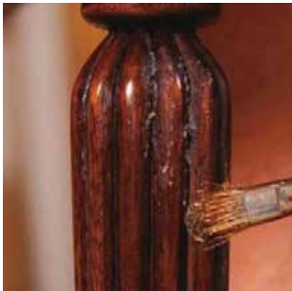
Wax the recesses. To imitate dust buildup, begin by using an old artist's brush to push clear paste wax into the recesses of carvings.
