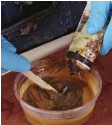
Tint the grain filler. Gedrys likes to use uncolored, oil-based grain filler that he tints using artist's oils.
