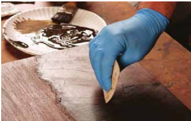
Pack the pores. Use an old paintbrush to force the filler into the pores. Let the filler cure for a few minutes and then pull a plastic squeegee across the surface perpendicular to the grain to remove the excess.
