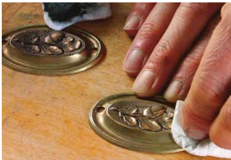
Patinating pulls. To add contrast to the antique-finish pulls, first use brass polish to give shine to the wear points, then rub some dark wax into the recesses. Finally, buff the whole surface with a clean cotton cloth.
