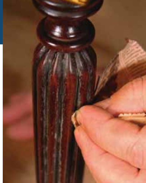
Complete the effect. After 20 minutes, use a piece of folded newspaper to remove most of the rottenstone but leave traces deep in the recesses.
