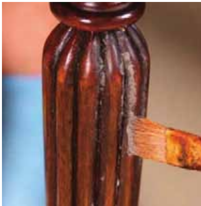
Add your dust. Brush rottenstone onto the freshly waxed areas. Rottenstone's pale blue/gray cast mimics dust well.
