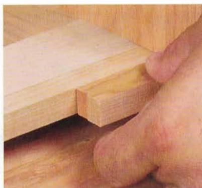
Glue, then shape. It's easier to glue oversize blocks to the frame and then shape them than it is to shape tiny pieces on the bandsaw and then try to clamp these irregular parts to the divider.
