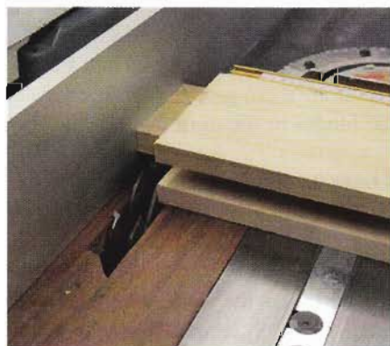
Poplar frame, plywood skin. A groove in the center of the 1 1/2-in. thick poplar stock receives stub tenons formed on the ends of the rails with a dado set (left). Although most of the strength comes from the plywood skins, stub tenons help keep everything square during the large glue-up (right). Once the glue dries, the interior compartments are filled with 1 1/2-in.-thick rigid insulation.
