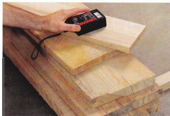
Moisture meter removes doubt. Ideally, the moisture content of new lumber should match the moisture content of wood already acclimated to your shop.
