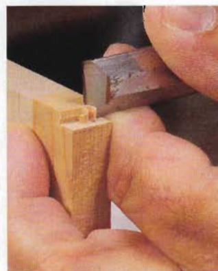
Test-fit the dividers. If the fit needs adjustment, plane the bottom face of the frame to fit. That way, if there is tearout or any other issue, it won't be noticeable. With the dividers pushed up against the end of the dado (far left), lay out the notch and use a handsaw and chisel to cut it (near left).
