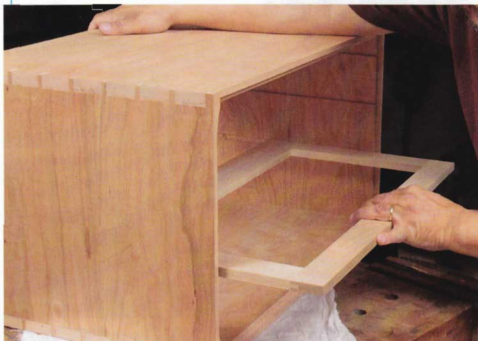
Test-fit the dividers. If the fit needs adjustment, plane the bottom face of the frame to fit. That way, if there is tearout or any other issue, it won't be noticeable. With the dividers pushed up against the end of the dado (far left), lay out the notch and use a handsaw and chisel to cut it (near left).
