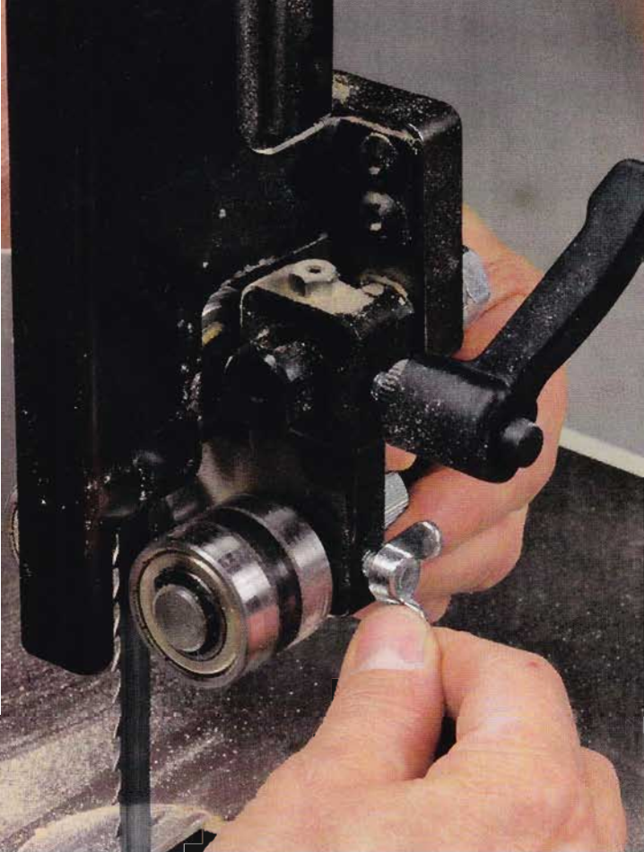
Tool-free is faster. Jet's easily adjustable roller guides move without tools and stay put when locked down.
