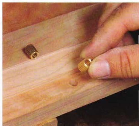
Pins and sockets keep the lid in place. Basic brass hardware (rockler.com; No. 32334) is pressed into holes drilled into the case and lid bottom.
