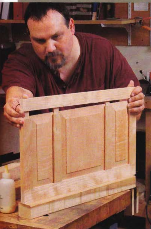
Prefinish the panels. Brown applies the polyurethane finish to the panels before gluing them into the frames so seasonal movement doesn't expose unfinished wood.
