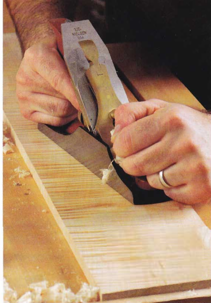
Standard smoothers are up to the job. Even on grain prone to tearout, a No. 4 smoother with a sharp blade leaves a finish-ready surface.
