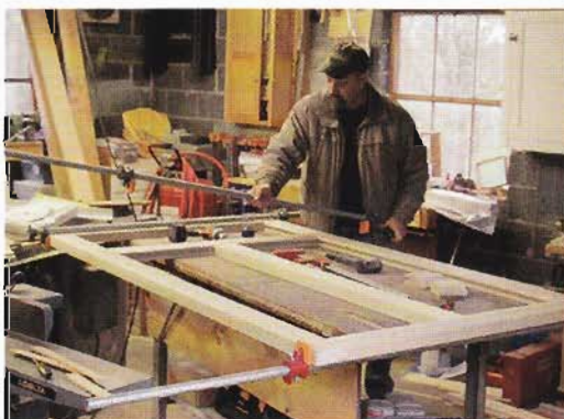
Poplar frame, plywood skin. A groove in the center of the 1 1/2-in. thick poplar stock receives stub tenons formed on the ends of the rails with a dado set (left). Although most of the strength comes from the plywood skins, stub tenons help keep everything square during the large glue-up (right). Once the glue dries, the interior compartments are filled with 1 1/2-in.-thick rigid insulation.
