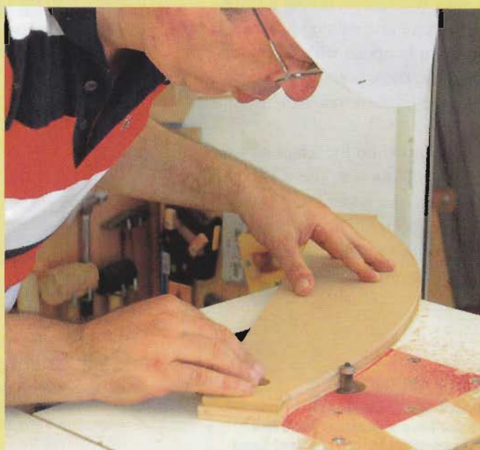
Shape the workpiece at the router table. The author's version doesn't have through-the-table height adjustment, relying on automotive technology instead (see drawing, facing page).
