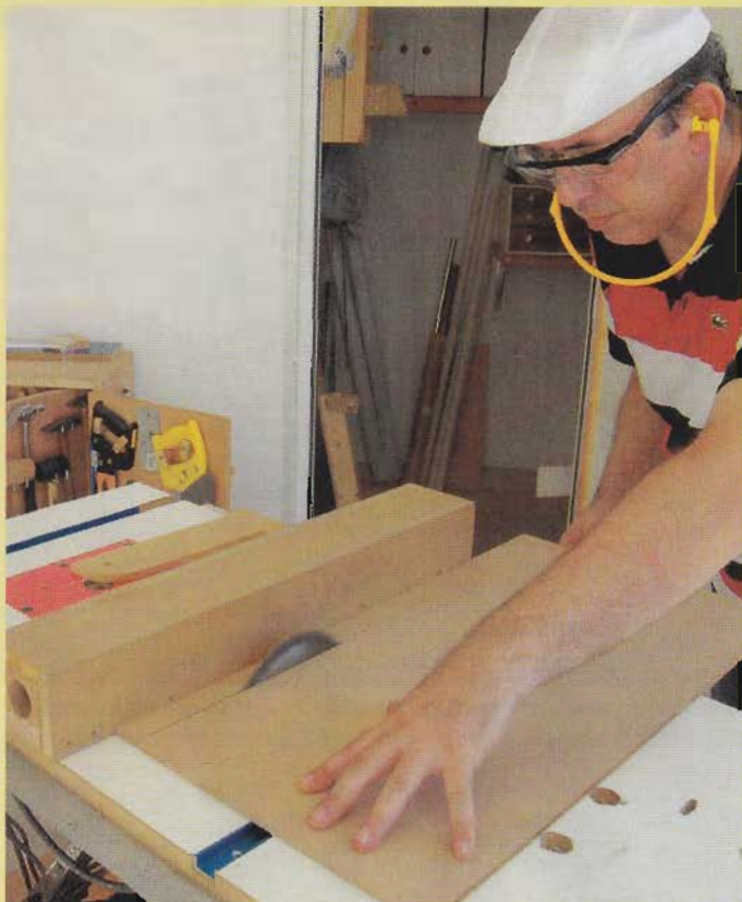
The circular saw yields straight, clean cuts. Note that the rip fence doubles as a router-table fence and includes dust collection.
