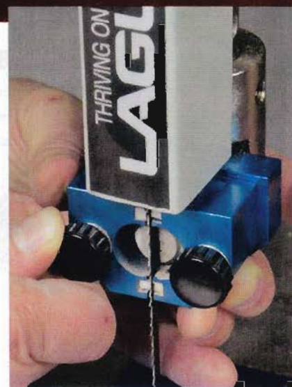
A little pinch. Designed to run with slight pressure on the blade, Laguna's ceramic side guides are easy to set and give excellent blade support.
