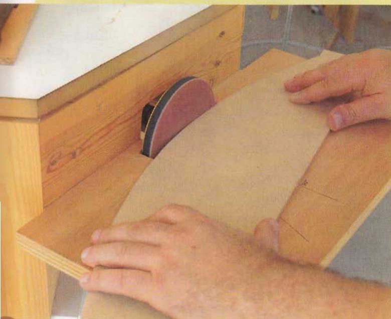
Fair the curve at the sanding station. A flip-up table supports the work. The sanding attachment uses hook-and-loop pads and is powered by a variable-speed electric drill.
