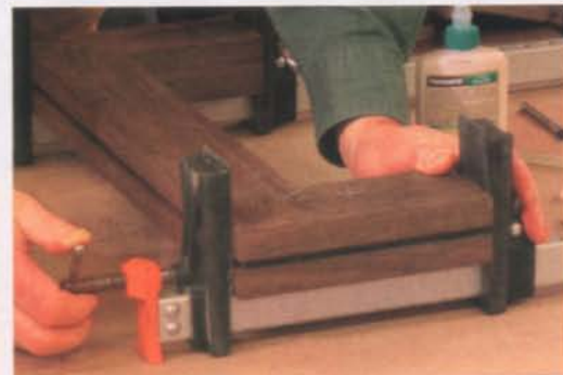
Tenons brace the corners. Each miter gets four slip tenons (left). Glue up the mitered feet first (above), then attach them to the stretcher assembly (below).
