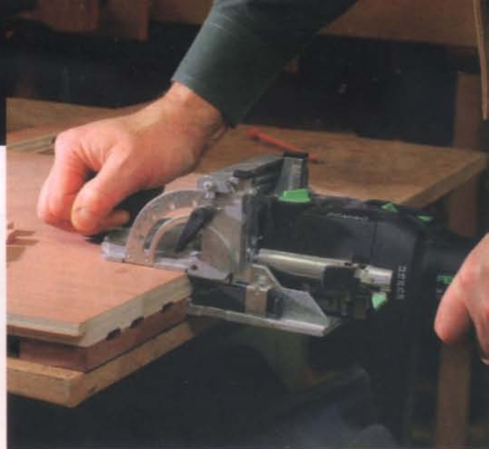
More tenons, more strength. Festool's Domino creates rows of slip-tenon joints in minutes. In the sides, Burkin moved the mortises partway into the glue blocks to accommodate the rabbet that follows.
