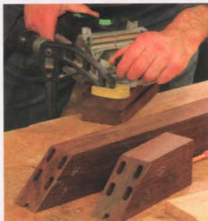
Tenons brace the corners. Each miter gets four slip tenons (left). Glue up the mitered feet first (above), then attach them to the stretcher assembly (below).
