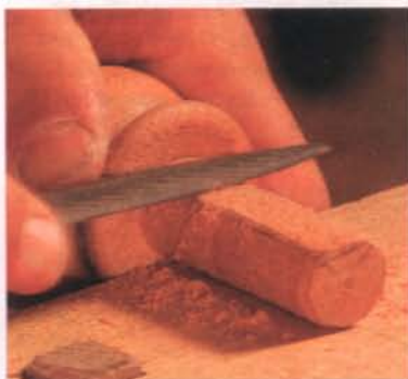
Create a flat on the tenon. The tenon will be exposed by the cut-away portion of the leg. The flat surface lets the legs marry to the beveled corners of the case.
