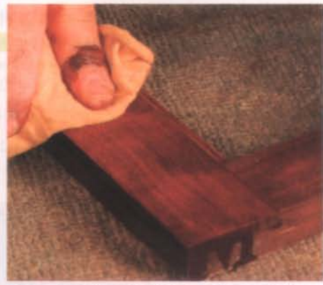
Re-sand while wet. While the finish is still wet, sand the wood with the last grit you used (left) until all the cross-grain scratches are removed. Wipe more stain onto the bare wood (above) and blend it into the surrounding area.
