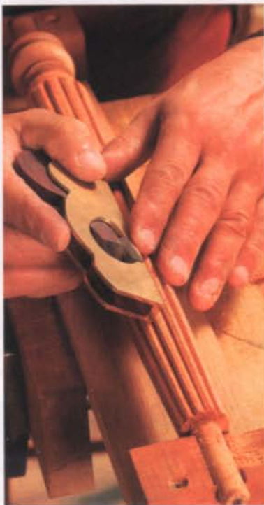
Shaping the reeds. Rodriguez mounts the workpiece in a shopmade jig, then uses a variety of tools to round the tops of the reeds and sharpen the grooves.
