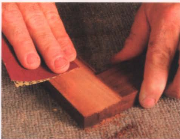
Re-sand while wet. While the finish is still wet, sand the wood with the last grit you used (left) until all the cross-grain scratches are removed. Wipe more stain onto the bare wood (above) and blend it into the surrounding area.
