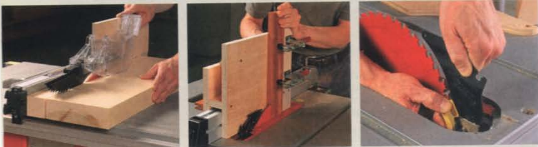
All new saws have riving knives. In our recent review of portable tablesaws (FWW #209), the type Carlos Osorio was injured on, we found state-of-the-art riving knives and blade covers, designed to stay on the saw for most types of cuts, and come off in a snap when necessary.
