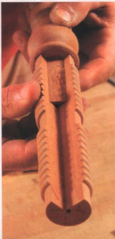
Create a flat on the tenon. The tenon will be exposed by the cut-away portion of the leg. The flat surface lets the legs marry to the beveled corners of the case.
