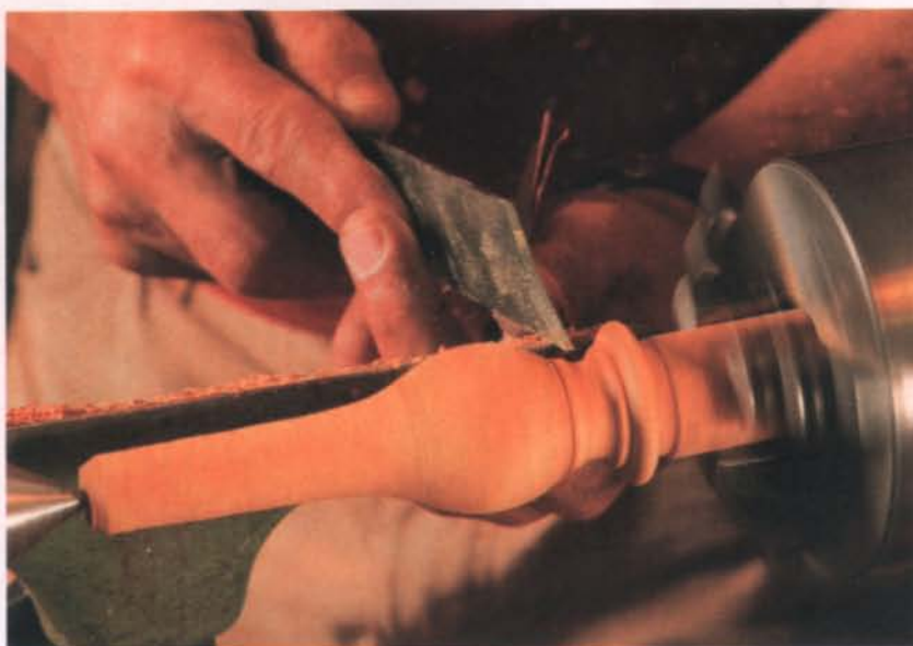
A graceful foot. Use the shopmade mandrel again to mount the foot blank on the lathe, using the tailstock and a live center again to stabilize the piece. The foot is shaped using a parting tool and a variety of spindle gouges.
