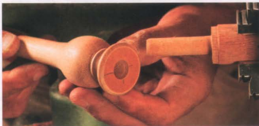
A graceful foot. Use the shopmade mandrel again to mount the foot blank on the lathe, using the tailstock and a live center again to stabilize the piece. The foot is shaped using a parting tool and a variety of spindle gouges.
