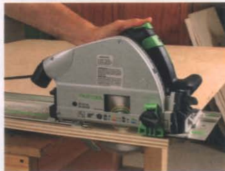
Sharp teeth. New 160 mm blades from Forrest and Freud are sized for track saws like Festool's TS 55. The Freud performed as well as the others, and costs less.
