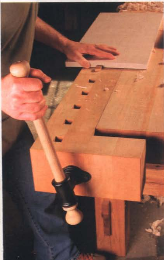
Tail vise. The tail-vise hardware rides in grooved slides. One of the slides is adjustable so you can fine-tune the fit between the moving steel plate and the slides it rides in.
