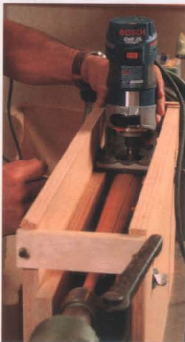
A box for reeding. Before mounting the workpiece between the lathe centers, Rodriguez clamps the reeding jig to the lathe bed.
