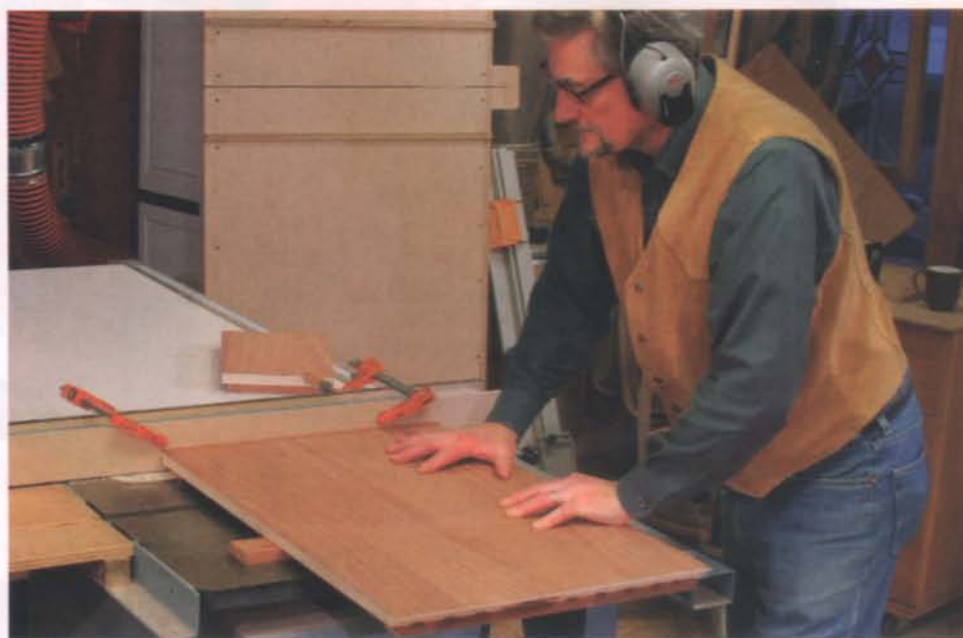
Use a dado set to rabbet the sides. Bury the blade in a sacrificial fence to dial in the width. Place an offcut from the glue-block stock under the workpiece to stabilize it.
