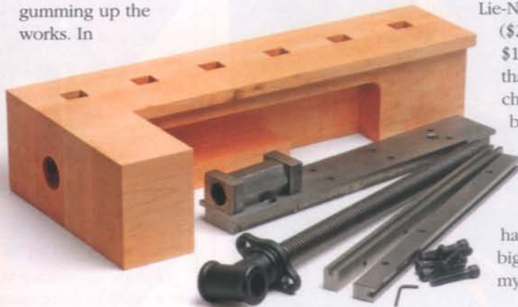
Tail vise. The tail-vise hardware rides in grooved slides. One of the slides is adjustable so you can fine-tune the fit between the moving steel plate and the slides it rides in.
