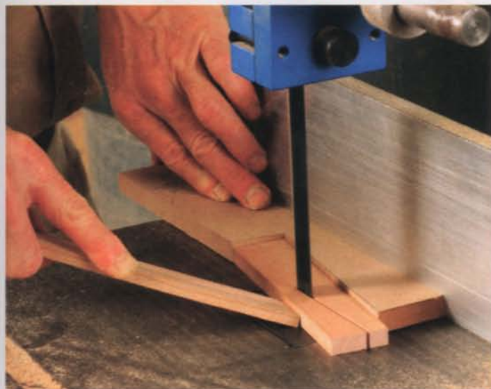
Bandsaw is safer than tablesaw. Rogowski uses a simple jig made of \frac{3}{4} -in. MDF with an 8° notch cut into it.
