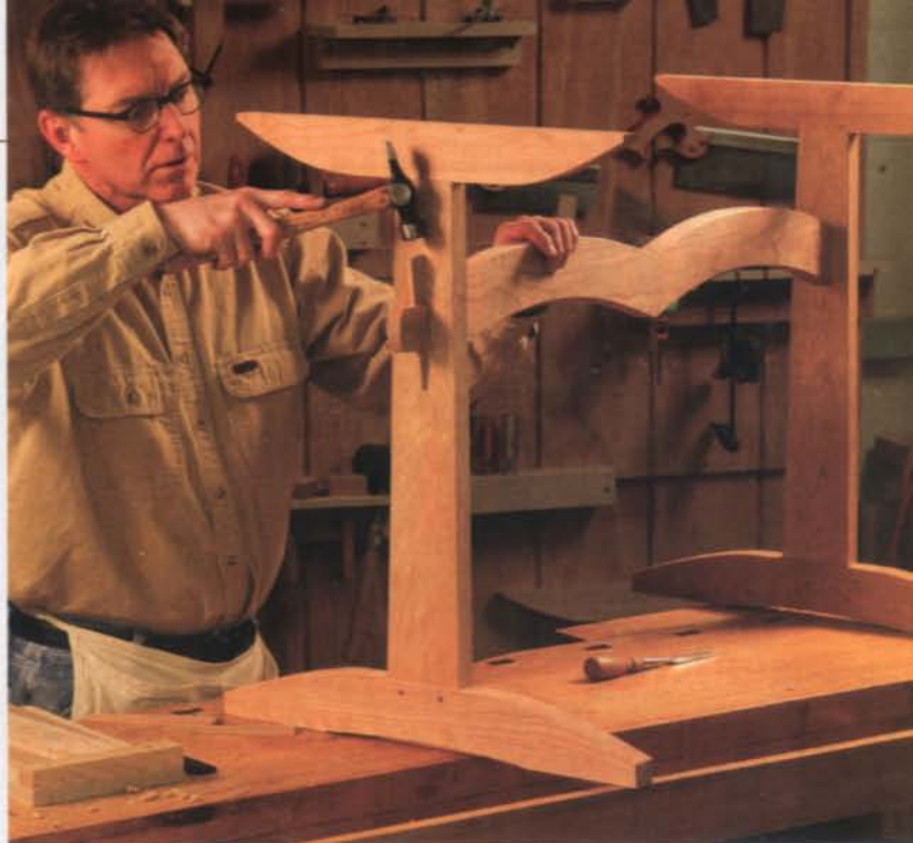
Tap the wedges home. When the wedges are tightly driven, they pull the tenon shoulders firmly against the post for an assembly that won't budge.
