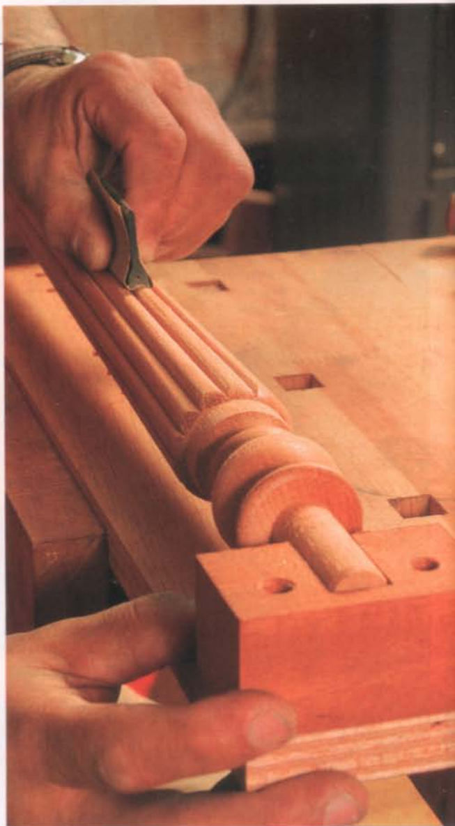
Shaping the reeds. Rodriguez mounts the workpiece in a shopmade jig, then uses a variety of tools to round the tops of the reeds and sharpen the grooves.
