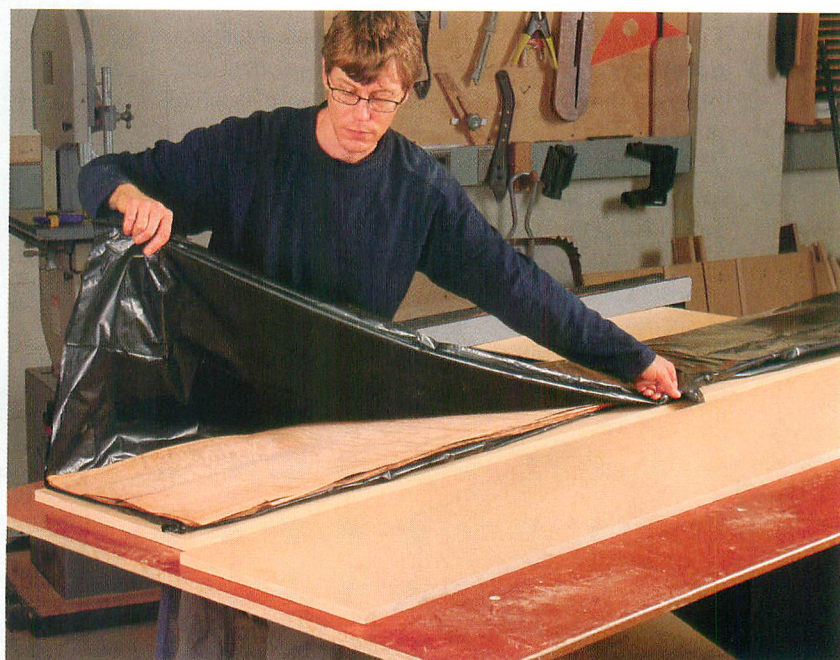
For best results, veneer should be flexible and flat. Wrap it in plastic so it doesn't dry out and become brittle, and then place it between two pieces of MDF to keep it flat.
