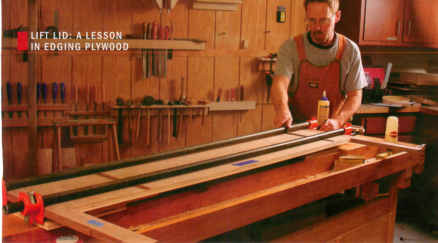
Fixed back gets solid edges. Attach the side trim pieces to the fixed back with biscuits.
