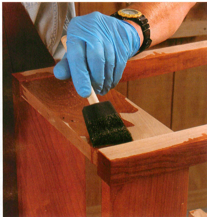
Foam brushes don't lay down perfect topcoats. But they are perfect for slopping on finishes that are soon wiped off, like boiled linseed oil.
