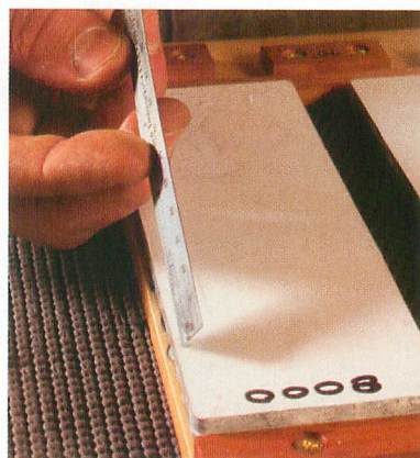
Tiny ruler is a huge time saver. Lifting the iron's back off the stone lets you polish only a thin band at the cutting edge, instead of the entire back. The work is done with just 10 to 20 passes on an 8,000-grit stone.
