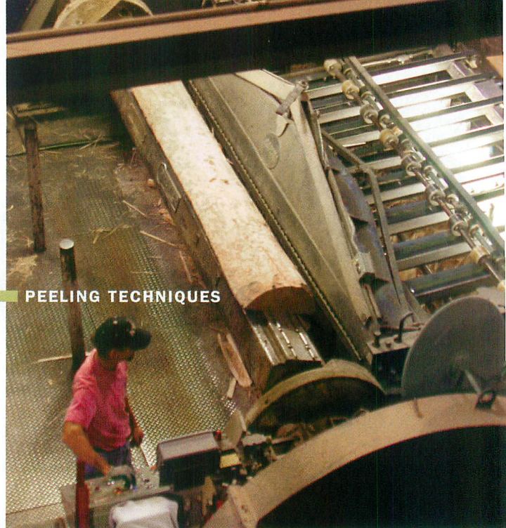
Round and round. Rotary-cutting, or peeling, produces wider sheets from smaller logs and is also used for certain figured veneers.
