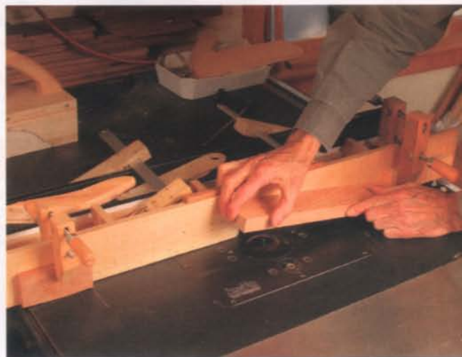
Stopped grooves in the top and bottom. With two stop blocks clamped to the fence so that the bit lines up in the mortise holes at each end, pivot down into the first hole with the router running, run the groove, and lift the workpiece out of the second hole.
