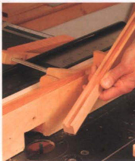
Through-grooves on the sides. With a straight bit on the router table, run through-grooves on the two side pieces.
