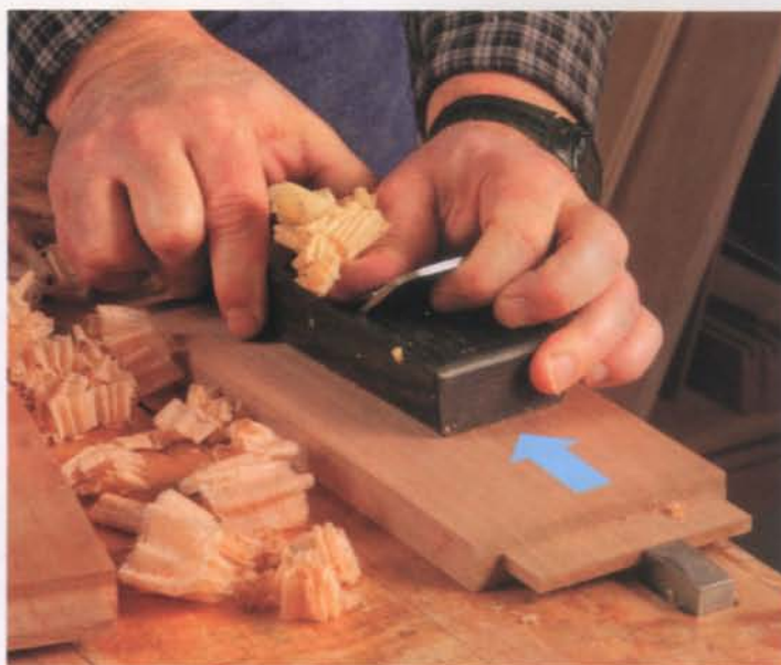
No pushing. The 8-in. ebony plane from Woodline works best when pulled rather than pushed.
