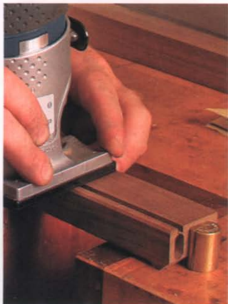
Chamfer the rails. The front, back, and side rails receive a decorative chamfer along their inside edges.
