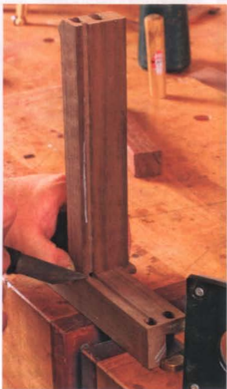
Stop-chamfer the legs. Dry-fit the rails to the legs and lightly mark where they meet (above). Chamfer the inside corners on the show faces of the legs. Stop just short of where they intersect with the rails (right). The mason's miters will be completed after the table base is assembled.
