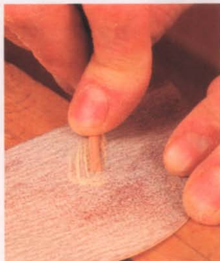
Flatten the dowels to create a perfect fit. Sand a flat into each dowel and then insert it, flat side against the top of the frame, until hand tight.
