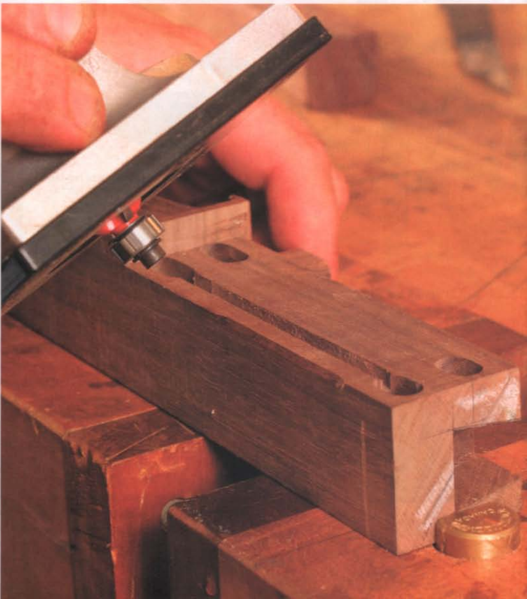
Stop-chamfer the legs. Dry-fit the rails to the legs and lightly mark where they meet (above). Chamfer the inside corners on the show faces of the legs. Stop just short of where they intersect with the rails (right). The mason's miters will be completed after the table base is assembled.
