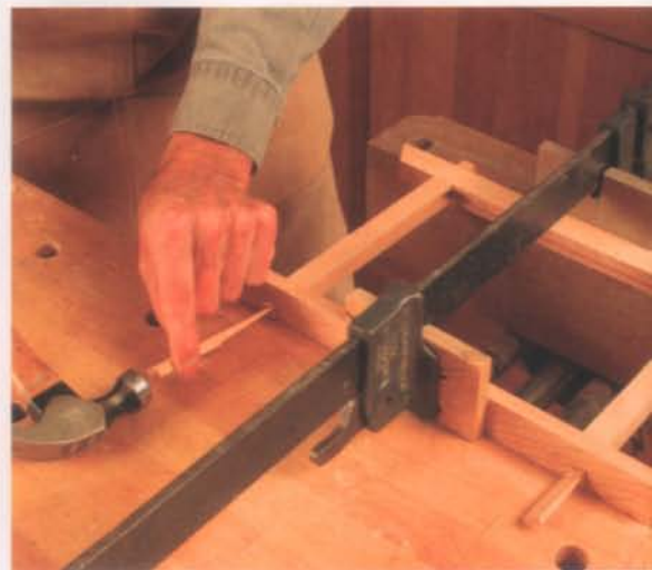
Tap in wedges. Glue the sides into the bottom, set the top in place for clamping, glue the wedges, and tap them into place. Saw the tenons and wedges flush, and then smooth the bottom with a block plane.
