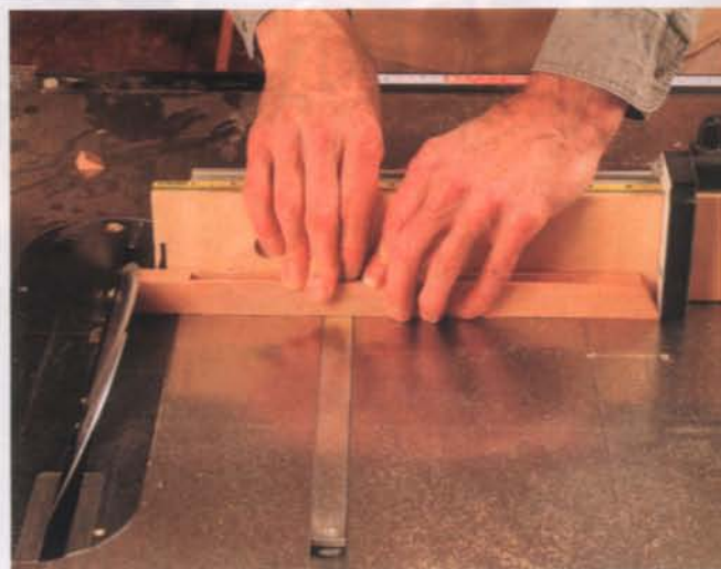
Angle the ends, too. With the tablesaw blade still tilted from the bevel, use a miter sled and cut angles on the ends of the top and bottom.
