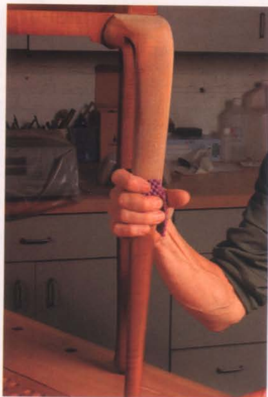
Foam mesh. 3M's Sandblaster is a drawer-liner type of foam mesh coated with abrasive. It can be folded over to reach into tight corners or wrapped around curves.
