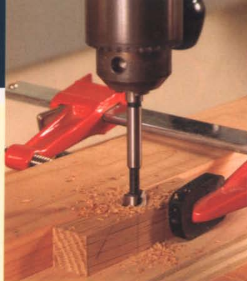
A mortise houses the pressure pad. Drill a stepped through-mortise to hold the pad and the threaded insert.
