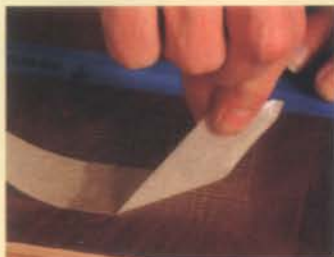
Perfect adhesion. No finish from the scratched area stuck to the tape when he pulled it away.
