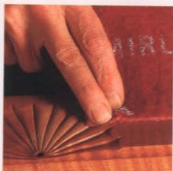
Abrasive pads. These pads come in a variety of grits and are thin enough to get into carvings.
