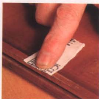
Sticky paper. Adhesive-backed sandpaper is useful for sanding narrow surfaces. Simply stick it to a finger.
