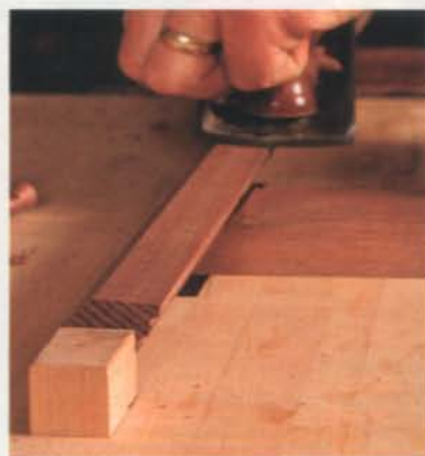
Plane to fit. The radius of the turning is oversize to leave room for ripping and handplaning the sides until they fit.
