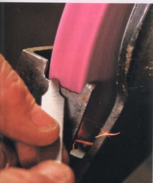
Two profiles on one piece. Start with a piece of card scraper or old hacksaw blade. On one end, grind the rounded profile for scraping the fluting (left). On the other end, grind the concave profile for the beaded stop-fluting (above). Any burr raised is insignificant, and the tool is used in both directions.
