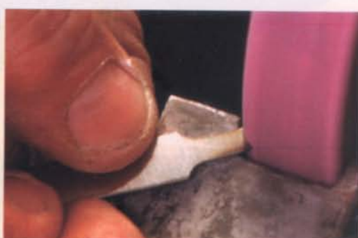
Two profiles on one piece. Start with a piece of card scraper or old hacksaw blade. On one end, grind the rounded profile for scraping the fluting (left). On the other end, grind the concave profile for the beaded stop-fluting (above). Any burr raised is insignificant, and the tool is used in both directions.
