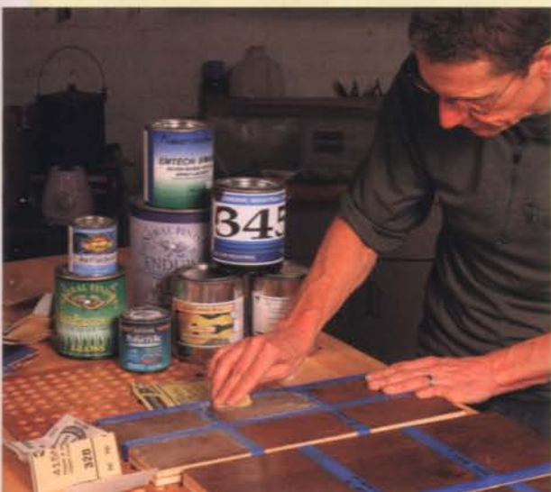
Tough test reveals the truth. Jewitt applied eight waterborne finishes to a sample board and then sanded sections with different stearted sandpapers before adding a final coat of each finish.
