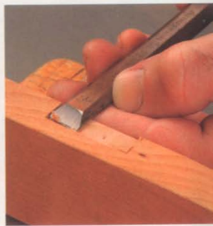
The jig squares corners, too. The square opening makes a perfect chisel guide. Remove the template to pare away the waste (below).
