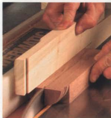
Eight parts from one turning. Rip the turned blank into four equal sections, four capitals and four bases.
