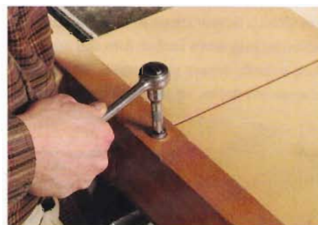
Wiggle room. Use bolts and slightly oversize holes when you need room for adjustment, such as on this crosscut-sled fence.
