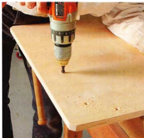
Clearance hole first. Each screw requires a shank hole and a shallow countersink for the screw head.
