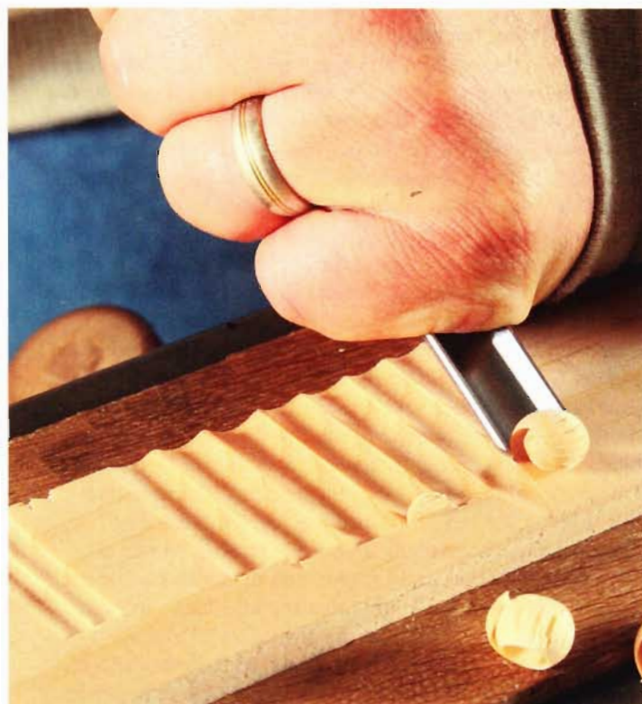
Do your carving tools cut like this? A series of clean cross-grain cuts with clearly defined ridges and no tearout indicates a sharp gouge.
