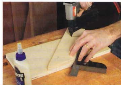
Pinned down. A few strategically placed brads keep the parts from shifting during glue-up.
