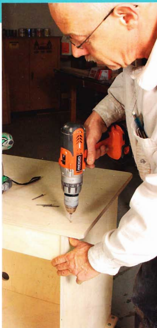
Pilot hole next. Align the parts and drill pilot holes into the plywood edges below. This makes them much less likely to split.
