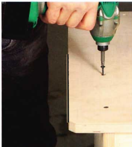
No glue needed. Drywall screws provide plenty of holding power, so there's no need to fuss with glue.
