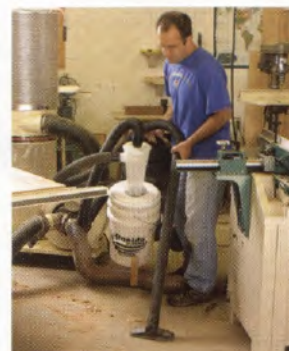
Not very portable. The Dust Deputy and shop vacuum in tandem result in a rig that's awkward and tippy. A short wood leg added to the Deputy bucket helps keep everything upright.
