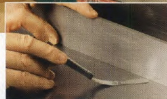
Check for flatness first. Use a straightedge and feeler gauge to test each table at each edge and in the middle.
