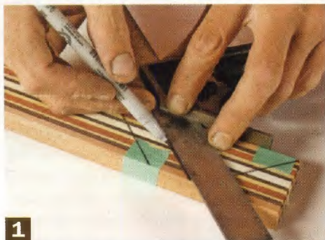
1 Lay out the segments. Tape together a stack of the striped veneers and lay out the geometric shapes, keeping them slightly oversize.
