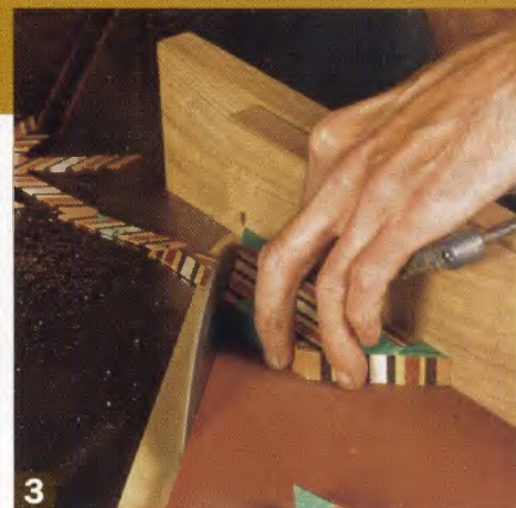
3 Uniform, precise cuts. After rough-cutting the shapes, tape them back together and trim them all to the final size.
