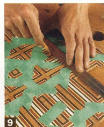
9 Cut away the side veneer panels. Align a straightedge with the ends of the side sections of veneer and mark where to slice the side veneers away from the top piece.
