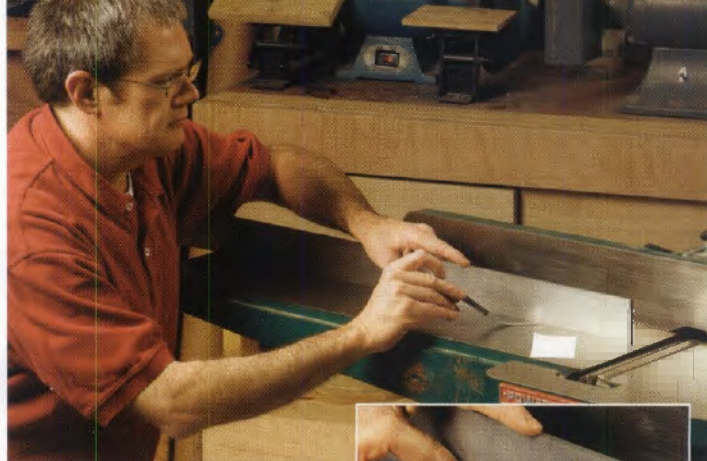
Check for flatness first. Use a straightedge and feeler gauge to test each table at each edge and in the middle.
