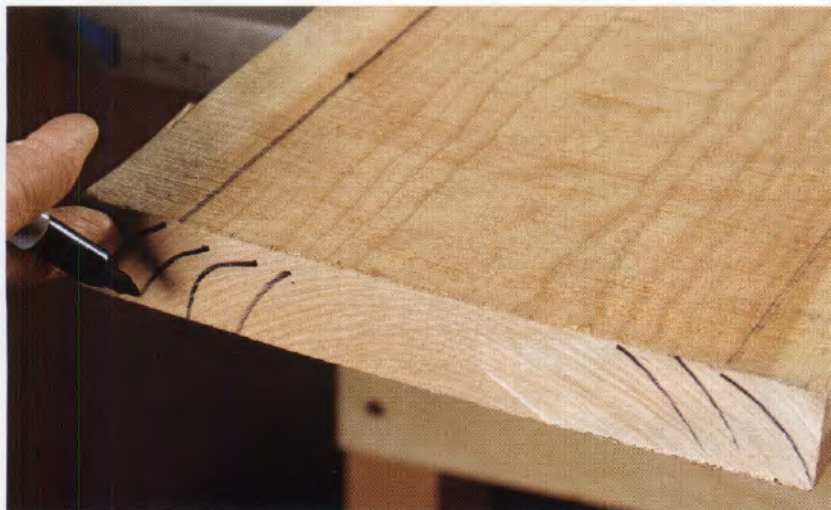
Riftsawn edges add stability. Try to find boards where the growth rings run at about 45° to the face where the finished edges will be. This ensures that the sections of the top will stay flat.
