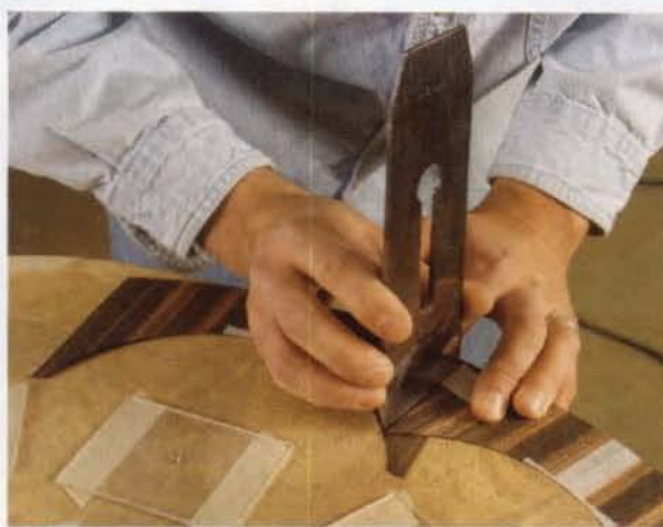
Align the pieces. Place the book-matched joint in the border on the center line of a sunburst segment. Then cut the veneer along a line that extends from the sunburst seam.
