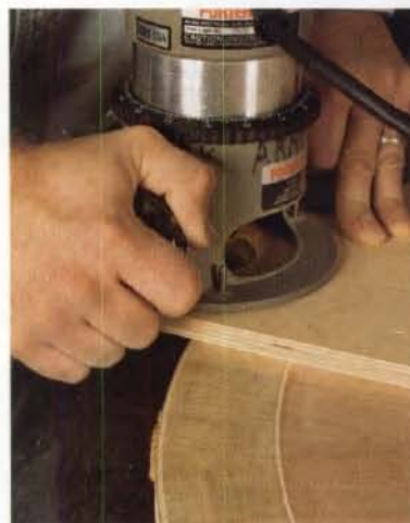
The final cut. Use the trammel-mounted router one last time to cut a 1/8-in.-square rabbet on the top corner of the tabletop.
