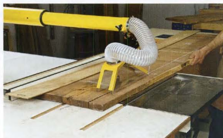
Serious curve? Saw it. Tack a straightedge guide board to the workpiece (above left). The guide runs against the fence so the saw can make a straight cut (below left). Anthony keeps several lengths of \frac{1}{4} -in. plywood on hand for this. He puts the nails into a waste area of the board.
