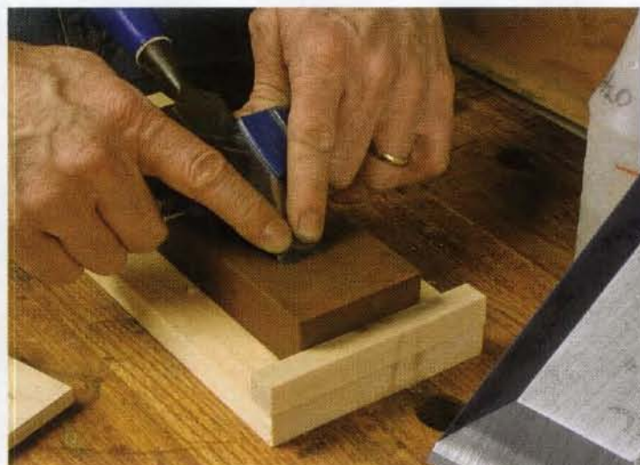
Precision honing. By setting the jig slightly steeper than your grinding angle, you polish just the tip of the tool.
