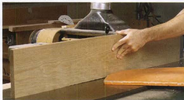
Mild curve? Joint it. With relatively straight stock, a pass or two over the jointer should yield an edge straight enough to run against the tablesaw fence.
