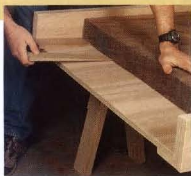
Steady the slab. Push shims under the slab to prevent it from wobbling in the jig as you flatten the face.
