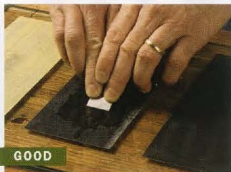
The alternative. Rogowski suggested setting up a station like this, with individual strips of sandpaper held in place with spray adhesive.
