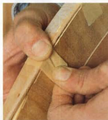
Added protection. A strip of hard maple protects the vulnerable veneered edge.
