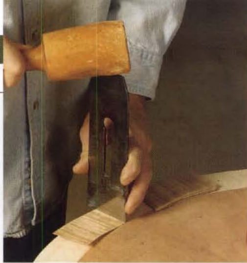
A clean cut. A plane iron creates a tight seam when joining the sections.
