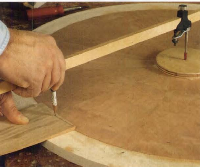
Prepare the sections. Use a trammel to scribe the sunburst curve onto a stack of border veneer.
