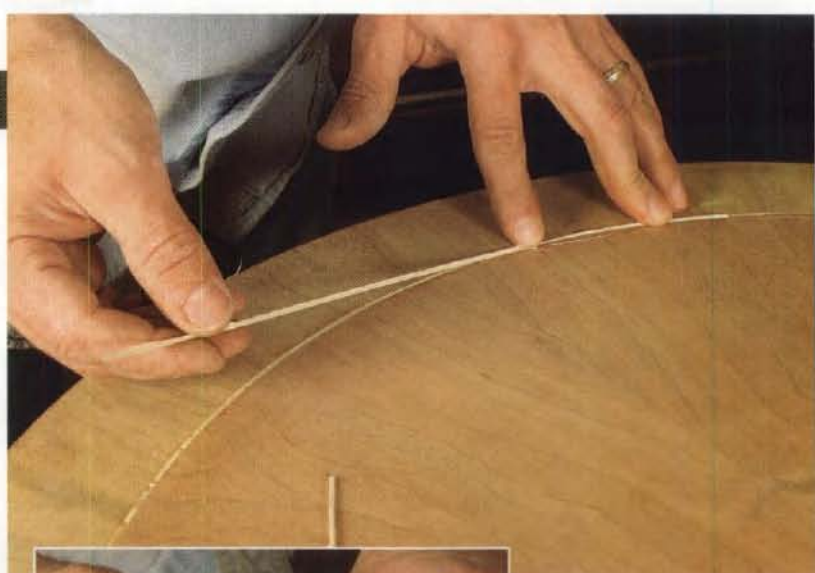
Insert the stringing. Use a syringe to insert glue into the groove, and then add the holly stringing. When the glue has dried, bring the stringing flush with a scraper.
