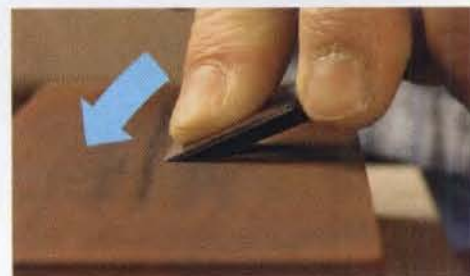
Lock the arms to lock in the angle. Rogowski showed Cecala how to concentrate pressure on the blade's tip while keeping his arms rigid to help maintain the honing angle.
