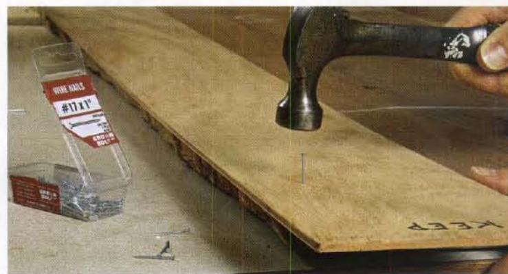
Serious curve? Saw it. Tack a straightedge guide board to the workpiece (above left). The guide runs against the fence so the saw can make a straight cut (below left). Anthony keeps several lengths of \frac{1}{4} -in. plywood on hand for this. He puts the nails into a waste area of the board.
