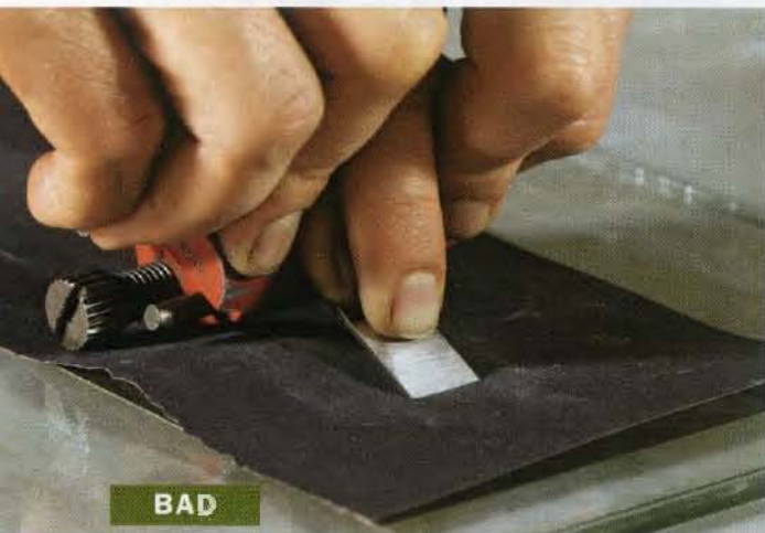
Catch a wave. Petersen's loosely stacked sandpaper bowed up in front of and behind the cutting edge.
