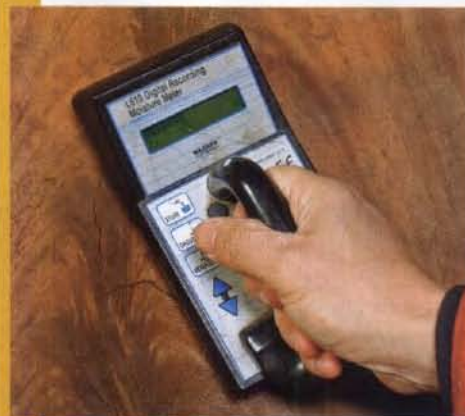
Check the dryness. Use a moisture meter to determine whether the wood is dry enough. Aim for a moisture content of about 11% or less.
