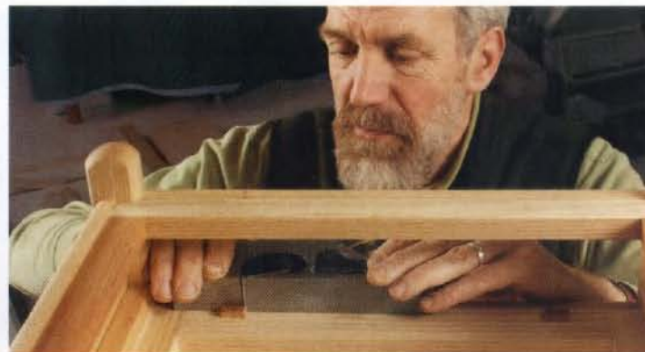
Dial in the reveal. Insert the drawer to check its alignment. Then trim the stop as needed, using a shoulder plane set for an ultralight cut.
