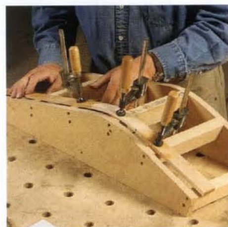
Multiple parts. If you are making several identical parts such as chair back slats, it can be quicker to build a single large setting jig.
