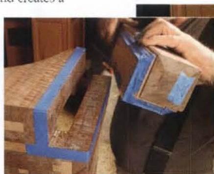
Glue the legs in place. Taping anywhere squeeze-out will seep onto the end grain or surrounding area will save you cleanup time (above). Once the leg is glued in place, apply clamp pressure in both directions (right).
