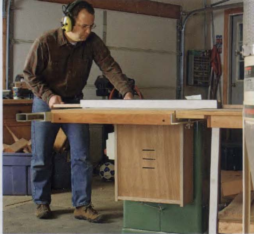
Add intake. Christiana had a plywood box covering the motor opening. So he just routed three slots, positioned to wash cool air over the motor.
