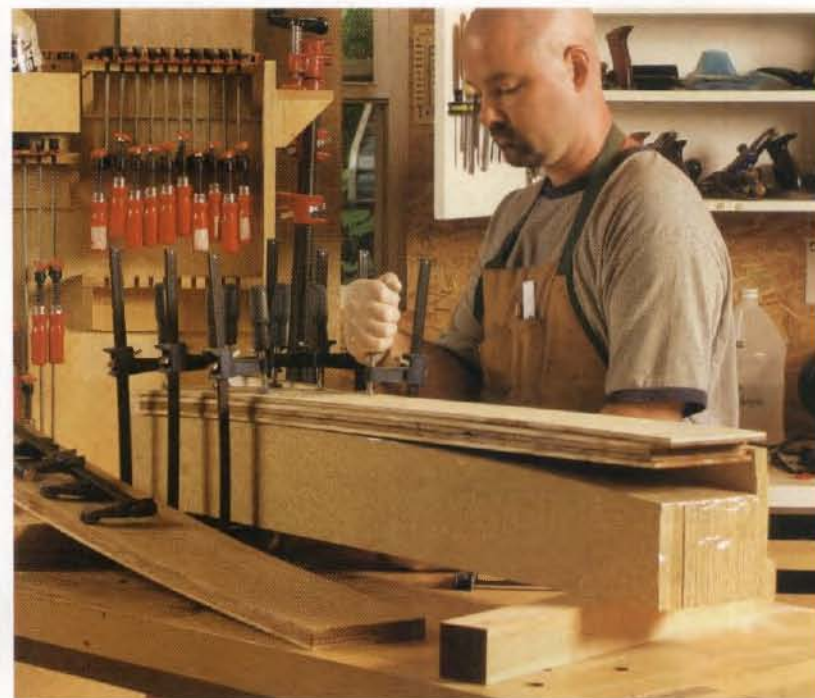
Clamps, clamps, clamps. After coating the plies with glue, press them against the stop and fence. Add a flexible caul on top and start clamping next to the stop. Work progressively down along the form. Place a clamp every 2 in. You'll need two dozen.
