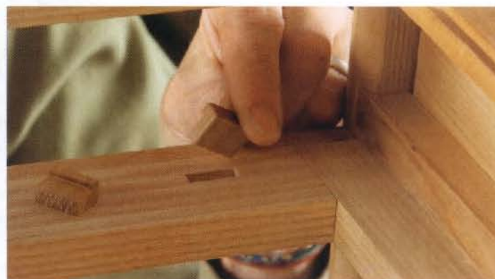
Drop in the stops. After gluing up the case, install the stops in their mortises. Just remember to orient the lip outward.
