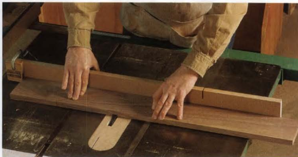
Cut accurate dados. The twin-gauge setup works well for making cuts across the middle of a long workpiece. Used miter gauges are inexpensive and easy to find at flea markets or online.
