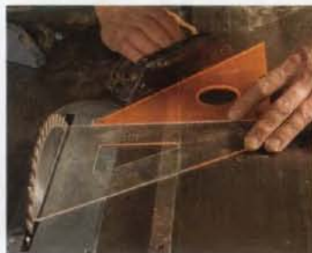
Setting up an angled cut. Use a pair of drafting triangles to set the gauge for a 45° cut. Also be sure the triangle is against the body of the blade and not a tooth, and set the gauge so the leading end of its fence points toward the blade.
