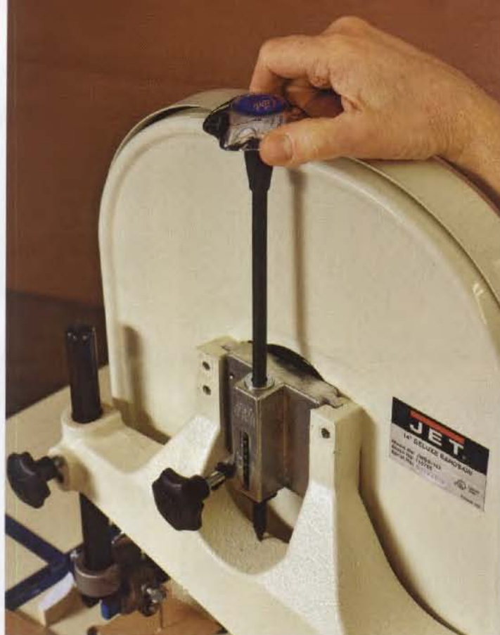
Better tension adjuster. The knob on this aftermarket tension adjuster has a ratcheting action, so your hand doesn't have to work as hard.
