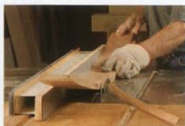
Rip to width. The second edge can be cleaned and squared, and the apron cut to width, all at once at the tablesaw. Rip it concave side up, keeping the piece against the table at the leading edge of the blade. Use a splitter to keep the piece on track.
