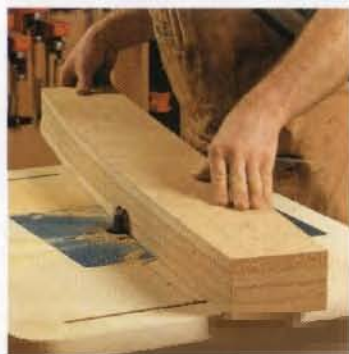
Build the form layer by layer. Make the first layer at the bandsaw, cleaning it up with sandpaper. Glue and screw on each successive layer and rout it flush.
