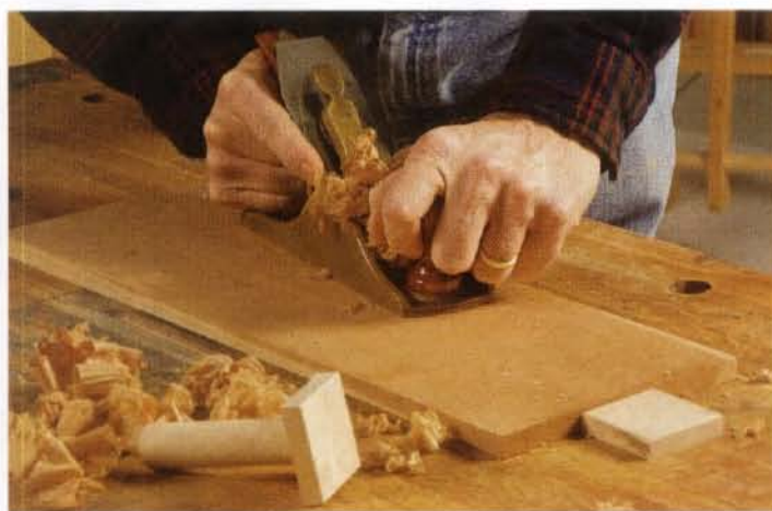
Drop-in stop. With round benchdogs, you can quickly make a planing stop, and easily match the stop's thickness to the workpiece.
