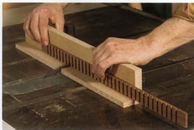
Add an L-shaped fence for small work. The fence helps prevent tearout in small work like this dentil molding. The sawkerf in the fence also helps locate cuts in the workpiece. To make the fence, screw a 2-in.-wide strip of 1/2-in. MDF to the bottom edge of a 3/4-in. piece.
