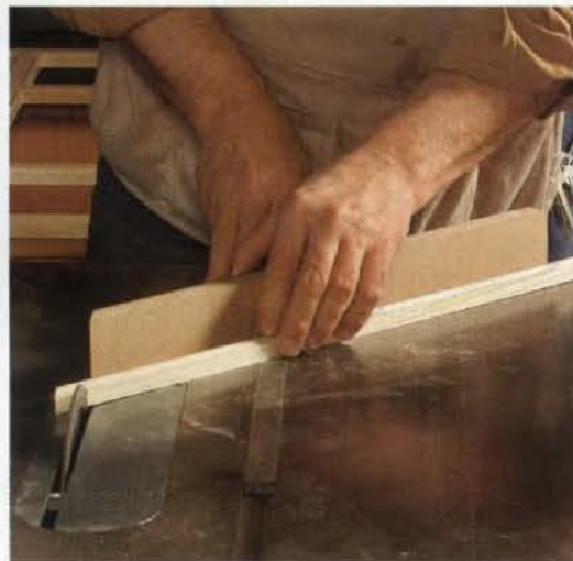
Setting up an angled cut. Use a pair of drafting triangles to set the gauge for a 45° cut. Also be sure the triangle is against the body of the blade and not a tooth, and set the gauge so the leading end of its fence points toward the blade.
