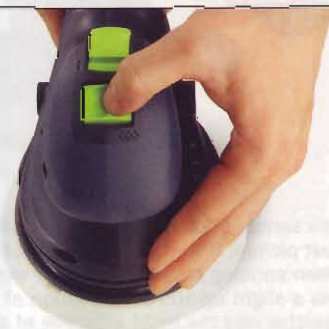
A random-orbit fingerprint. The combination of an eccentric orbit and rotation of the pad creates the swirling, random scratch pattern.
