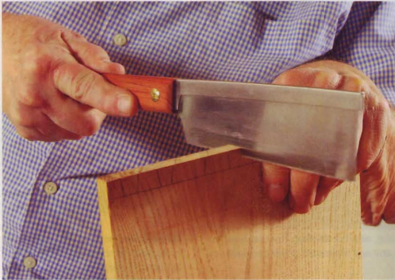
Gentler on the wrist. A Japanese-style saw cuts on the pull stroke and requires less force.
