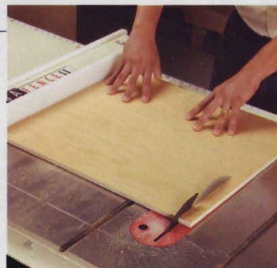
Pivot protection. A workpiece that inadvertently pivots into the teeth at the back of the blade is likely to go airborne. A splitter or riving knife acts as a barrier to prevent that contact.
