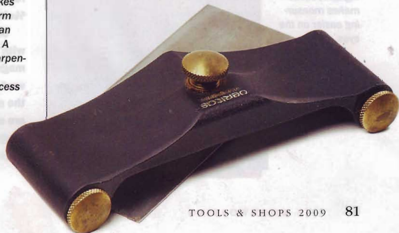
Better than just scraping by. A scraper holder maintains a constant bow in the tool so your fingers don't have to, allowing for a much more relaxed grip.
