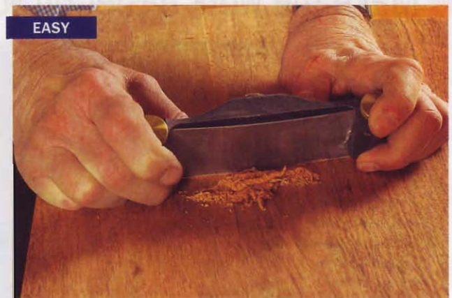
Better than just scraping by. A scraper holder maintains a constant bow in the tool so your fingers don't have to, allowing for a much more relaxed grip.
