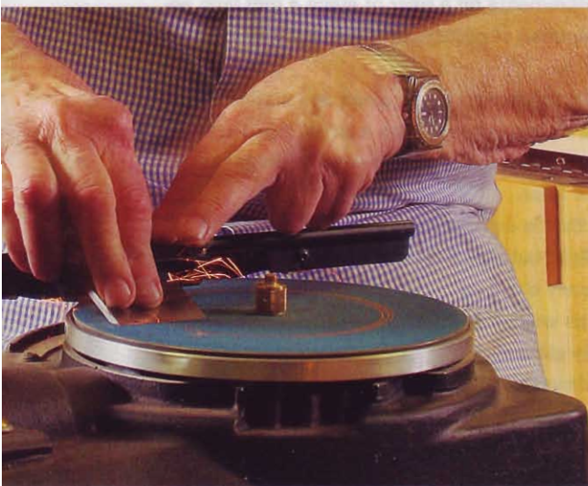
The quick way to a keen edge. Sharpening can wear out the muscles and joints in your hand with repeated strokes that call for firm pressure and an awkward grip. A horizontal sharpening machine eases the process dramatically.
