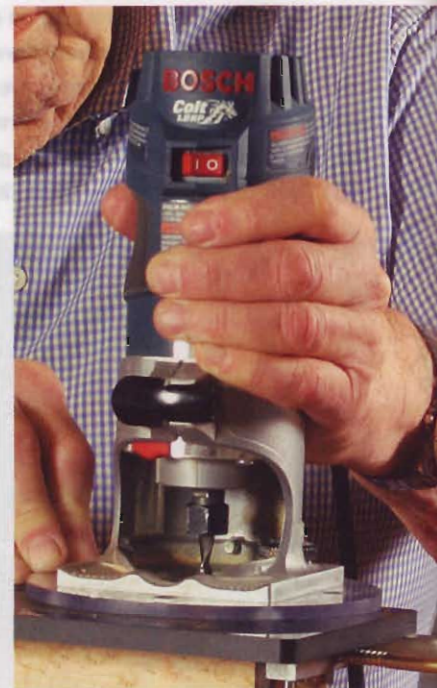
One-handed routing. For light-duty tasks such as mortising for a hinge, a lightweight router is much easier on hands and wrists.
