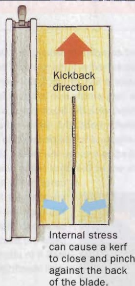
Pinch protection. A splitter or riving knife fills the kerf, so if the wood starts to close, it pinches the splitter or knife, not the blade, preventing kickback.
