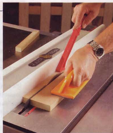
Pinch protection. A splitter or riving knife fills the kerf, so if the wood starts to close, it pinches the splitter or knife, not the blade, preventing kickback.
