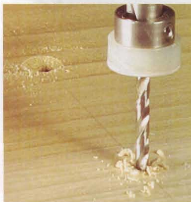
No more burn marks. The depth stop stops spinning when it contacts the workpiece, so it won't leave a burn mark in the wood.
