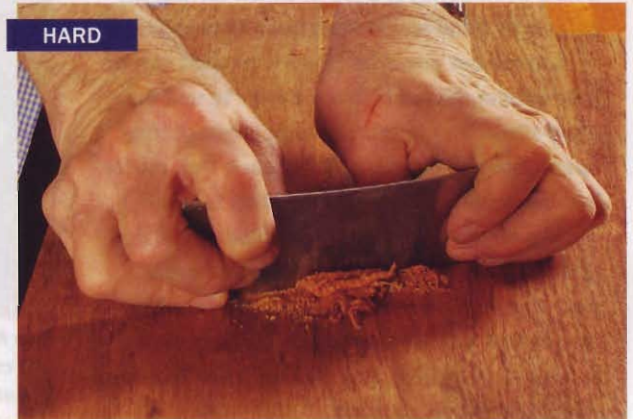
Two thumbs down. Scraping takes a toll. The process puts pressure on thumbs and fingers to flex the scraper for a decent cut.
