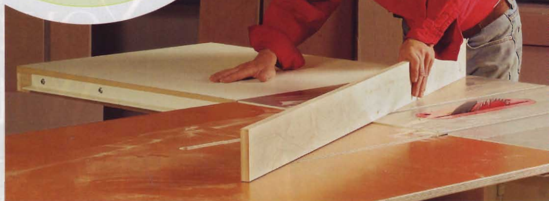
Check for a consistent gap. The outfeed table should be a hair below the saw table. Hold a straightedge firmly down on the tablesaw to check.
