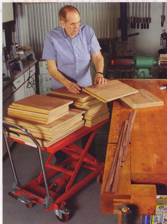
A little pick-me-up. A scissor-lift cart lifts heavy materials to bench height, and makes a multilevel work surface.
