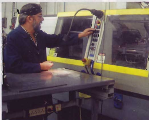
Molded under pressure. Metal-injection molding (MIM) is used to form the powder/binder/wax mixture into more complex shapes. The equipment is similar to that used for injection molding of plastics.
