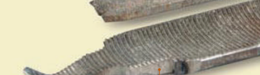
Old files reground as custom scrapers
