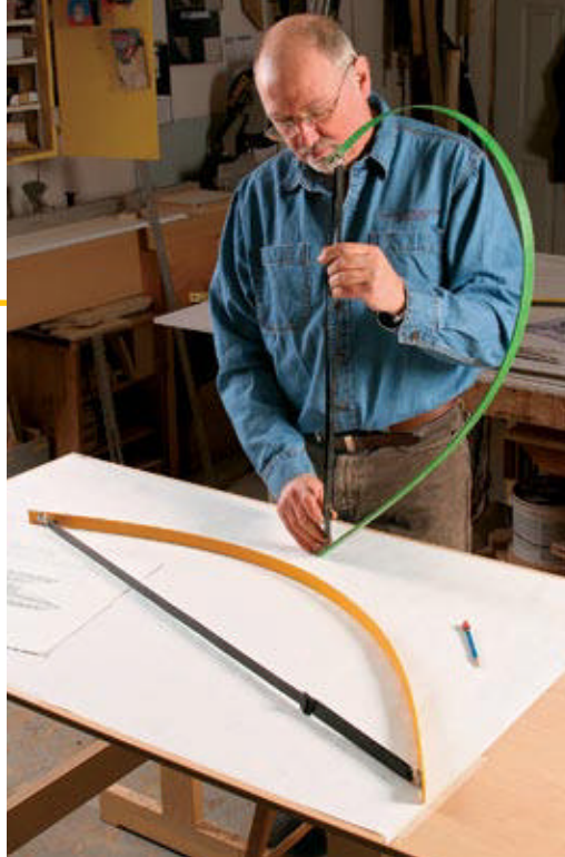
Large. Drawing bows, both symmetrical (yellow) and asymmetrical (green), are bent into shape by tensioning and locking the strap.
