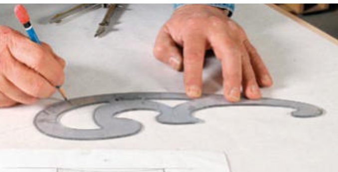
Small. Use french curves to render small details such as door handles or knobs.
