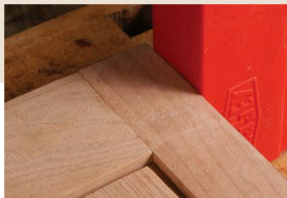
Remove the roll. Insert the tenon partway into the mortise, until the glue forms a "roll" on the tenon cheek (left.) Remove this excess glue with a clean brush (right). Keep a paper towel close at hand to clean the brush.
