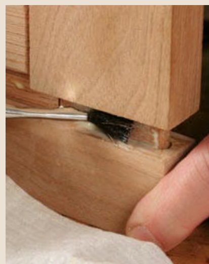
Remove the roll. Insert the tenon partway into the mortise, until the glue forms a "roll" on the tenon cheek (left.) Remove this excess glue with a clean brush (right). Keep a paper towel close at hand to clean the brush.
