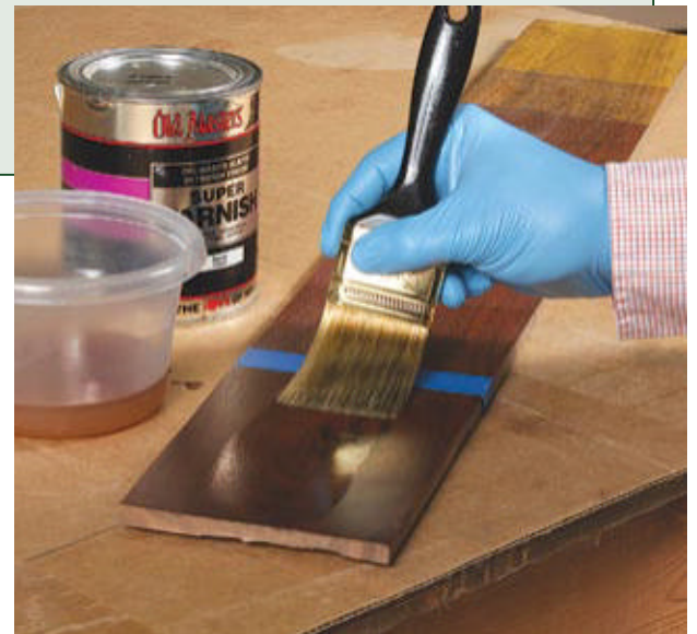
From prep to finish. Start by scraping, planing, or sanding the sample board as you will the actual workpiece (left). Then mark the lines separating each step in the coloring process (center). Then apply the finish, coat by coat, until the desired color and gloss are achieved (right). A piece of blue tape offers a way to isolate a section.
