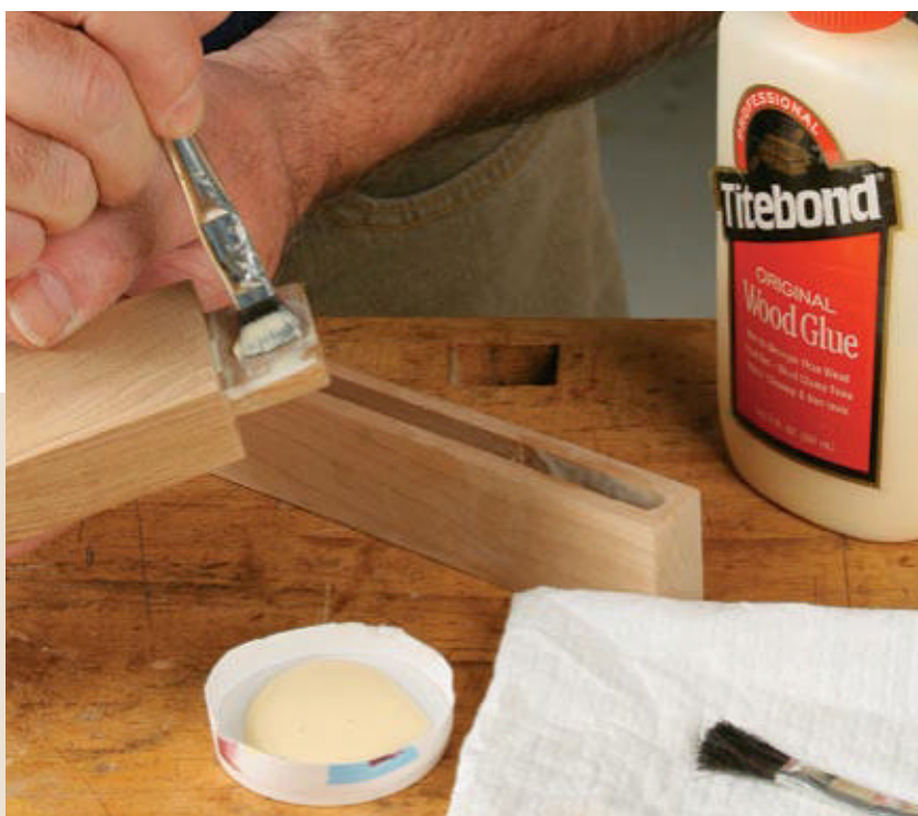
Apply the glue. Use a brush and apply it on face grain only—the mortise walls and the cheeks of the tenon.
