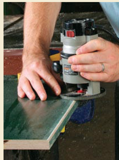
Sharp edges. Break all edges with sandpaper or a roundover bit (shown).
