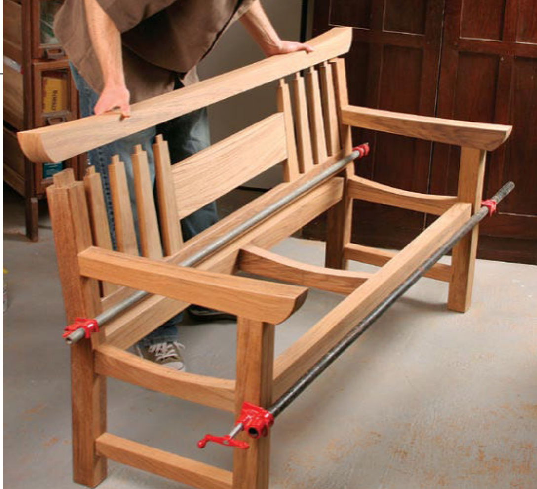
Glue the center rail to the center back splats. Jensen uses the cutoff pieces from the tapering process to create a square clamping surface (above). The tapered back splats, center rail, and crest rail complete the glue-up (right).
