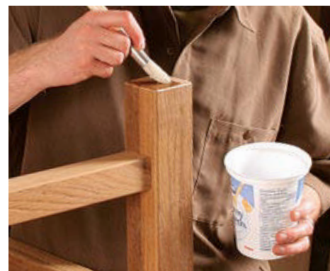
Seal the legs. Seal the bottoms of the legs by coating them with the same epoxy used in the glue-up.
