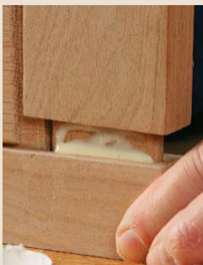
Remove the roll. Insert the tenon partway into the mortise, until the glue forms a "roll" on the tenon cheek (left.) Remove this excess glue with a clean brush (right). Keep a paper towel close at hand to clean the brush.
