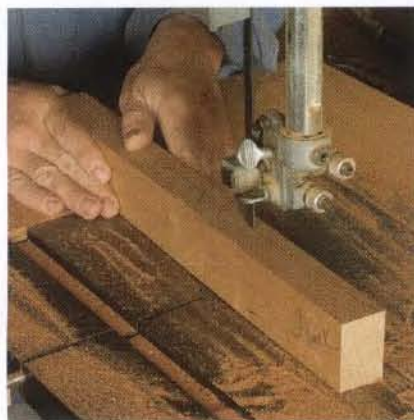
Bandsaw curves. Begin with the curve for the top of the armrests (above), then bandsaw the curves for the sides (right).
