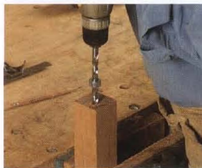
Drill for dowels. Use \frac{3}{8} -in.-dia. dowels to connect the legs to the armrests. Drill the legs first, then use dowel centers (left) to locate the holes in the armrests. Position the armrest and press down (right). Now you can drill the mating hole in the armrest.
