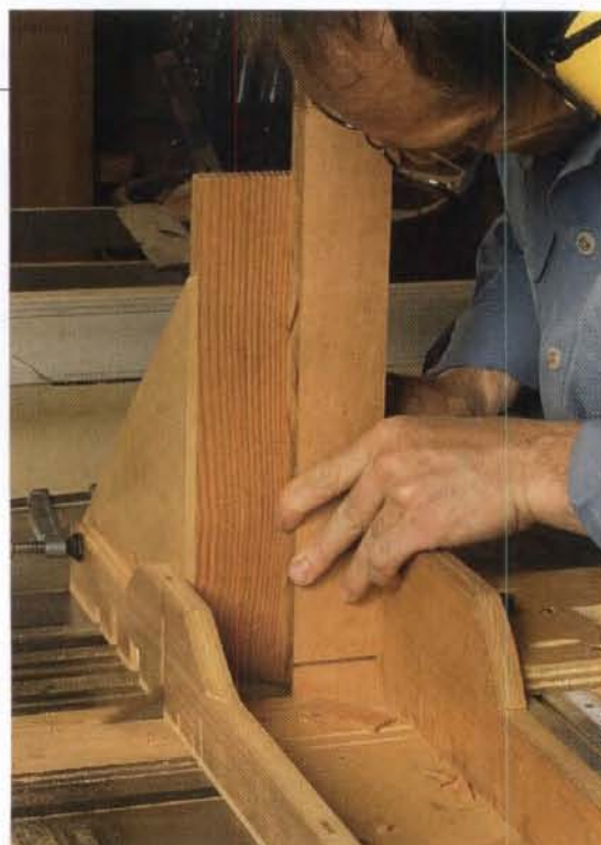
Cut tenon shoulders first. Edmundson uses a narrow, shopmade sled to cut the tenon shoulders, with a stop block clamped to it.
