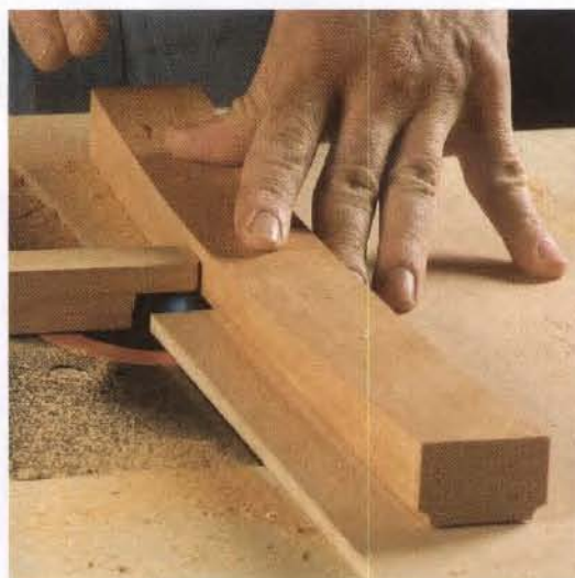
Route a cove on the underside. The cove gives the thick armrest a lighter look. Edmundson uses a narrow shopmade guide that clamps to the router table and sits above the blade. It follows both the convex and concave sides of the armrests. Reset the stop for the end-grain cuts.
