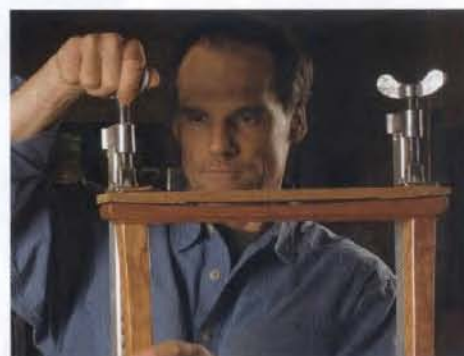
Clamp armrests last. The offcut from the curved top acts as a clamp pad. Use the edge of the bench to hold one end of the clamp, and tighten it directly over the leg.
