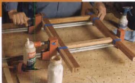
Glue up the end frames. Curved offcuts again make ideal clamping pads. Because Edmundson oils the components before glue-up, he puts leather scraps between the leg and offcut to protect the finish.
