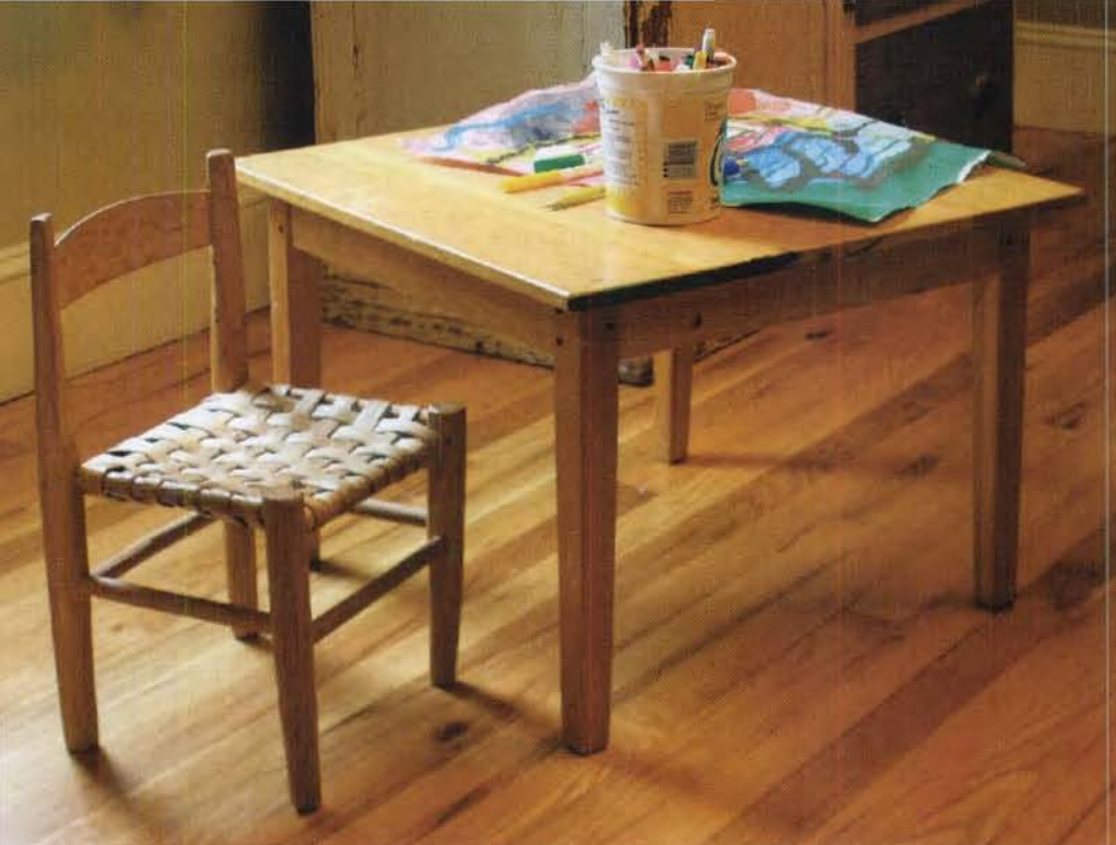
An old-fashioned play station. Built for a toddler, this set by Pekovich pairs a lightweight but sturdy post-and-rung chair with a bombproof table that features pinned mortise-and-tenon joinery.
