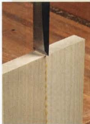
GLUE FAILURE A poor joint fails along the glueline.
