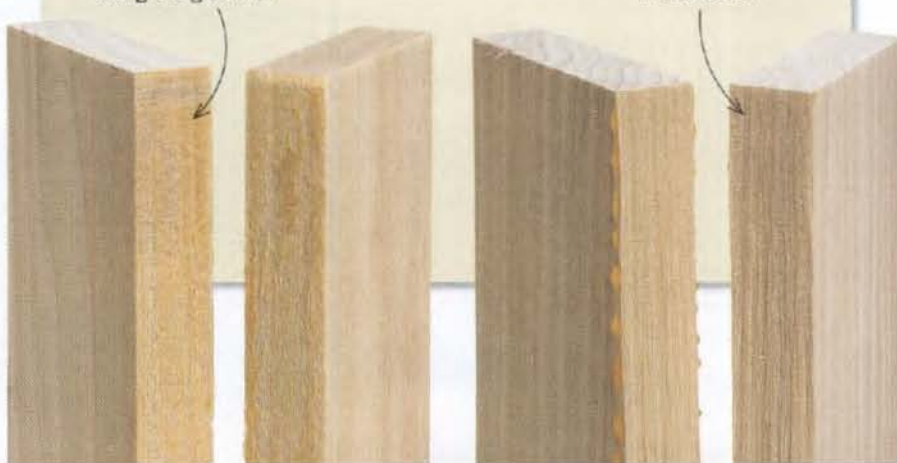
GLUE FAILURE A poor joint fails along the glueline.
