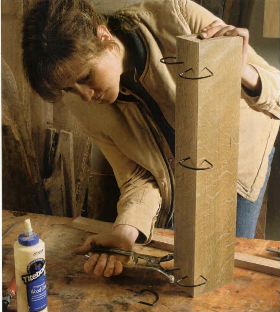
Start clamping at the front of the column. Because the pieces that form the column are now cut to length, make sure to get the ends level with each other.
