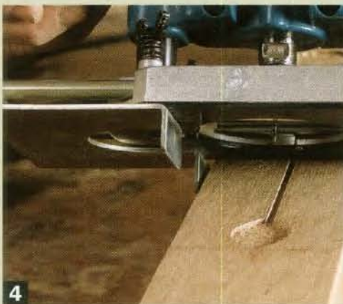
4 Rout for the stem. After routing the groove, rip stock to fit tightly into it.
