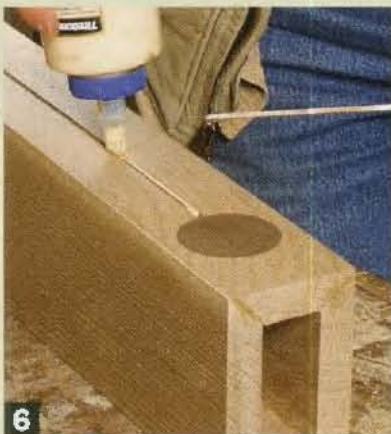
6 Insert the stem and finish up. Glue and clamp the stem in place (above). Once the glue is dry, scrape and sand the inlay flush (right).
