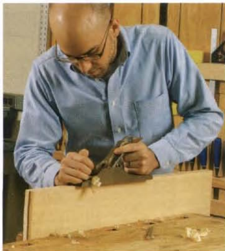
Plane both mating edges at once. This will help compensate for any misalignment in the planing angle.
