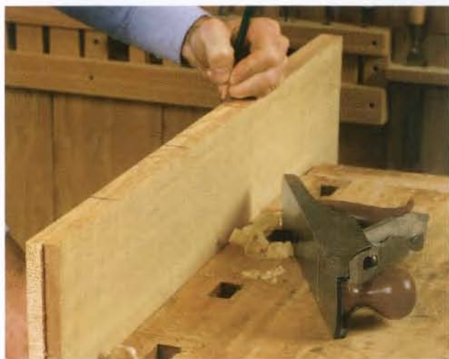
Lay out a visual guide. Separate the boards into five equal sections. Plane the middle section, the middle three, and then the entire edge.
