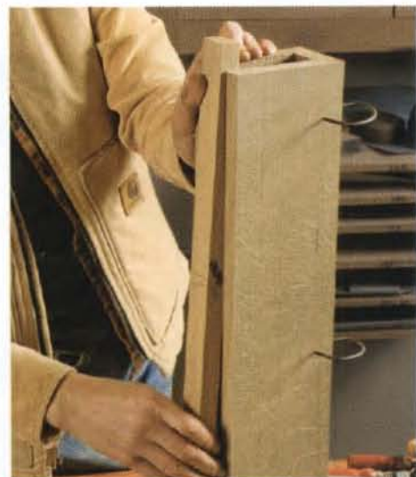
Insert the filler piece in the back. Once the back is in place, use bar clamps to apply pressure.
