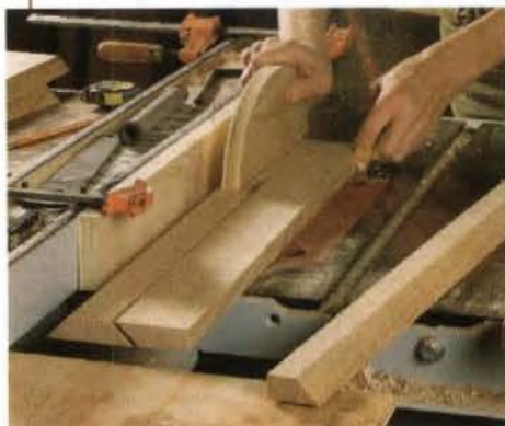
Attach an auxiliary fence. Using a supplemental fence on a right-tilt saw prevents the thin, already mitered edge from creeping under the sliding rip fence.
