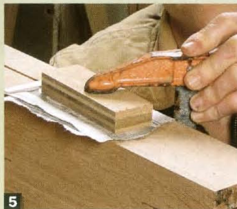
5 Glue in the flower and leaf. Use a caul to apply even pressure. Newspaper prevents the caul from sticking to the inlay.
