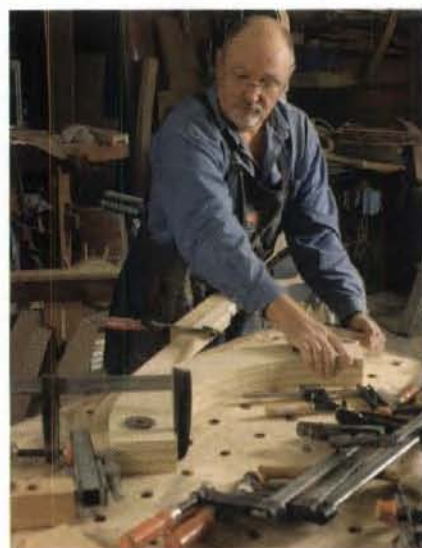
Bend, straighten, and bend again. Place the blank in the compression strap, tighten the end clamp, and then bend it around the form (left). Remove the blank from the strap, place it loosely in a vise, and lever it until it is almost straight (center). Flip the blank so that the face that was against the strap is now against the form, and bend it again. In this way the lignin that bonds the wood fibers is loosened across the width of the blank (right).
