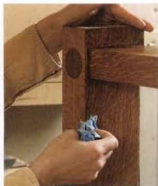
Wipe off excess gel stain. If the stain sets too long, a rag with paint thinner will return the stain to a workable state.
