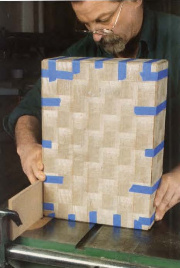
Grooves for binding. With top and bottom sections taped together temporarily, Janofsky cuts a shallow rabbet into each corner to hold the binding—thin strips of white oak.
