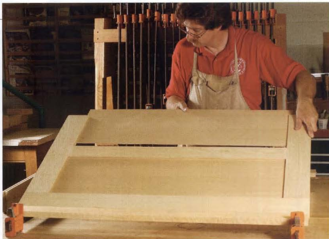
Assemble the back. The \frac{1}{2} -in.-thick plywood is rabbeted on the back side, ensuring a good fit in the grooves. Check carefully once the clamps are on to make sure the assembly is flat, tapping the components into place with a deadblow hammer, if needed, as you tighten the clamps.
