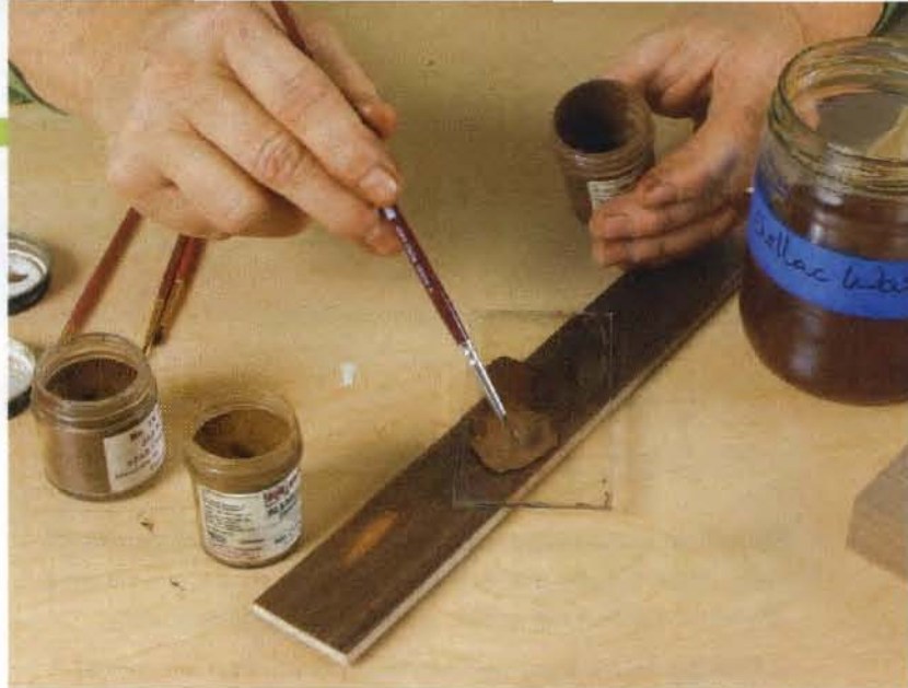
Practice patch. Make a similar burn-through on a scrap of the same plywood. Mix touch-up powders with thinned shellac to match the color of the face veneer and hide the sanded-through spot.
