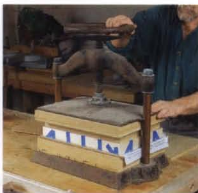
Begin veneering at the top. Liberal amounts of blue tape hold a veneer sheet securely in place on the top of the carcase.
