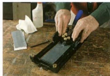
The good and the bad. The sled of the Pinnacle honing guide glides smoothly and keeps the blade square to the stone (above). But you can't flatten the back of a blade while it's in the sled (below). You have to remove the blade from the sled to perform that task.
