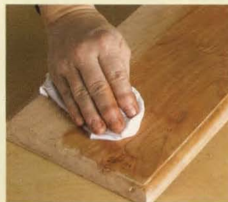
Check your work. Wipe on mineral spirits before applying the finish. This will reveal any lingering scratches or patches of tearout.
