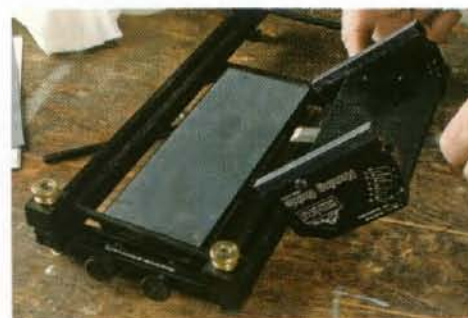
The good and the bad. The sled of the Pinnacle honing guide glides smoothly and keeps the blade square to the stone (above). But you can't flatten the back of a blade while it's in the sled (below). You have to remove the blade from the sled to perform that task.
