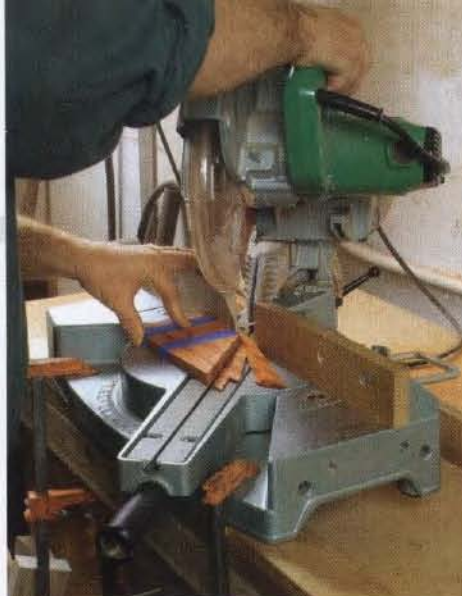
Leaves begin as simple shapes. Use a miter saw to cut blanks at a 45° angle from the end of a stack of veneers. Cut plenty of blanks, because you need 14 for each leaf.
