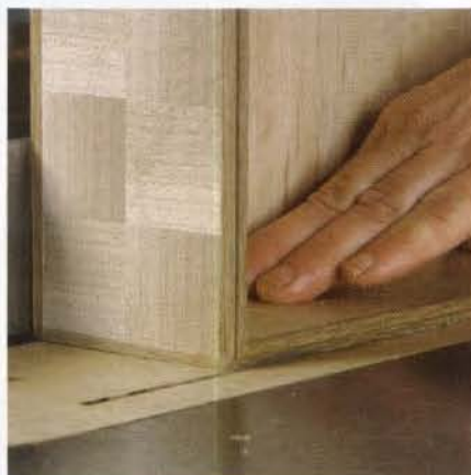
A rabbet meets its mate. Binding, mitered and glued to the lip of the bottom section, will mate with similarly rabbeted binding on the top section. Make a series of light cuts to sneak up on a tight fit.
