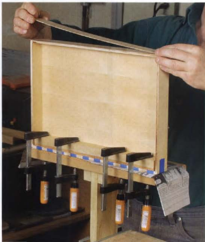
A box-sized caul. The top is clamped in an antique book press while the glue dries. A caul, made of layers of medium-density fiberboard (MDF) with cork padding on one face, provides even pressure. If you don't happen to own an antique book press, a pair of cauls and lots of clamps will do nicely.
