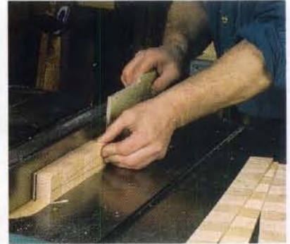
Block becomes veneer strips. Maple blocks are stacked so that the edge grain is alternately horizontal and vertical. Then they're glued and clamped in a simple fixture (left). Once completely dry, the glued-up block is ripped into strips ¼ in. thick (right).
