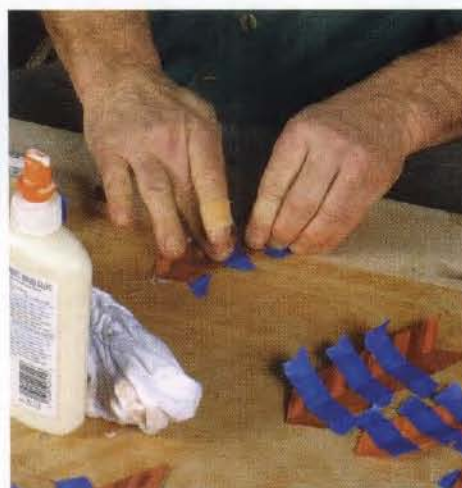
Glue up pairs. Edge-glue pairs of blanks to form a chevron or arrow-feather shape. The grain patterns will mimic veins in real leaves. Tape holds the pieces together.
