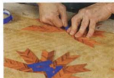
Glue groups of chevrons. Edge-glue seven chevrons to complete the leaf blank. Work carefully to be sure that all the chevron points converge at a single point.
