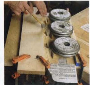
An ingenious clamp. Scrap blocks and weights keep veneer sheets from buckling (above). Wedges tapped in place between the veneer and fence provide clamping pressure.
