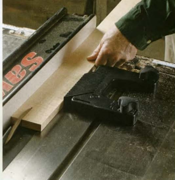
Safety where you need it. A featherboard helps keep the board snug to the fence at the start of the cut, where you have the least amount of control.
