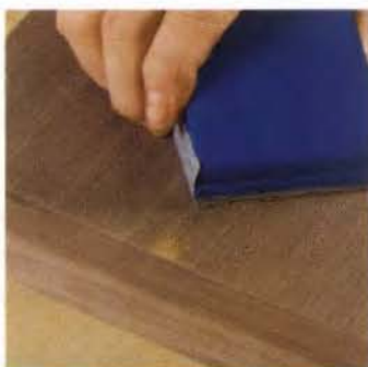
Overdone. It doesn't take much to sand through the face veneer on hardwood plywood.
