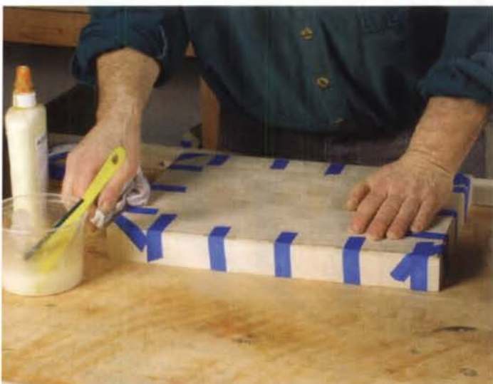
Begin veneering at the top. Liberal amounts of blue tape hold a veneer sheet securely in place on the top of the carcase.
